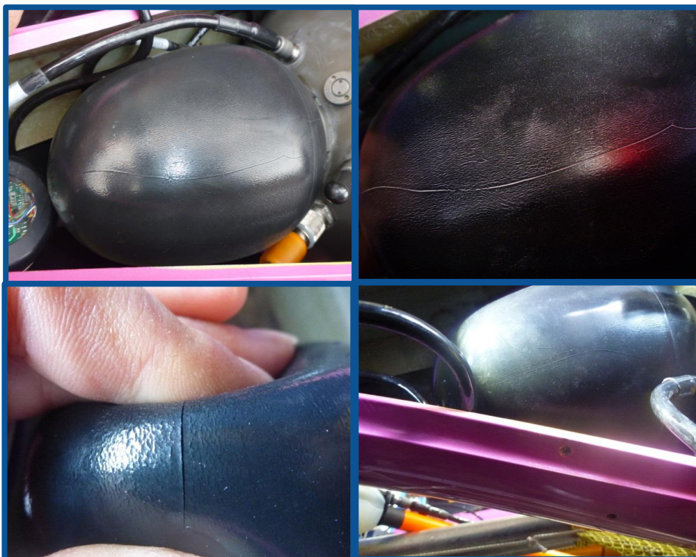
Figure 26: Clockwise from top-left: 1) Crack along the top of the bladder; 2) closer view of same crack with talcum powder to make it more visible; 3) marks underneath the bladder; 4) close-up of crack.
