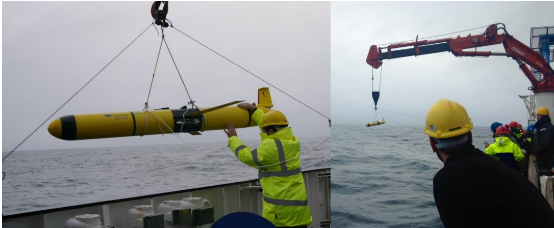
Figure 28: Deployment of the extended bay Slocum Glider.
