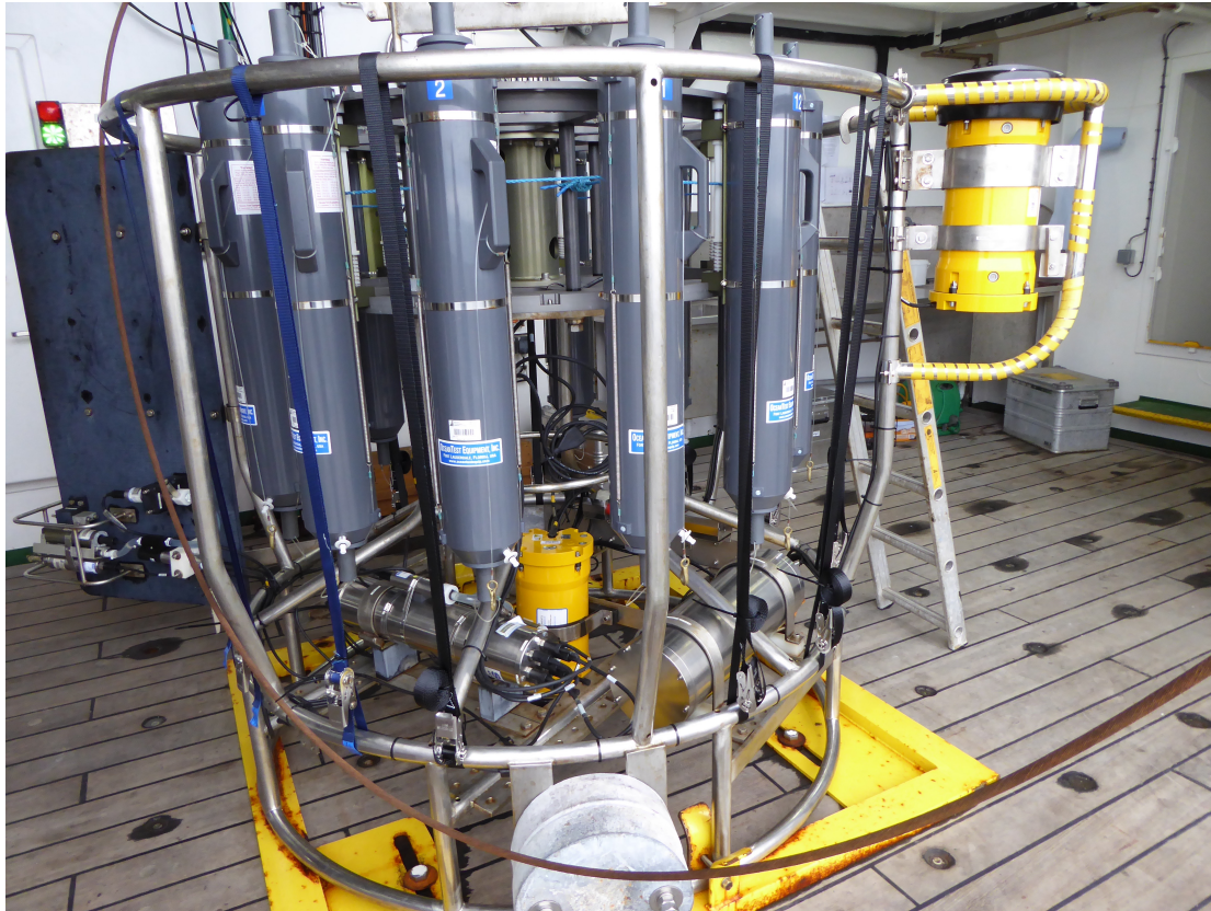
Fig. 4.1 DY054 Sensors arrangements. Primary sensors on the fin, secondary in-frame. 12 niskin bottles in place, and straps present for attaching microcats for calibration dips.
