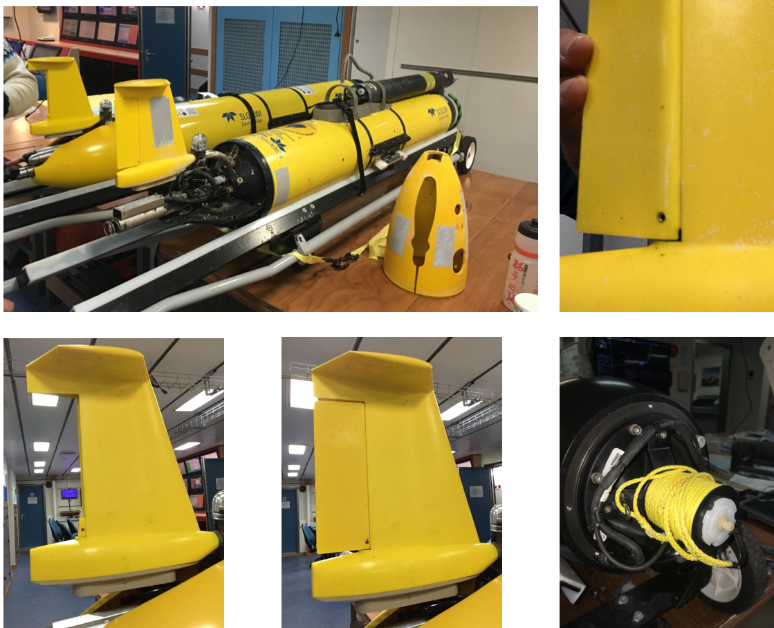
Figure 2.10: (top left) Churchill and Boomer on the bench before refitting. (top right) detail on the small crease found on newer models of G2 digifins that makes them interchangeable. (bottom left and centre) before and after refitting rudder on Churchill. (bottom right) nose recovering system reinstalled.
