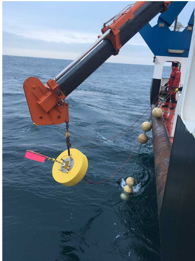
Figure 2.56: End of the third deployment in very calm seas. The photography shows the release of the immersed floats and the surface buoy.
