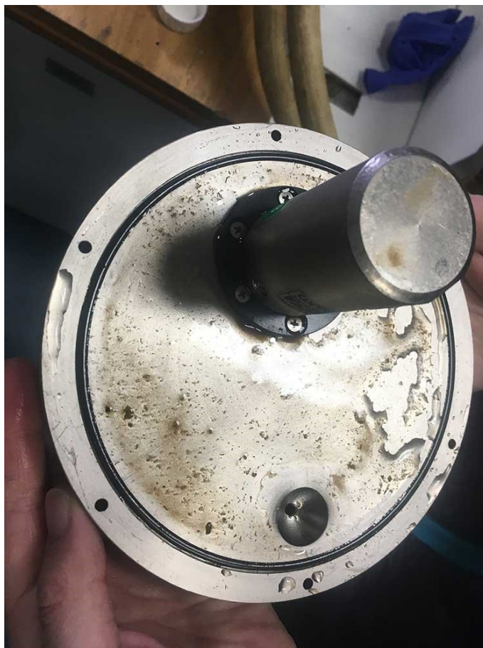
Figure 2.46: Particles remaining at the surface of the bottom plate after drainage of the incubation chamber (100 m trap, deployment 1)
