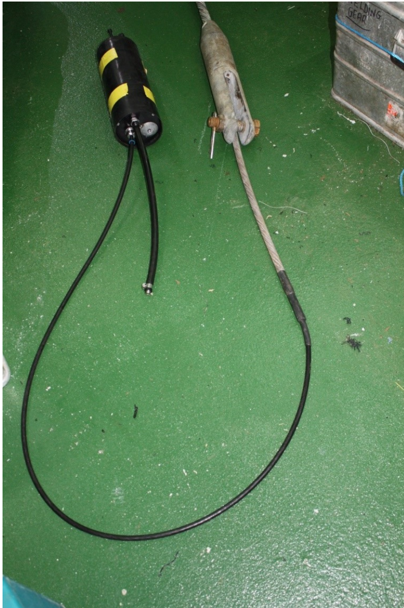
Figure 2.63: Evergrip termination and core cable to BAS electronics housing
