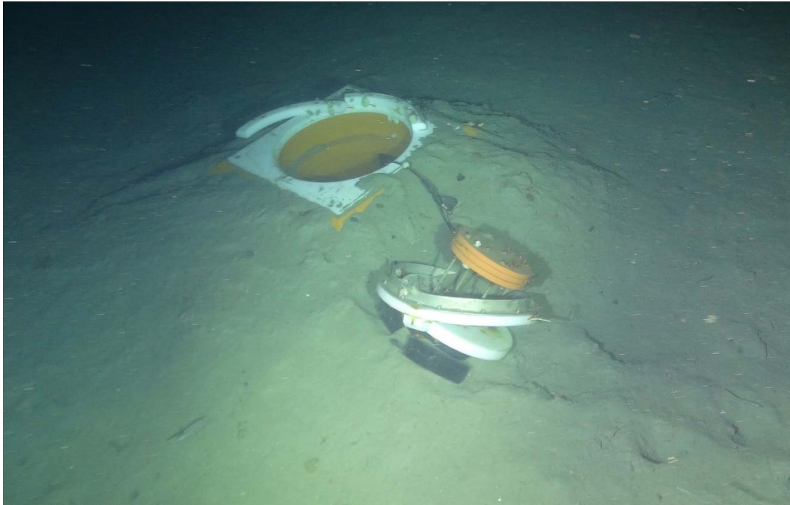
Fig. 6.82 ADCP lander deployed on AR30 cruise in 2018. Imaged by HyBIS in September 2019 after it failed to surface and was found to have been damaged and partially buried by trawl activity.
