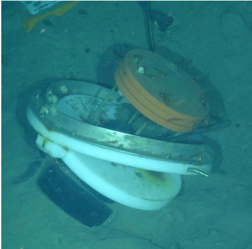
Fig. 7.33 - Photo showing close up of detached ADCP.
