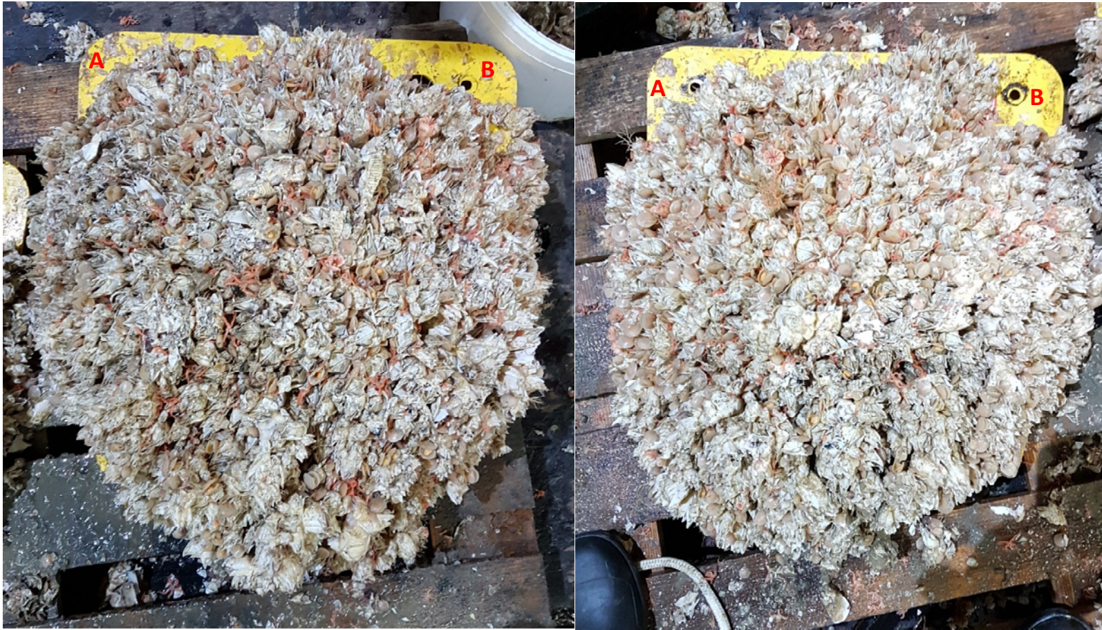
Fig. 6.70 Biofouling on the two halves of the Darwin Mounds East mooring buoy - the width of the buoy (from point A to point B) is 494 mm.
