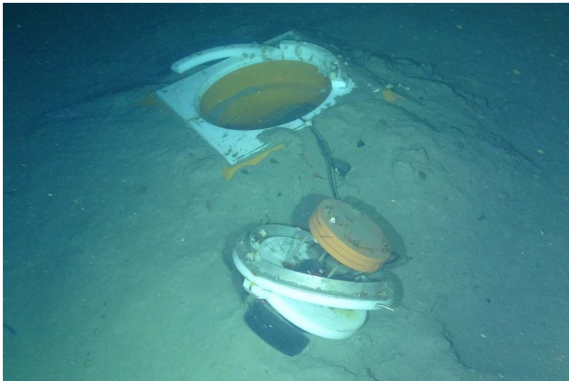
Fig. 7.32 - Photo showing silt covered lander with detached ADCP.
