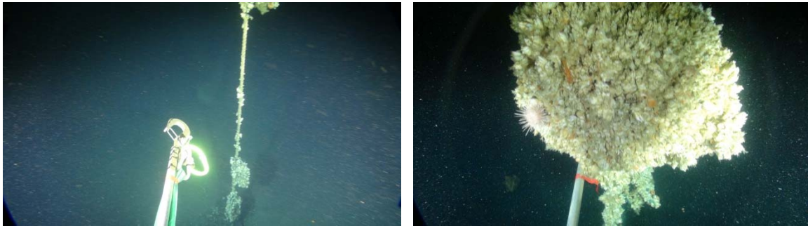
Fig. 6.65 a & b. Darwin Mounds East buoy on seabed showing the location of the two settlement panels near the base of the mooring (left) and close-up of buoy during ascent (right).
