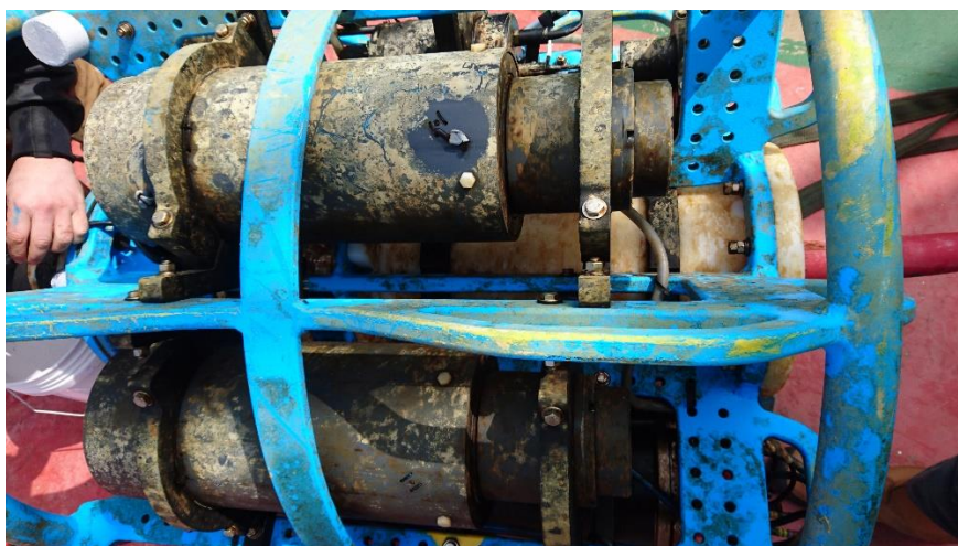
Figure 24 Lab-on-a-chip sensors within the NSIF on recovery of the buoy.
