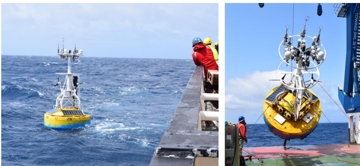
Figure 23 Buoy hooked and coming astern (left) and being hauled on board (right).
