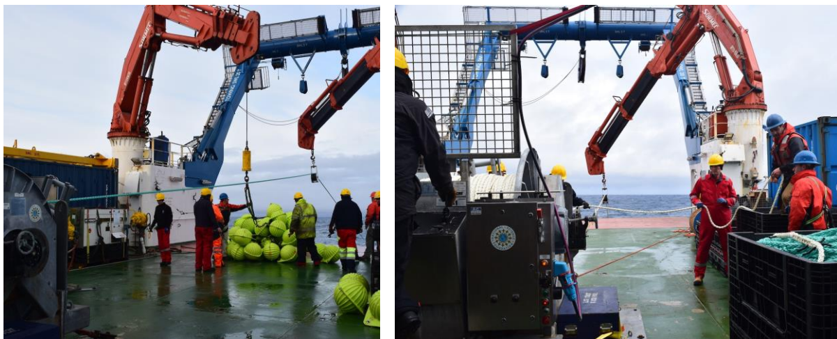
Figure 21 Glass balls on deck and Colmege line being hauled in (left), and the TSE winch being off-spoiled (right).
