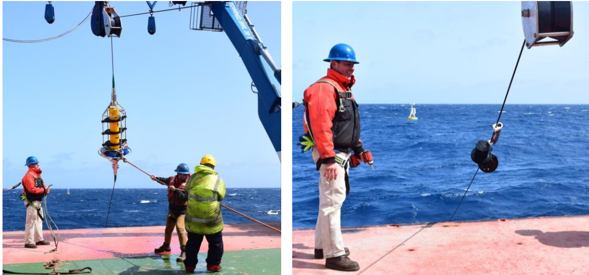
Figure 22 ADCP and instrumentation clamped onto the wire rope being hauled aboard.
