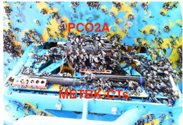
Figure 3-8 – Buoy subsurface sensor panels – starboard side (left) and port side (right)
