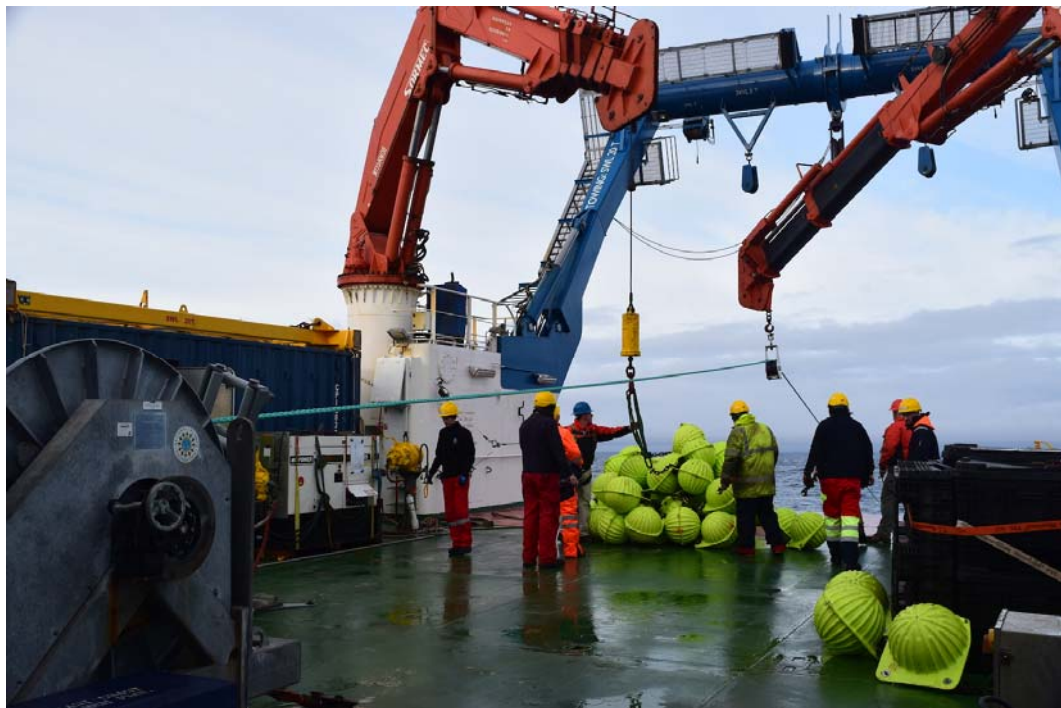
Figure 3-2 – Glass balls secured on deck and Colmega line being hauled in onto the TSE winch
