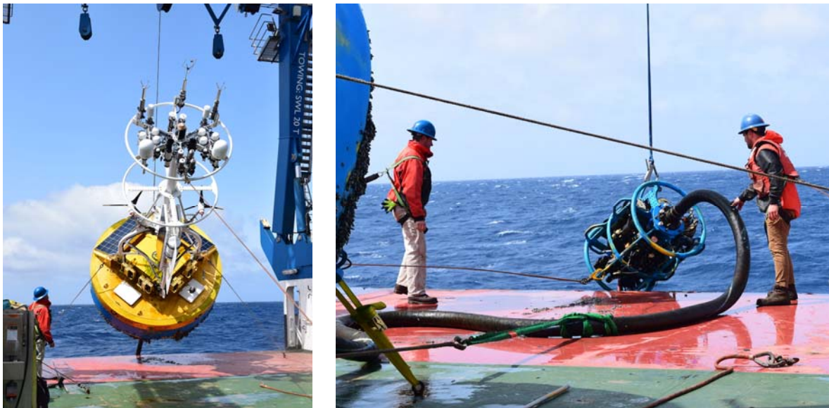
Figure 3-6 – Recovery of the GS01SUMO-00004 surface buoy and NSIF
