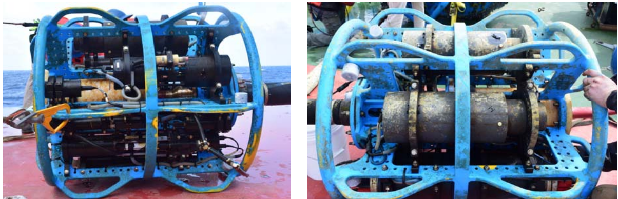
Figure 3-9 – GS01SUMO-00004 NSIF – OOI core instruments (left), CUSTARD sensors (right)
