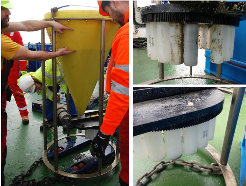
Inspection of the sediment trap from the WCM, filled with sediment on recovery to deck
