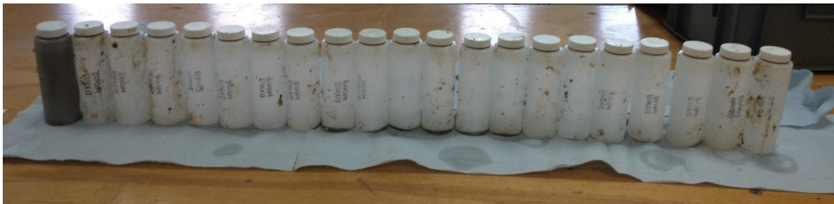
Sediment trap bottles removed from WCM and shown in sequence in the laboratory
