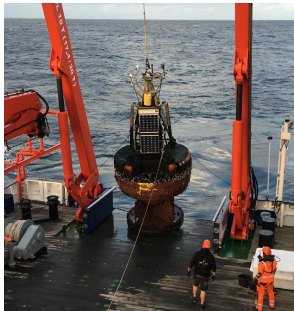
DY103 PAP1 buoy onboard FS Maria S Merian, showing the extent of biofouling
