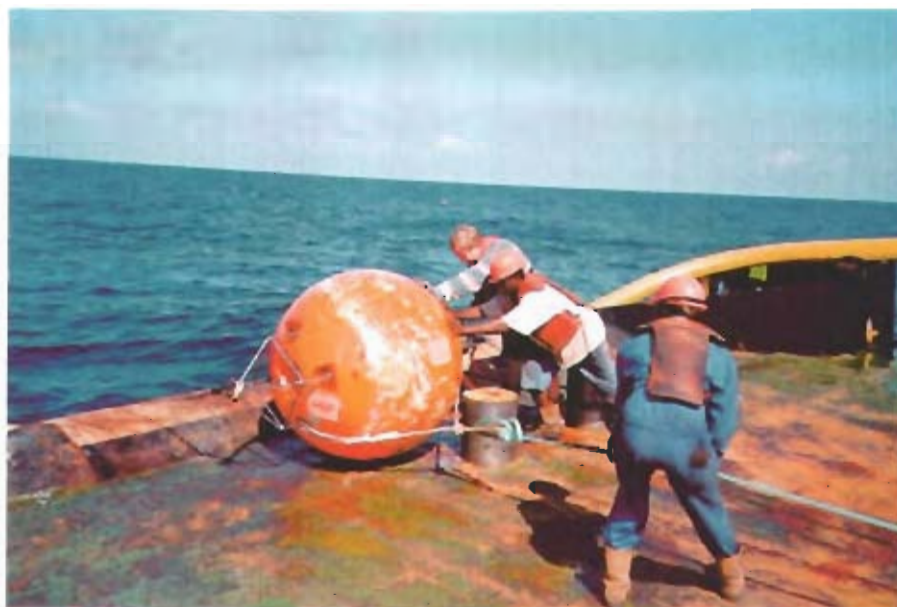
PLATE 5 Recovering the Broadband ADCP and Flotation Collar
