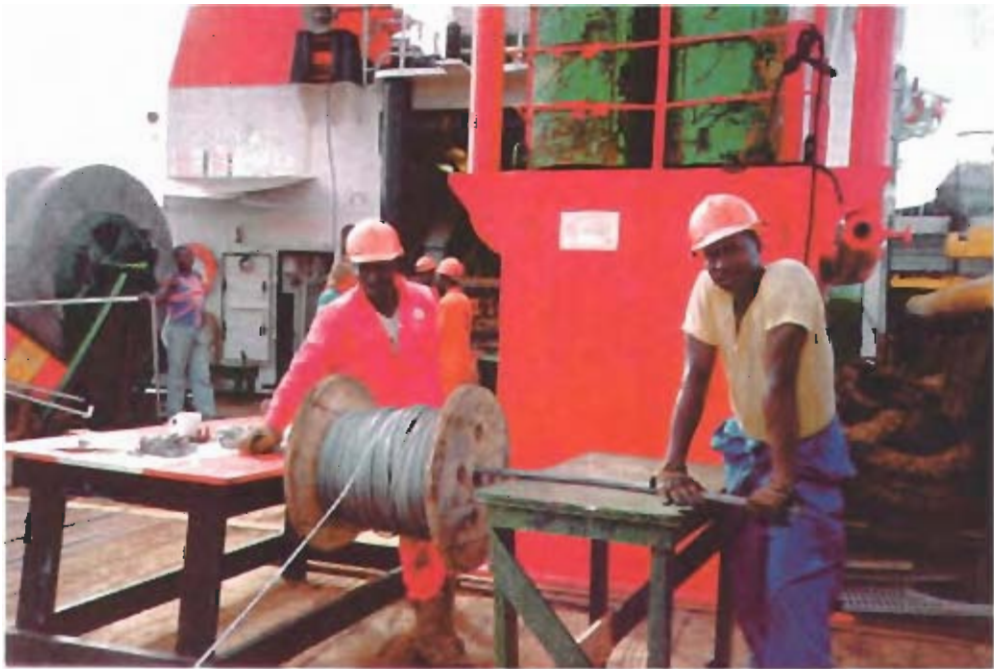
PLATE 2 Winding Wires onto the Winch
