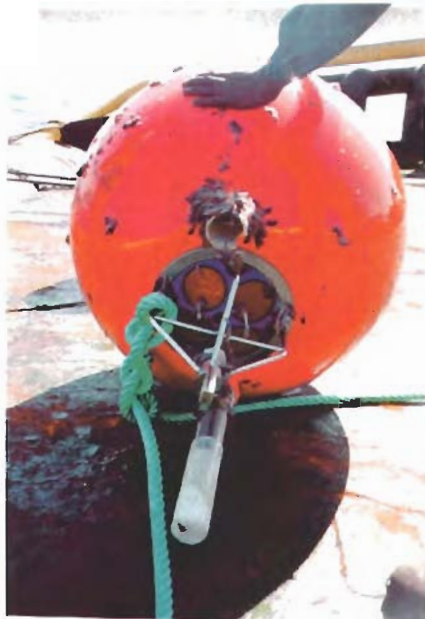
PLATE 4 Bio-fouling on the Workhorse ADCP
