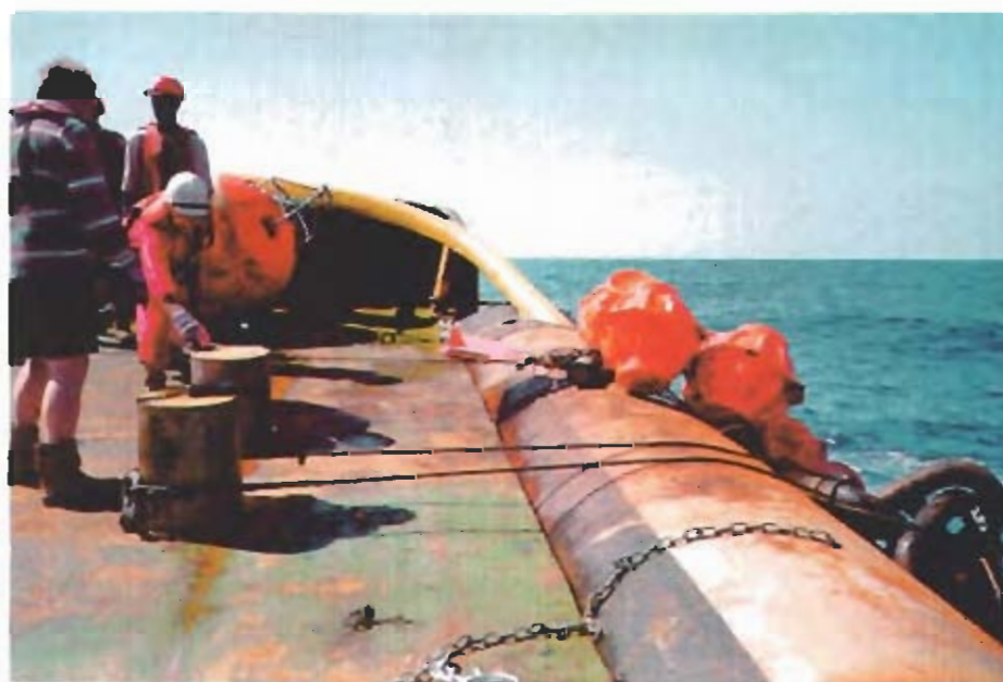
PLATE 6 Recovering an RCM and Glass Buoyancy
