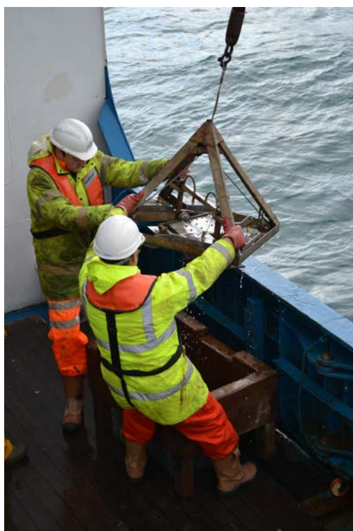
Figure 2 – Use of the 0.1 m 2 Day grab during retrieving. Photo by Robin Masefield (Cefas).
