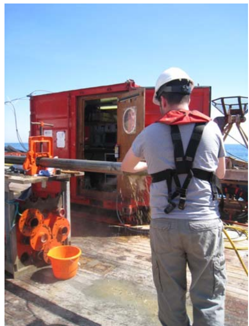
Figure 2, Removing the core liner from the core barrel
