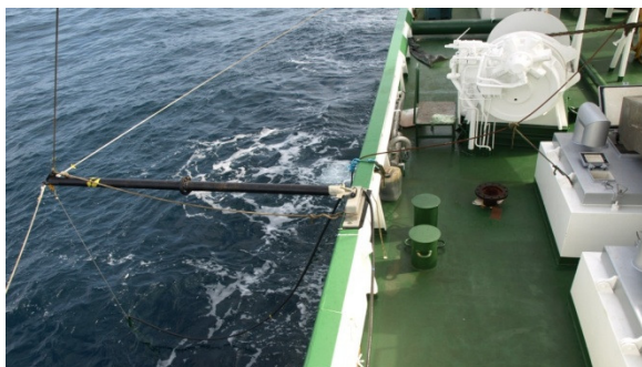
Figure 3. Towing boom c.3m long, with support stays.
