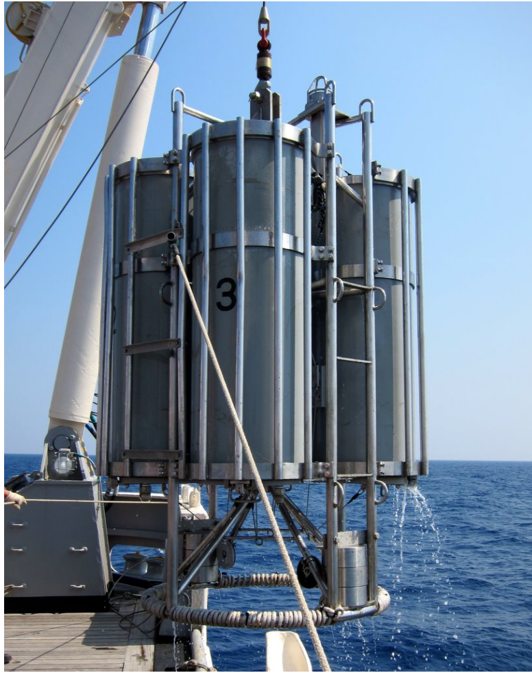
Fig. 1 Photograph of the large-volume water sampler used in the KH-09-5 cruise.
