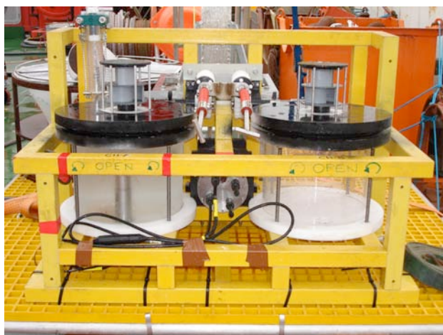
Figure 16. Left: BICS2 on deck after deployment, attached to the elevator by cable ties and jubilee clips. The titanium pressure housing is flanked either side by a respiration chamber, only the left chamber contains an optode and is in use. Right: BICS 2 at the seabed during deployment 1; it is deployed on the elevator with the chamber lids open. The right hand ROV manipulator is in view; the collection scoop being held contains a starfish ready for placement in a respiration chamber.
