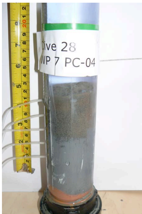
Figure 8. A push core modified for pore water extraction retrieved from Mercator MV. The core shows 4 cm of hemipelagic sediment on top of mud breccia.
