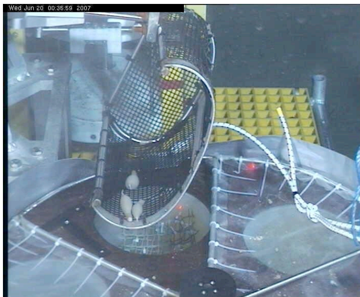
Figure 11. ISIS scoop putting M. musculus in each chamber of the experimental apparatus
