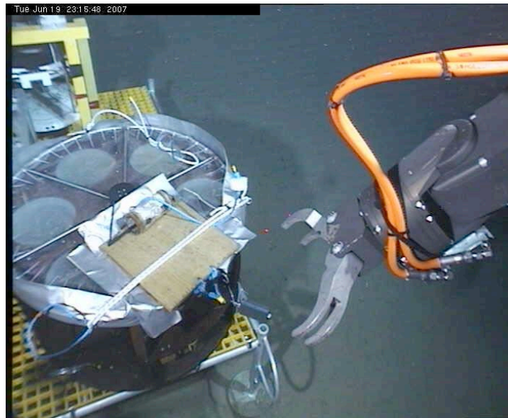
Figure 10. Holothurian experimental chambers at 3500 m in the Nazare Canyon.
