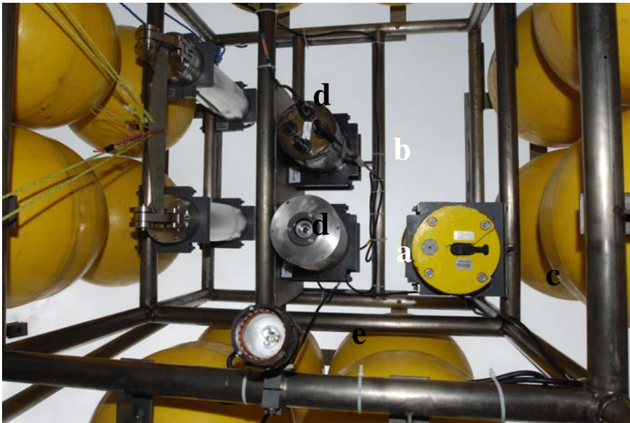
Figure 47: DOBO camera (a), controller (b), ADCP (c), acoustic releases (d) and LED light (e).
