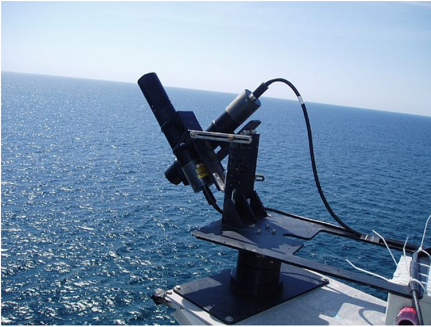
Figure 23: Configuration of the SATLANTIC HyperSAS mounted on the observation platform of RRS James Cook.
