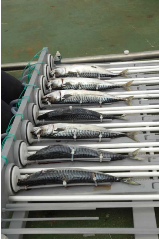
Figure 49: Mackerel bait in position before the bait release tubes were filled with seawater and cocked.
