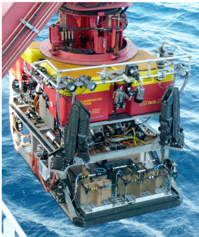
Figure 3.1. View of the forward part of the Isis vehicle, about to be launched from the port side of RRS James Cook . Note sample baskets on the sled, two manipulator arms, and array of forward-looking video and still cameras.
