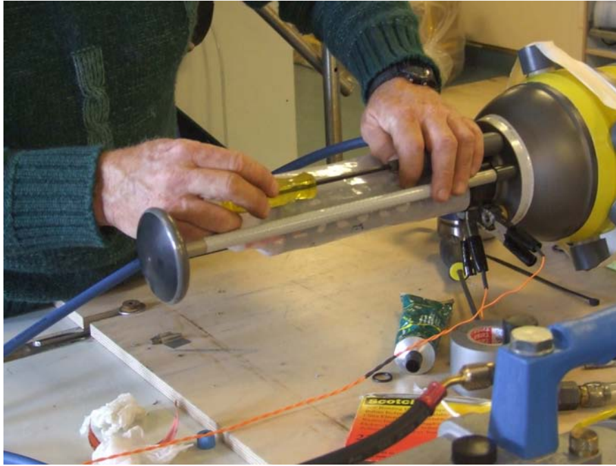
Figure 12: Phil Adam's hands using the tool he made to obtain a vacuum, in a controlled manner, in float 4051.
