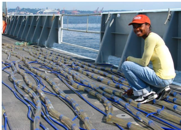
Figure 8. Streamers laid out on deck prior to deployment. Each streamer is summed into a single channel.
