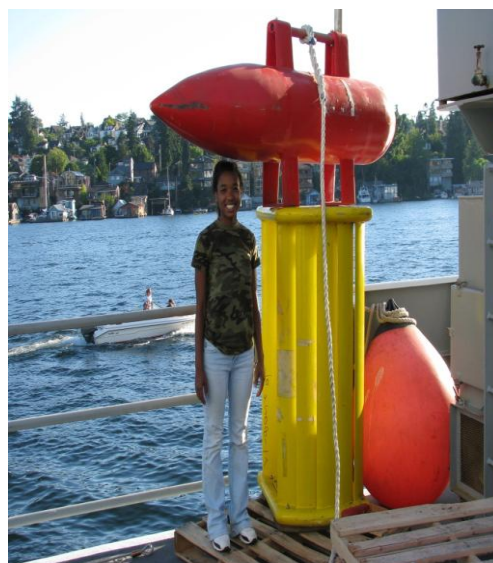
Figure 9. One of two Paravanes that connect to the cross wire and used to separate streamers. See Fig 7 for diagrammatic arrangement of the paravanes.
