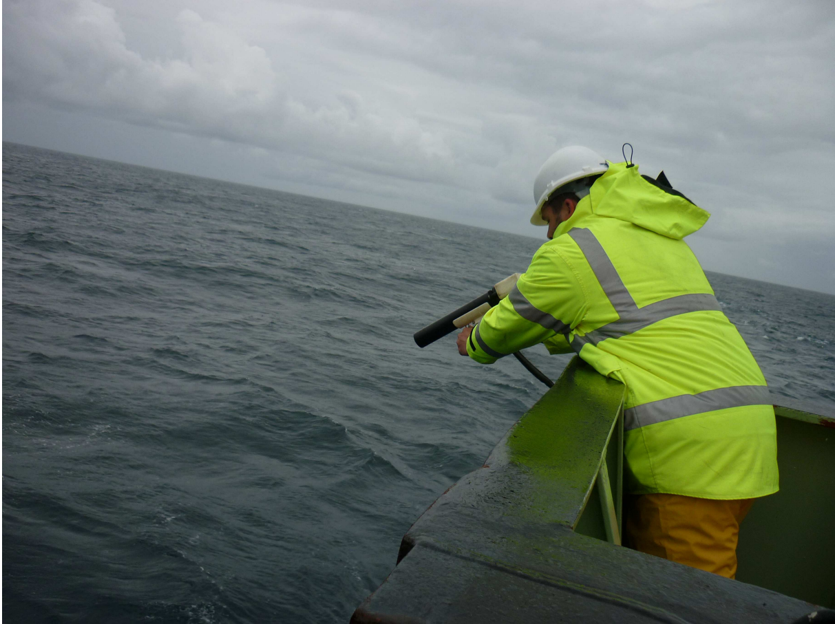
Figure 7: Launching of XBT-T5 probe from aft starboard deck.
