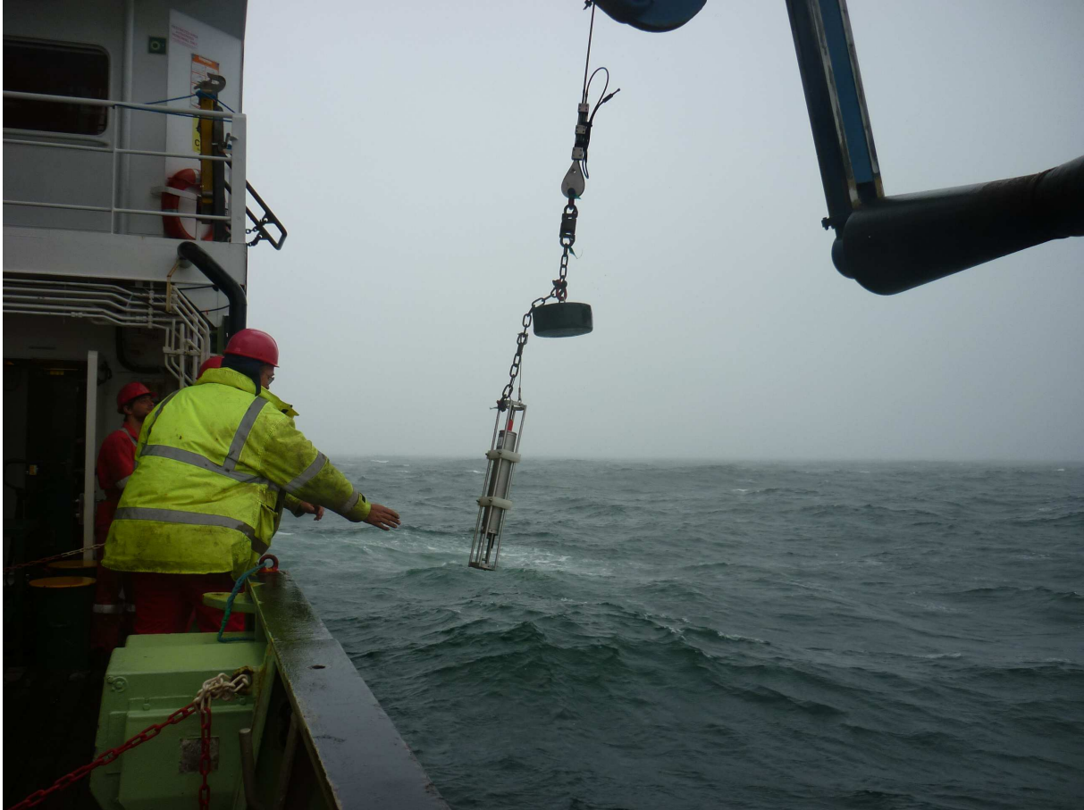
Figure 8: Launching of Sound Velocity Probe (SVP) from starboard midships.
