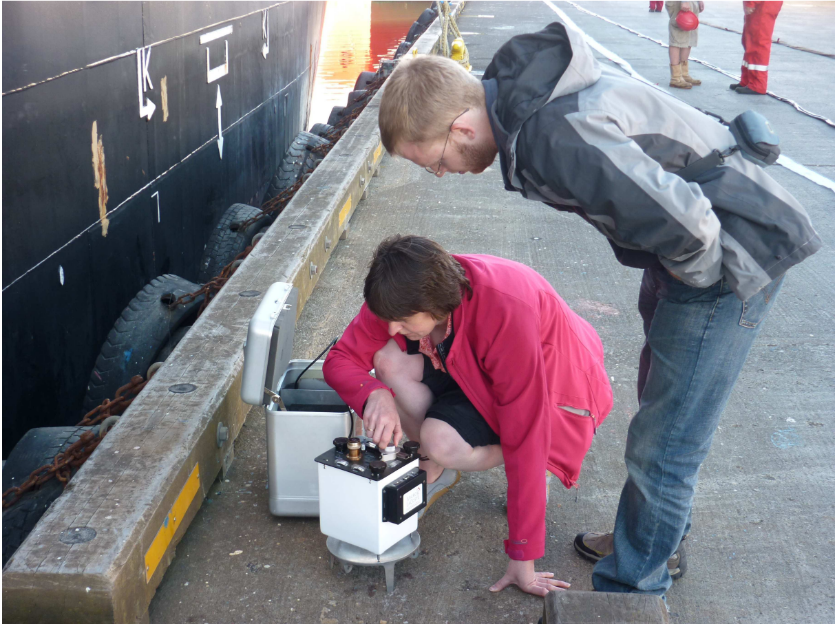
Figure 9: Calibration of gravimeter beside vessel prior to measurement of gravity field at nearby base station.
