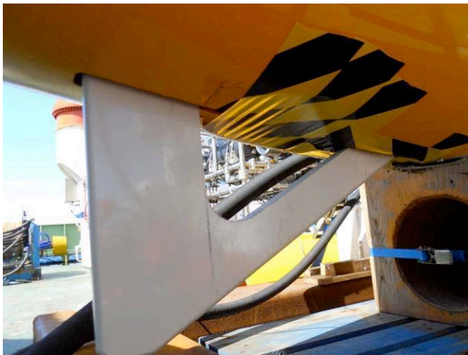
Fig. 1.11. Looking up at the tail section, 'bumble bee' tape covers the aperture cut after mission 41 for the sub bottom profiler transmitter
