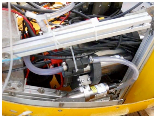
Fig. 1.3. Port CT (mounted below the panel split line) and Oxygen sensor uppermost
