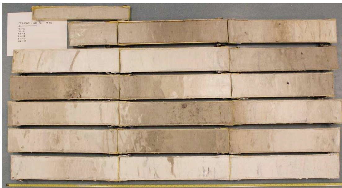
Fig. 6.2. Core photo of piston core JC060-060 showing alternating dark (cold period) and pale (warm period) hemipelagic units
