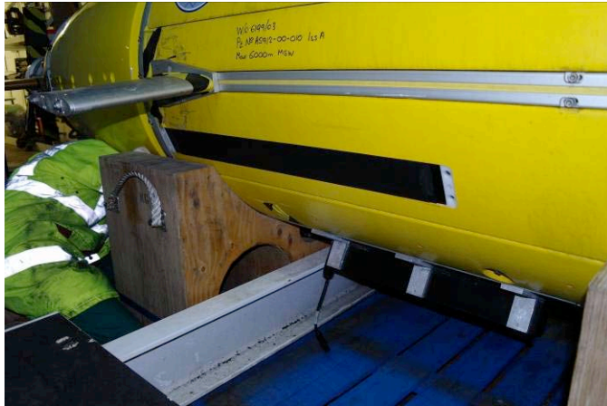
Fig. 1.12. Sub bottom profiler receivers (bottom of photo) mounted outside vehicle after mission 41
