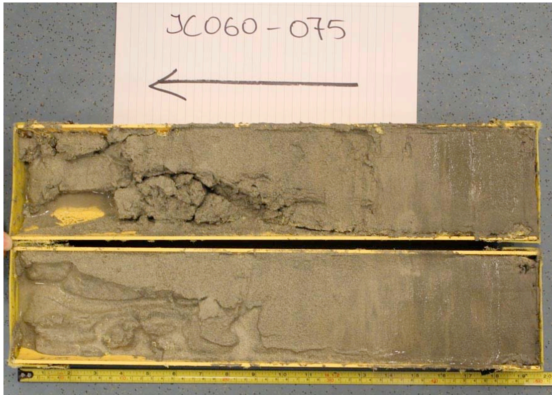
Fig. 6.4. Core photo of piston core JC060-075 showing disturbed sand overlying darker glacial mud at base.
