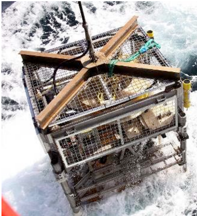
Fig. 11.2. The TMS was routinely equipped with two USBL Beacons, 12 and the new wideband super sub mini. Both beacons are shown in this image
