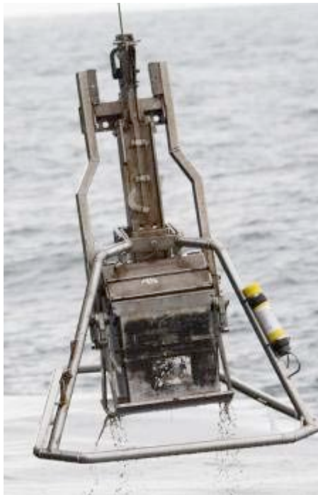
Fig. 11.1. SMBA Box corer had a super sub mini mounted on the frame which gave good returns
