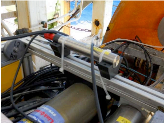
Fig. 1.4. Magnetometer mounted on top of nose frame, avoiding magnetic materials where possible. Shown here across the vehicle, moved 90 degrees in line with vehicle and to port side before cruise to reduce magnetic effect of the Argos batteries (just in shot at bottom RH corner)
