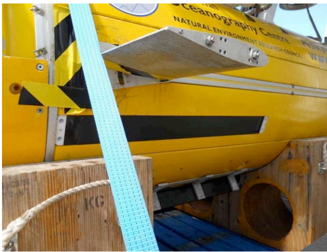
Fig. 1.10. Edgetech Side Scan inset into the centre buoyancy blocks just below the winglets
