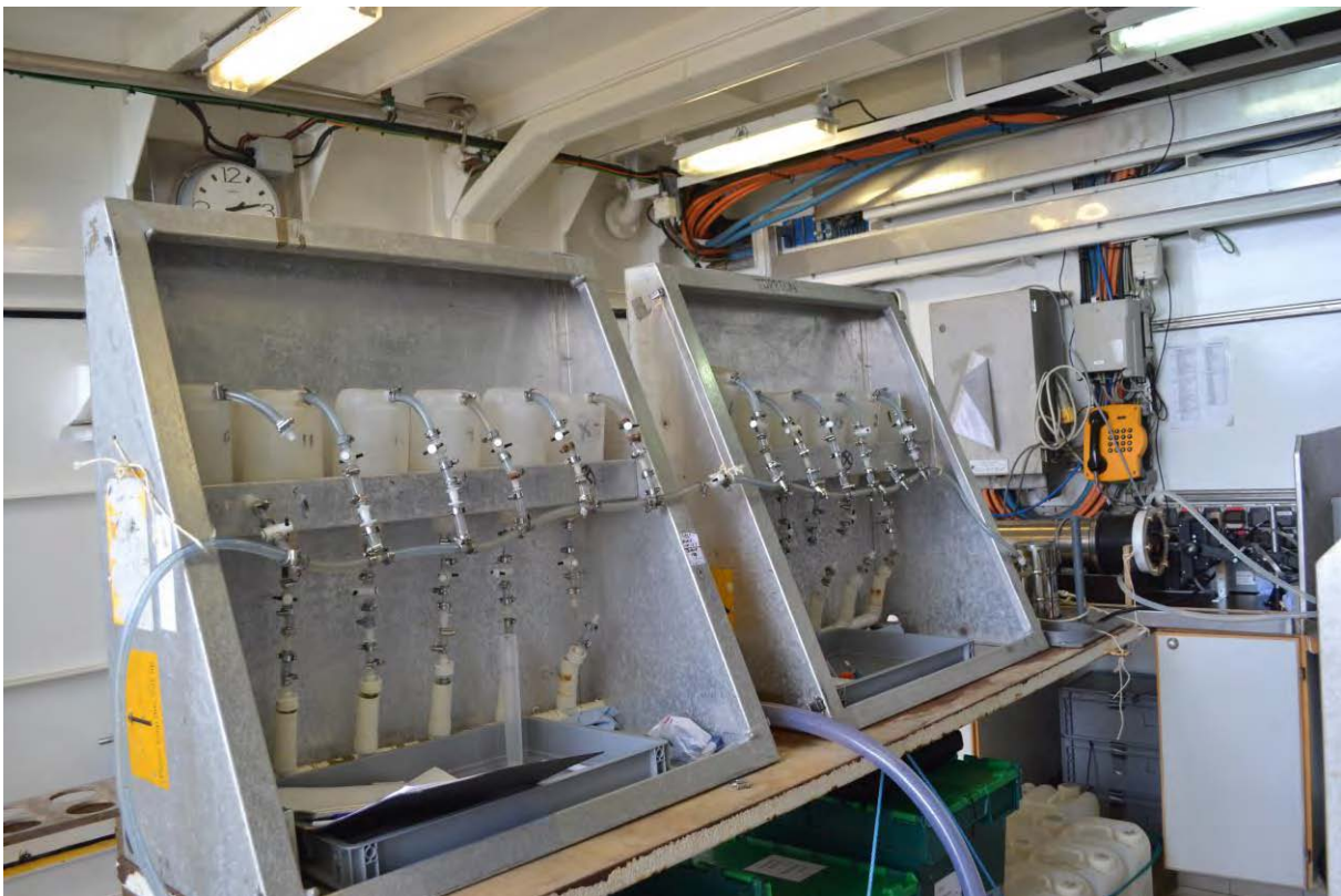
Figure 4.7.1. Shipboard water filtration system.
