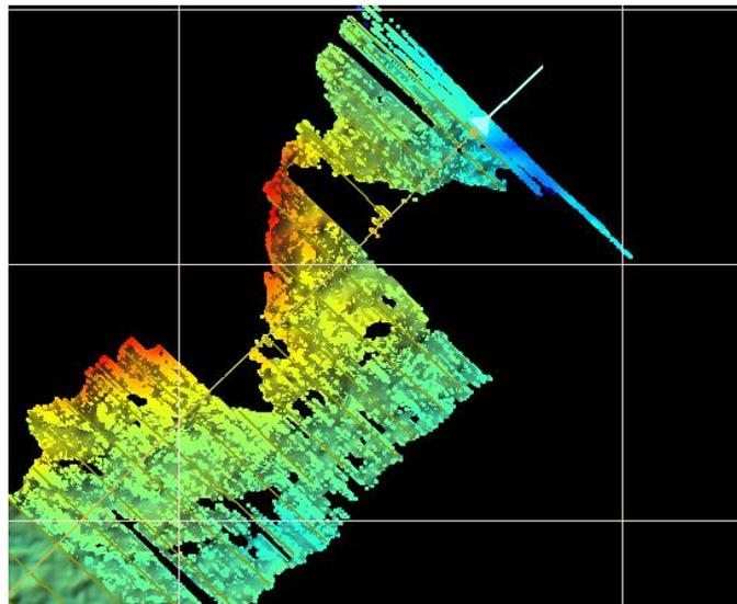
Figure 71. Bad swath. This bad data has been fixed by stop/starting the pinging.
