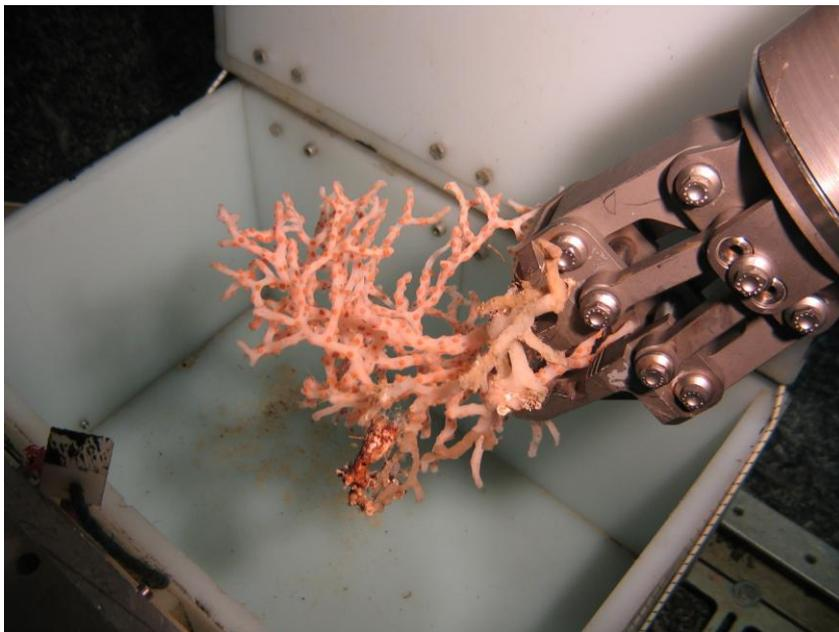
Figure 29. Orion arm being used to place sponge / zoanthid colony into port lidded-biobox.
