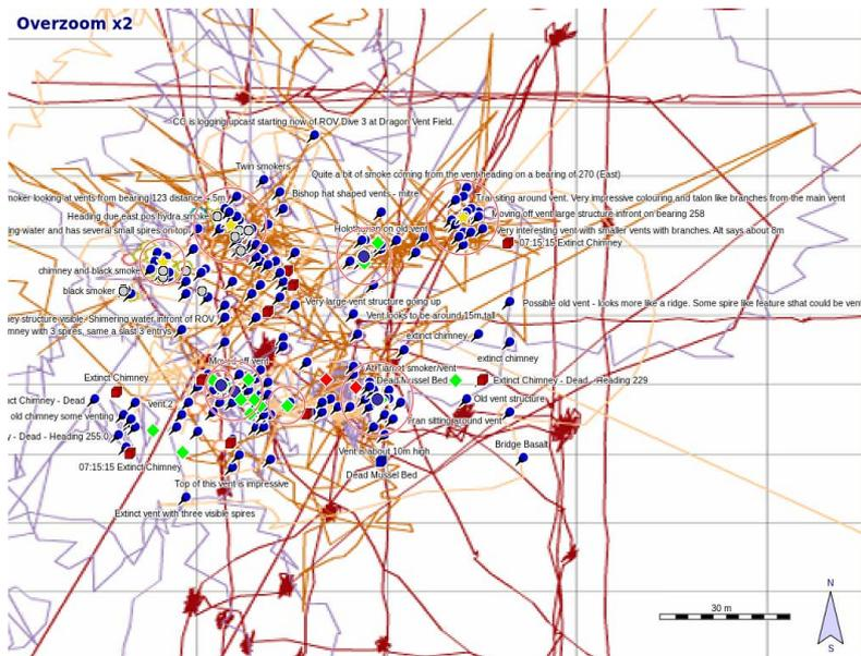
Figure 84. Example of a chart produced using the events logged in the event logger and then overlaid on the a track plot for the USBL/Ship position to show the position of vents and features during JC067.
