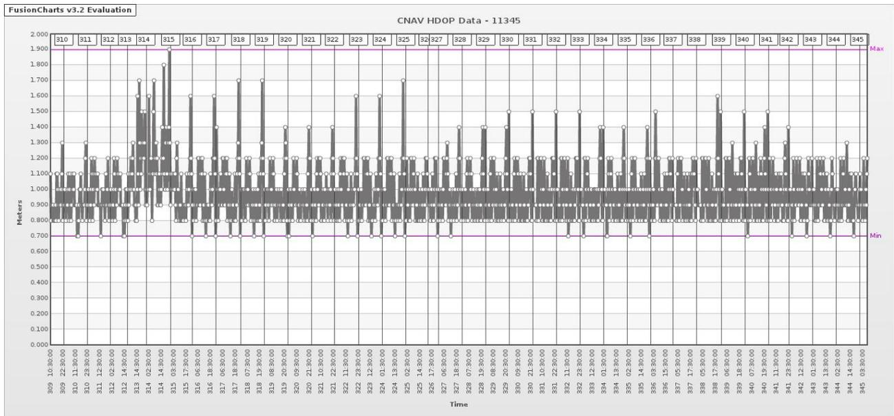
Figure 66. Despite “High Noise” errors on the DP system the actual HDOP values for the DPS116 were very good for the duration of the cruise.
