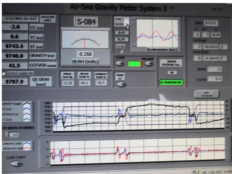
Figure 20. Screenshot of the gravimeter console. The black line represents corrected gravity values, while the purple line shows the EOTVOS correction. These are fluctuating periodically as the ship completes a swath survey passing over the seamount in different directions.
