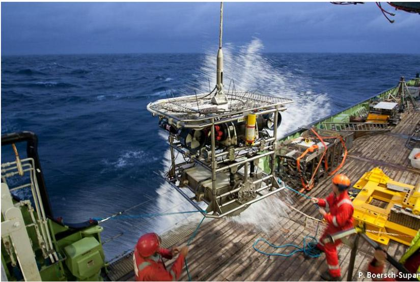
Figure 9. HYBIS towed camera and grab system being recovered on James Cook Cruise JC055. Photograph © Philipp Boersch-Supan.
