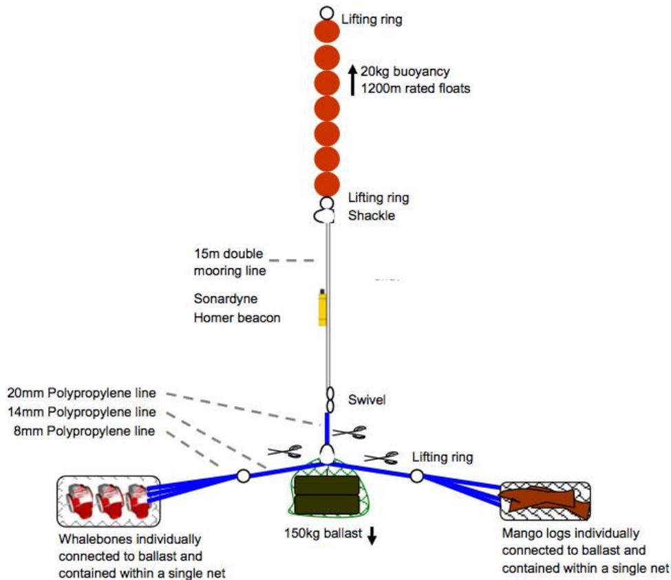
Figure 45. Mooring schematic. The scissor symbol designates where the ROV should cut during recovery.
