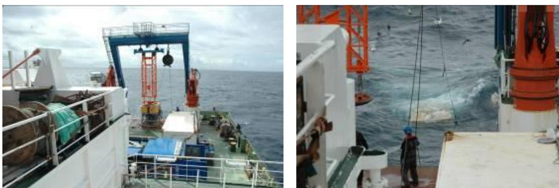
Figure 103. Deployment of ROV KIEL 6000 from the stern gantry of RRS *James Cook*. ROV still on deck (left) and in the water released from its latch (right).
