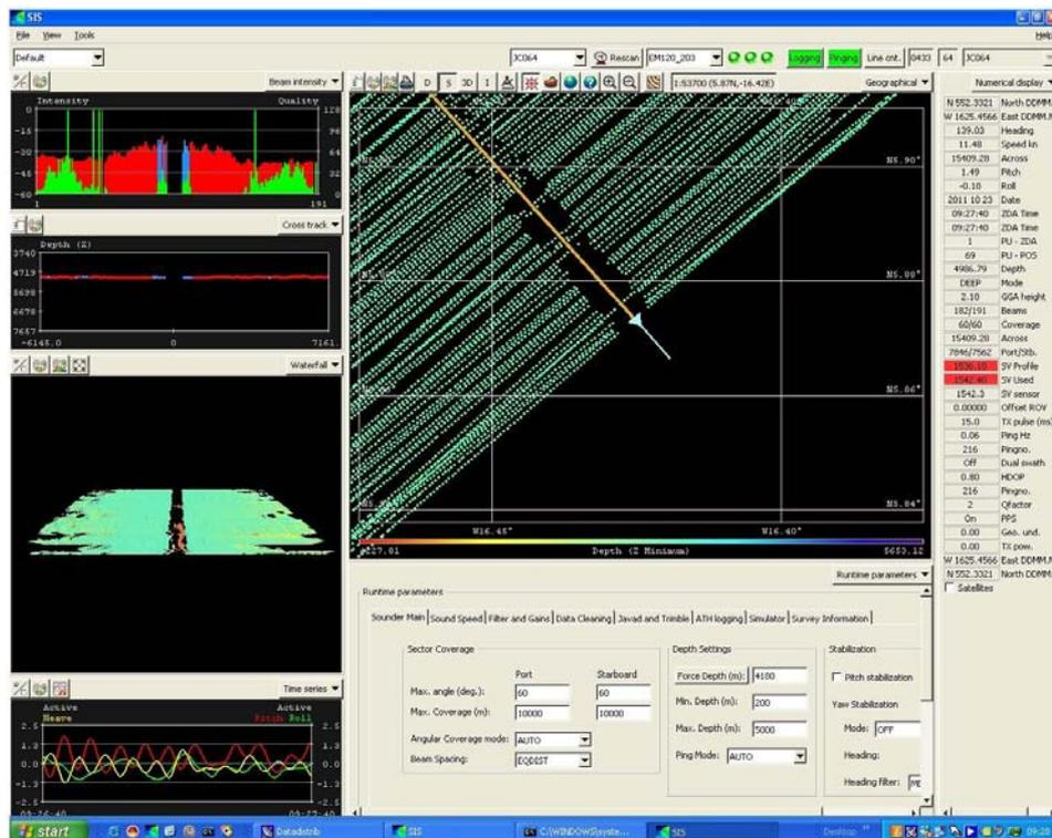
Figure 73. A similar issue occurred with a visible raised area below the vessel. As with the “no data” problem described above, this was solved restarting SIS.
