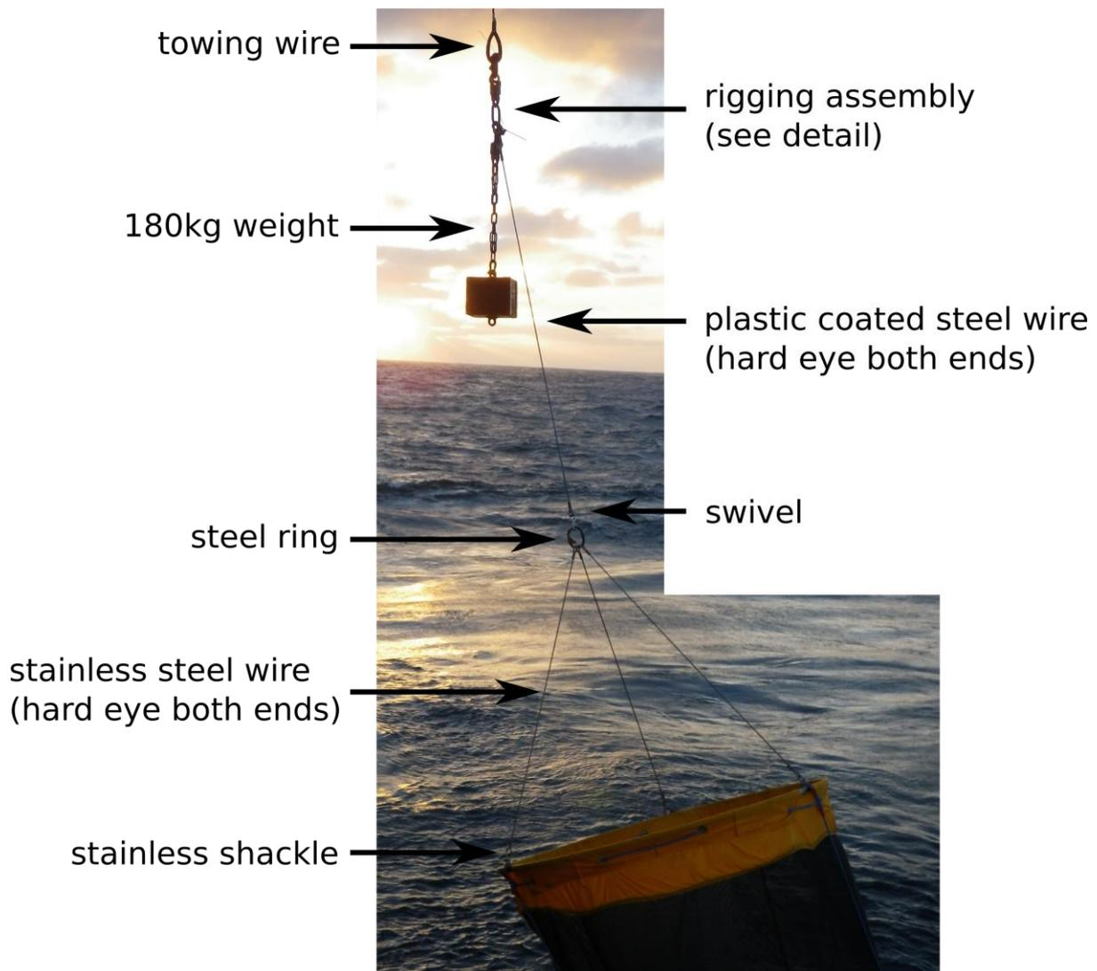
Figure 23. Bridle assembly for oblique towing of the large ring net.
