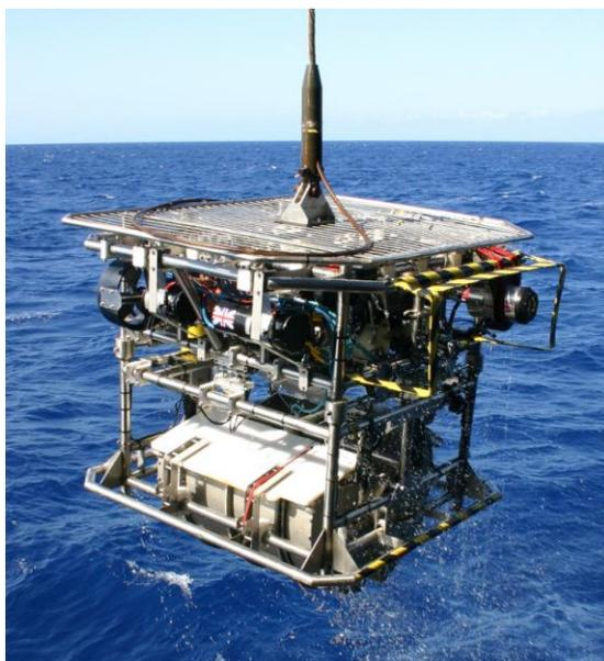
Figure 115. HyBIS vehicle with grab module.
