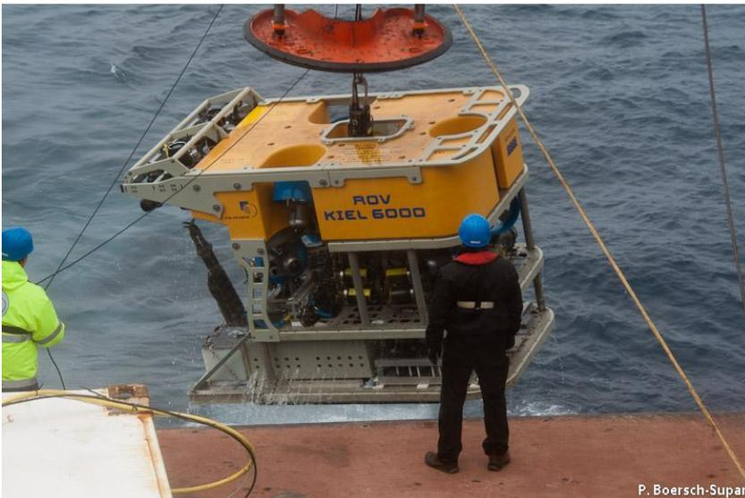
Figure 7. IFM Geomar *Kiel 6000* ROV system being recovered on *James Cook* Cruise JC066. Photography © Philipp Boersch-Supan.
