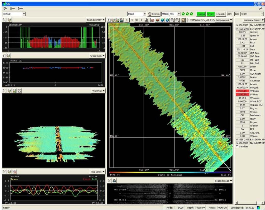
Figure 72. On one occasion during the cruise a problem occurred where no centre beam data was displayed in SIS. Stopping and restarting SIS solved this issue. During this stage we did not have an accurate sound speed profile.
