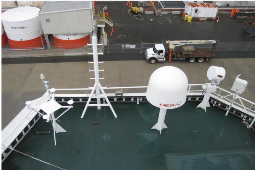
Figure 67. The ADU5 is the 4 antennas in the left of the image.
