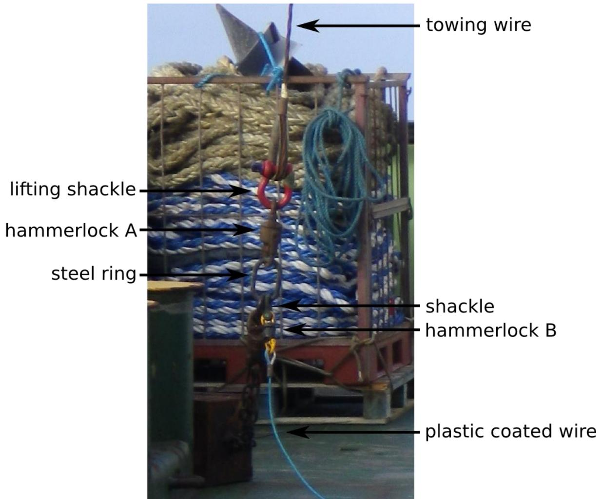
Figure 24. Detail of rigging assembly of the large ring net.
