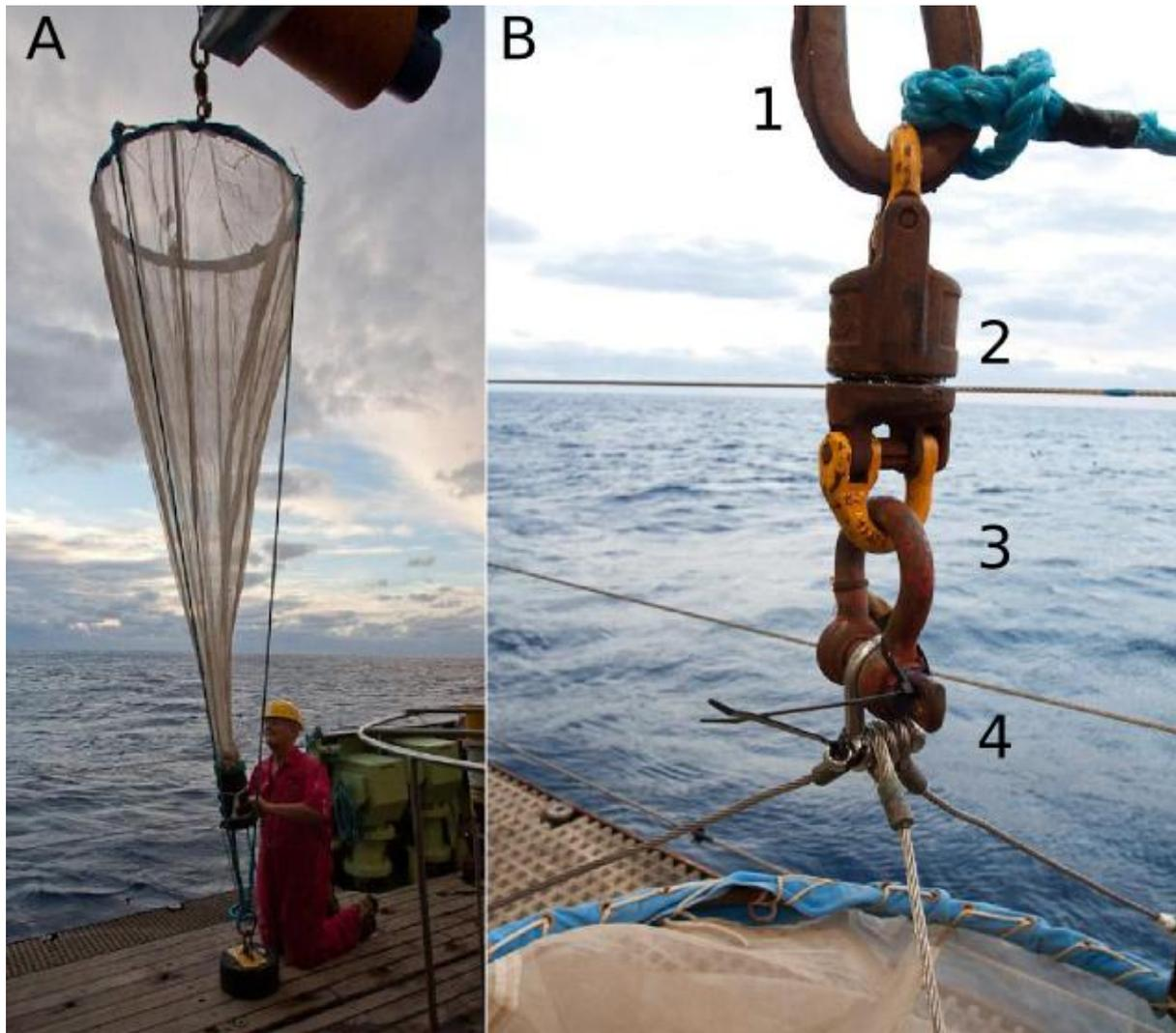
Figure 25. (A) Small ring net rigging overview. (B) Detail of connection between the towing wire (1) and the three-point bridle (4) using a hammerlock swivel (2) and a lifting shackle (3).
