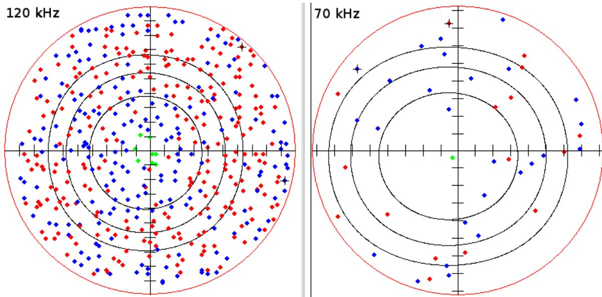
Figure 27. Single target detections of the 120 kHz transducer (left) and the 70 kHz transducer (right) during calibration of the EK60 echosounders on the RRS James Cook. This comparative example (the remaining three transducers were similar to the 120 kHz) shows there are significantly fewer single target detections on the 70 kHz than the other transducers.
