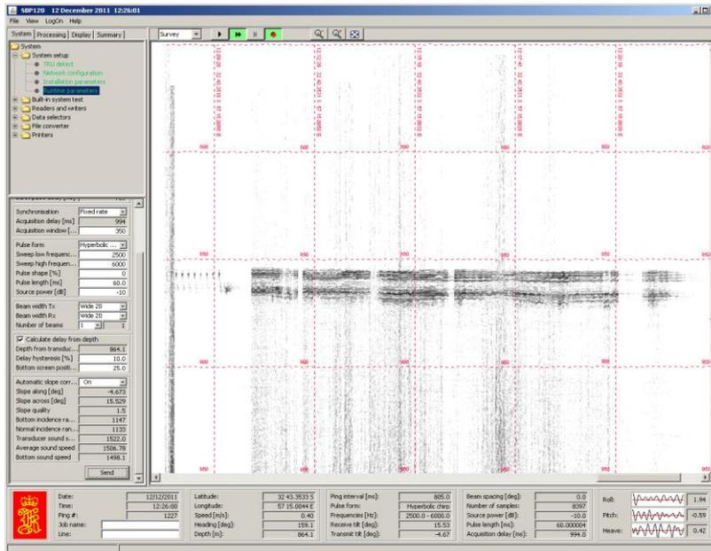
Figure 74. SBP profile from seamount showing minimal penetration of seabed.
