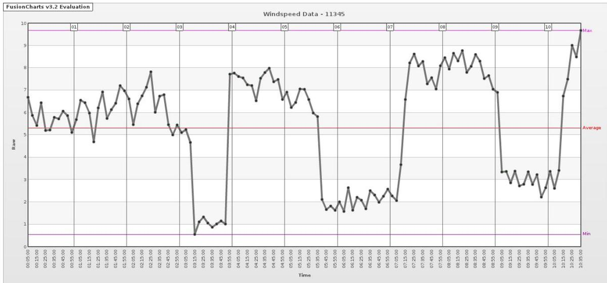
Figure 93. Graph showing evidence of wind speed sensor blocking.
