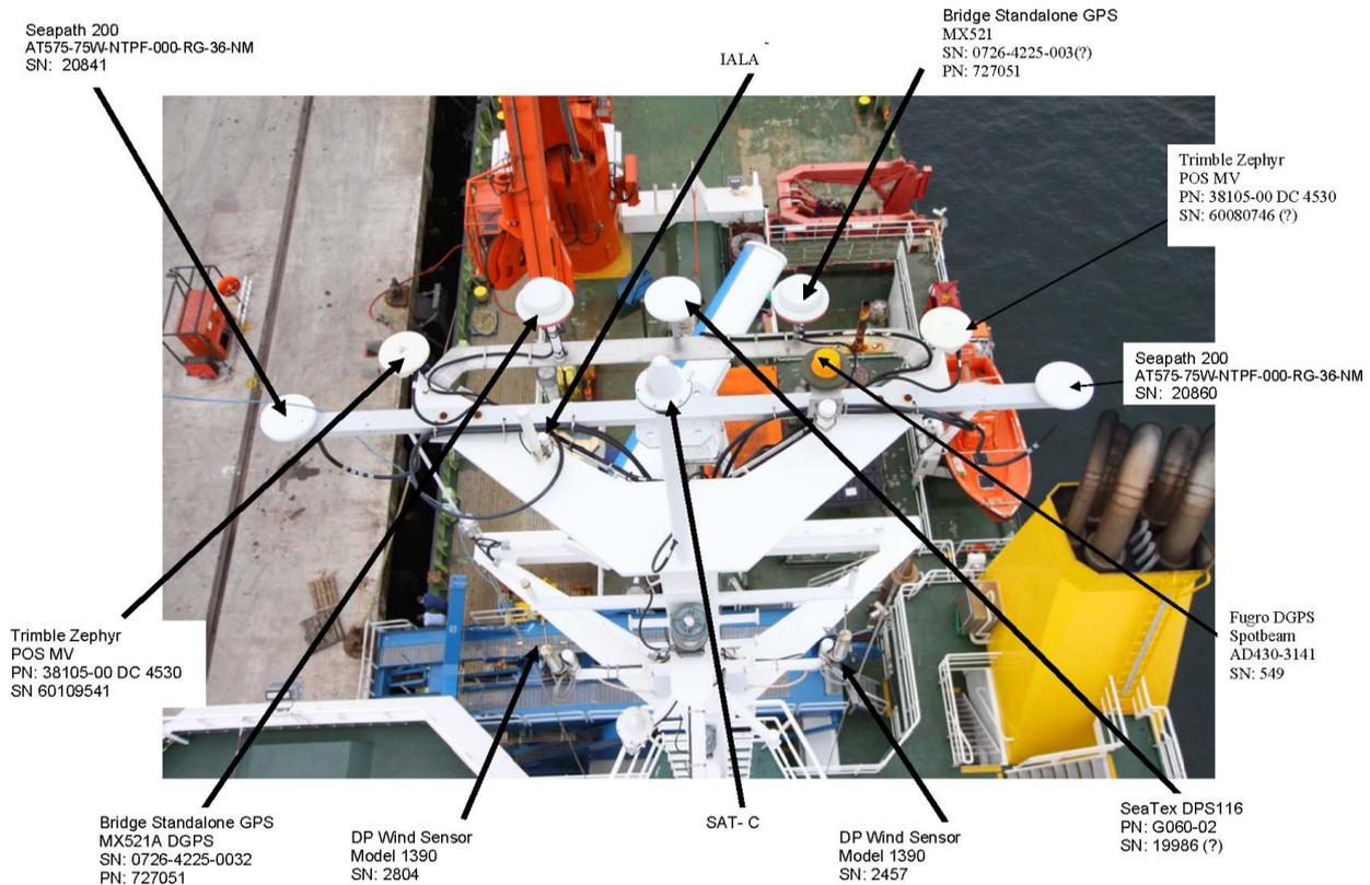
Figure 65. Pre 2011 set-up. The only difference is the Spotbeam has now been replaced by the CNAV antenna which occupies the same position.
