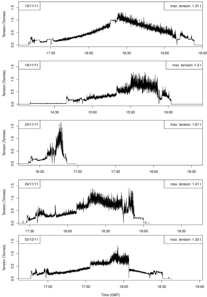
Figure 26. Records of wire tension during deployments of large ring nets. Note the sudden drop in tension in the last panel at approximately 18.06 GMT.
