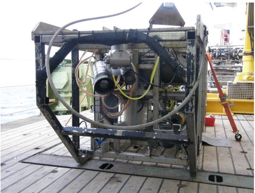
Figure 8. SHRIMP (Seabed High Resolution Imaging Platform) towed camera system. Photograph © Dr Jane Read, NERC.
