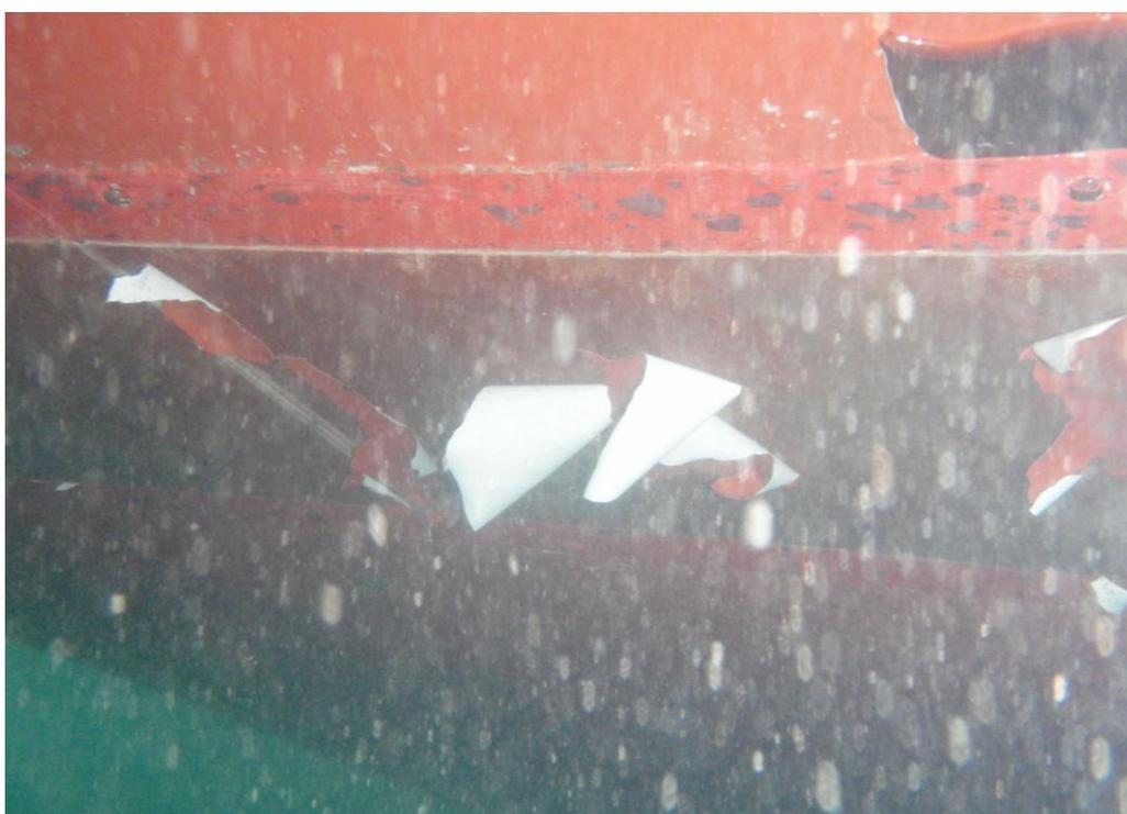
Figure 70. Paint peeling on EM120 transducers.
