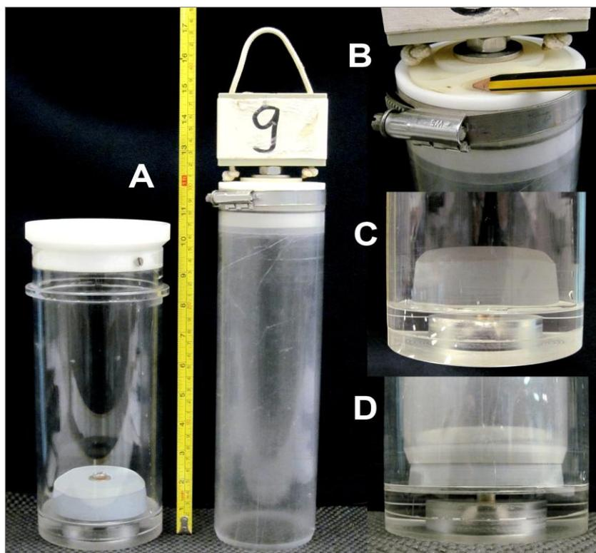
Figure 43. Design of the *Kiel* 6000 Push Core system. A: Complete system showing quiver on the left and core on the right, B: Detail of top insert showing silicone flap valve, C: Detail of base of quiver showing fixed sealing bung, D: Detail of push core seated on sealing bung.
