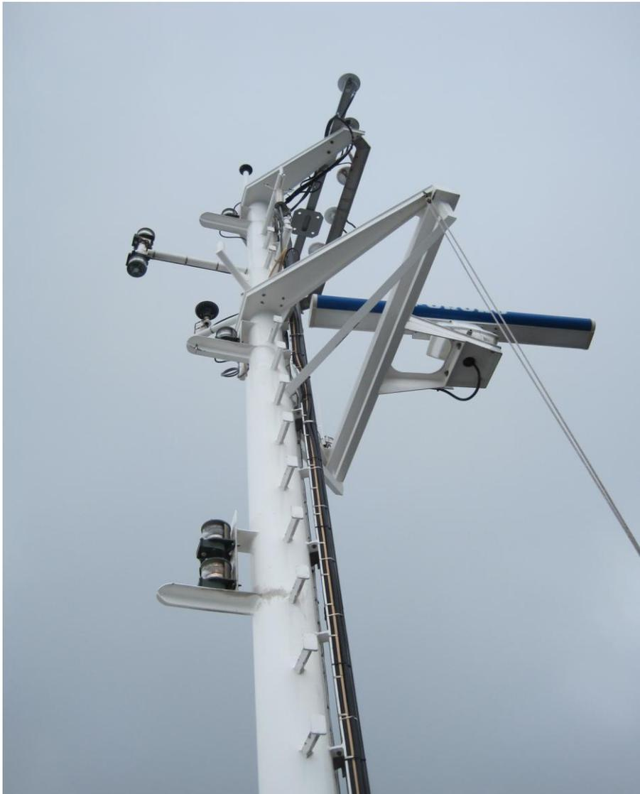
Figure 101. This image shows how far from the actual mast the radar unit and motor assembly are located.
