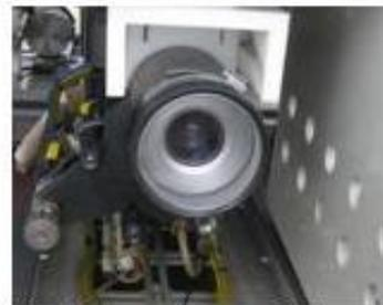
**Fig. 5:** Forward looking HD camera with laser array
