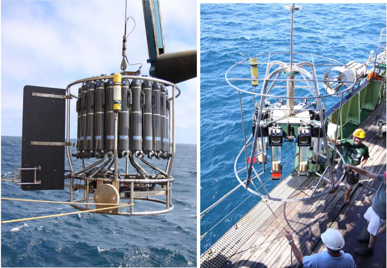
Figure 88. Photographs showing the mounting of USBL beacons on the CTD and Megacorer.
