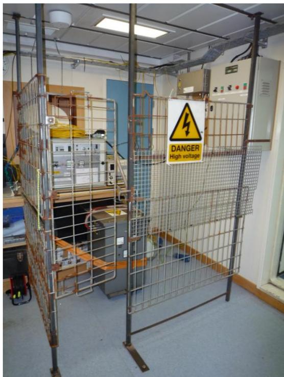
Figure 117. HV enclosure in the main lab.
