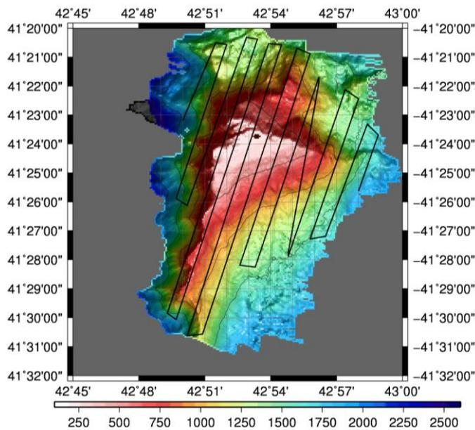
Figure 13 – Coral seamount bathymetry with cruise tracks
