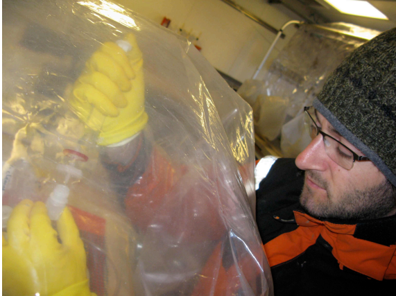
Figure 15. Low temperature in-line separation of porewater colloids from the dissolved size fraction under N 2 atmosphere.
