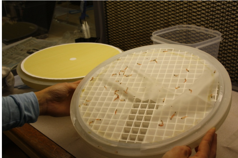
Figure 29: Particles collected onto PES filter (distant) and Nitex mesh (front). In this deployment Nitex mesh 'caught' a lot of krill
