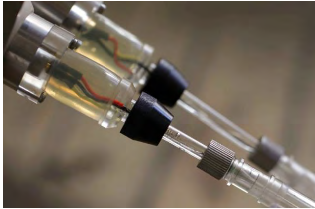
Figure 6.33 The acrylic pressure-compensated microelectrode housings used during JC073
