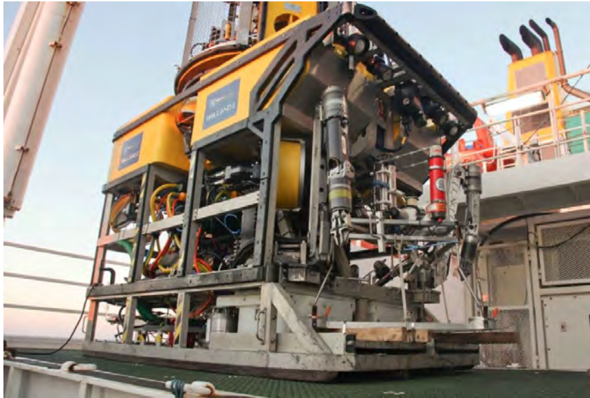
Figure 6.32 The JC073 AEC lander system mounted onto the Holland-1 ROV ready for deployment.
