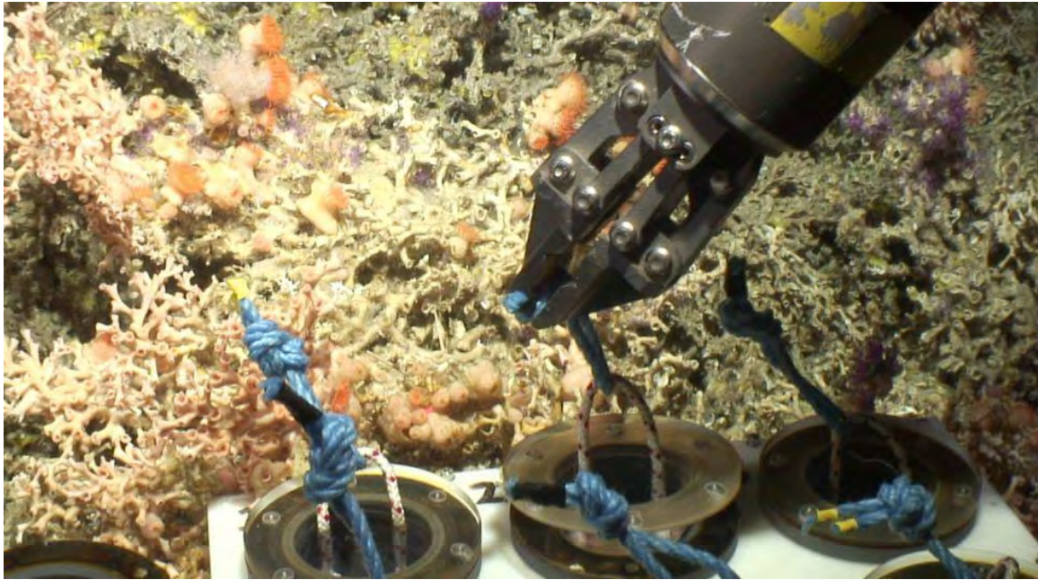
Figure 6.19 The self-seating lid easily adheres to the open-end of the canister.
