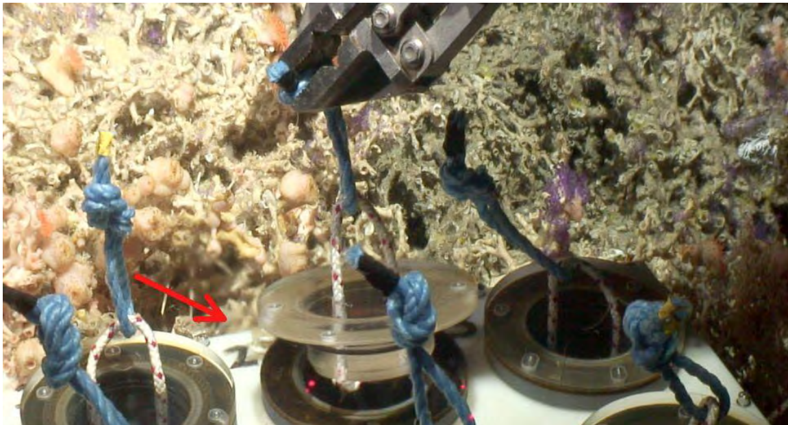
Figure 6.12 The starboard manipulator arm grasps positively buoyant rope and removes a lid from one of the canisters in the sampling array. Freshwater is immediately displaced by seawater, as can be seen by the cloudy disturbance next to the arrow in the above photograph.
