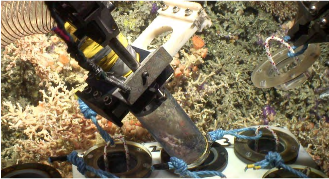
Figure 6.17 The slurp gun and associated coral fragments are positioned in the mouth of a dedicated canister. As can be seen in the above photograph, the coral fragments gently slide into a container when vacuum suction is stopped.
