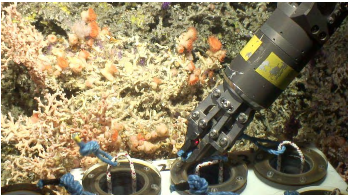
Figure 6.20 With only a modest amount of encouragement from the starboard manipulator arm, the lid is pushed into position to create a watertight seal that retains the Lophelia fragments at constant ambient water temperature and salinity.
