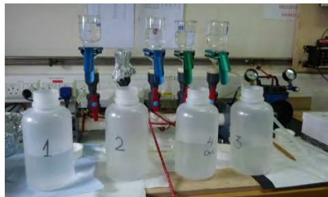
Figure 6.7 Filtration set-up used on board RRS James Cook . The bottles contain the sampled water used in each experimental and control chambers.
