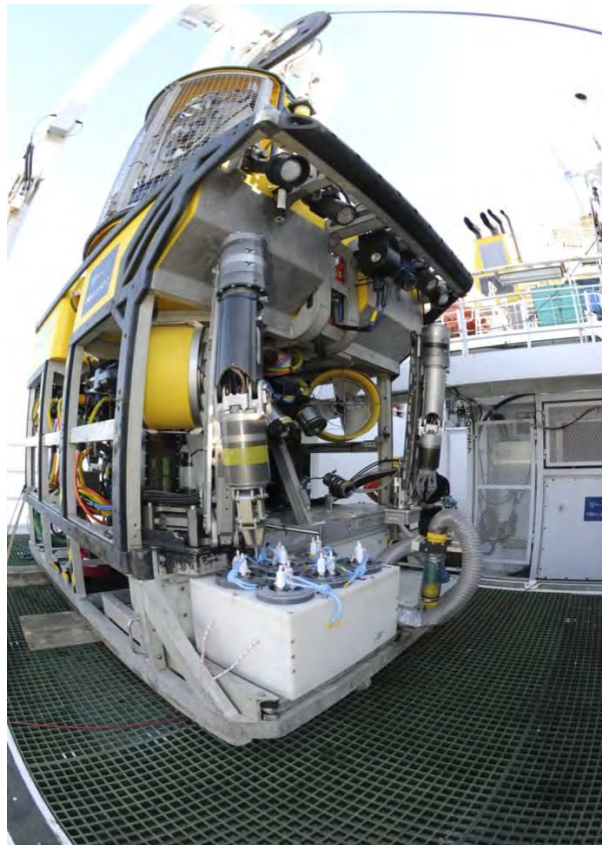
Figure 6.11 The sampling array, nested within a standard biological box, attached to the forward starboard footprint of the ROV Holland-1 .
