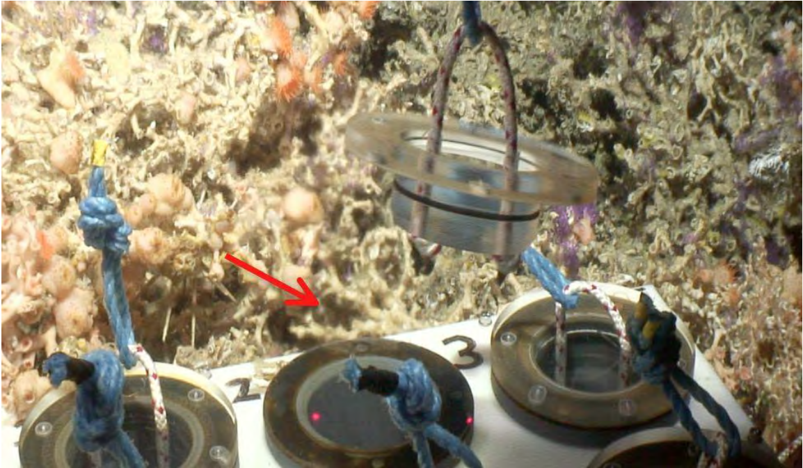
Figure 6.13: Moving the lid away from each canister allows the complete overturn of freshwater to ambient seawater. Freshwater rising out of canister #2 can be seen next to the arrow in the above photo.
