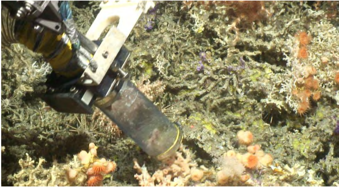
Figure 6.15 The acrylic extension tube of the suction sampling mechanism is gently grazed across a colony of L. pertusa . A mild vacuum lifts small coral fragments away from the substrate and holds them against a mesh screen positioned at the base of the extension tube.
