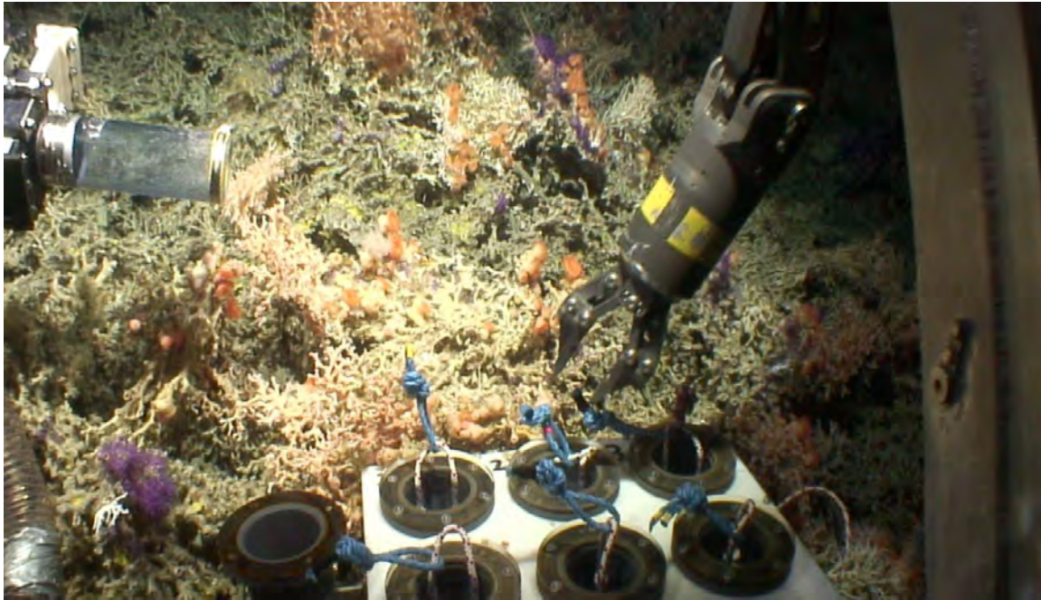
Figure 6.21 The slurp gun is pointed into the water column and full suction applied. This procedure serves to remove any residual biological material from the mesh screen before proceeding to collect additional samples.
