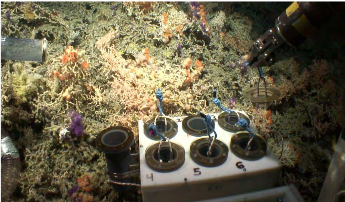
Figure 6.14 With a lid held securely by the starboard manipulator arm, the port manipulator arm grasped the ROV's slurp gun—seen in the upper left corner of the above photograph—in preparation for collecting live coral samples.
