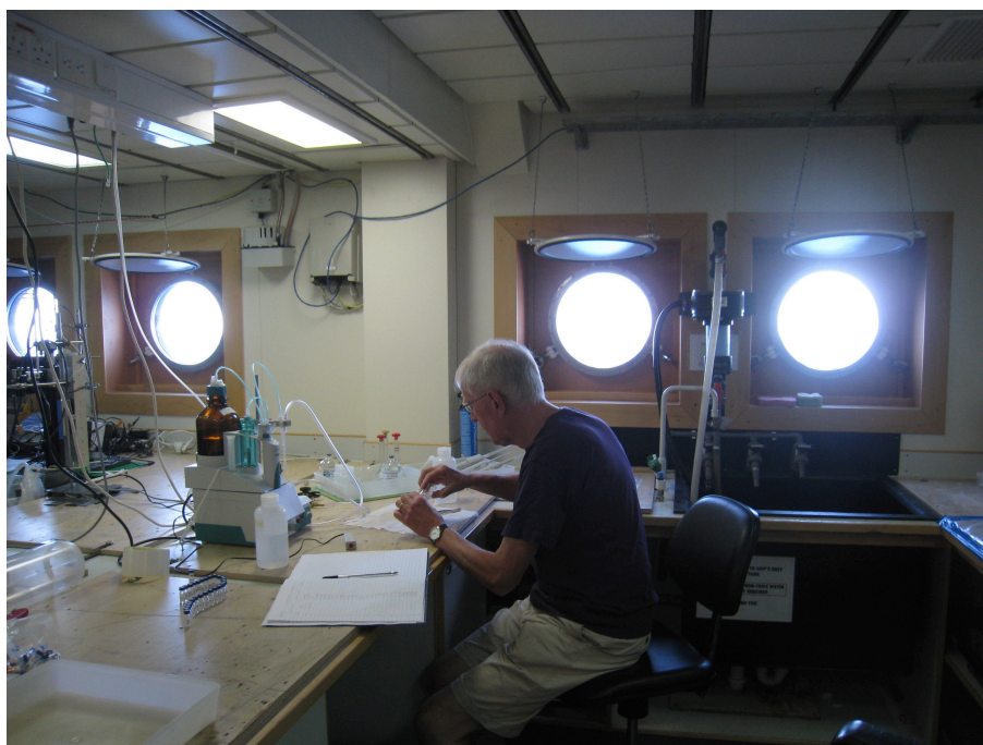
Fig. 19. Titration of pore-water samples for the determination of alkalinity
