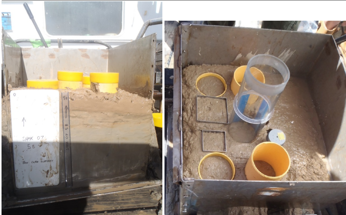
Fig. 10. Box Cores showing (L) sampling of side with tray and U-channel and (R) tubes of various types and surface sampling guides. Clear plastic tube is pre-drilled to take Rhizons.
