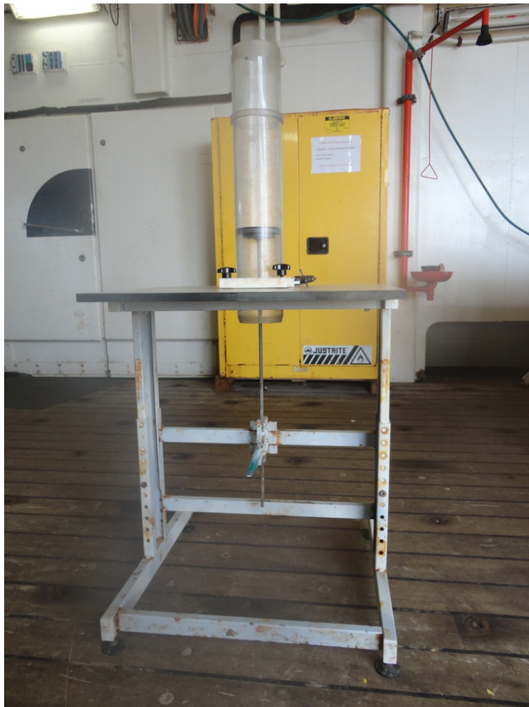
Fig. 15. Purpose-built table for extruding and sampling megacore tubes. Designed and fabricated at the University of Cambridge.
