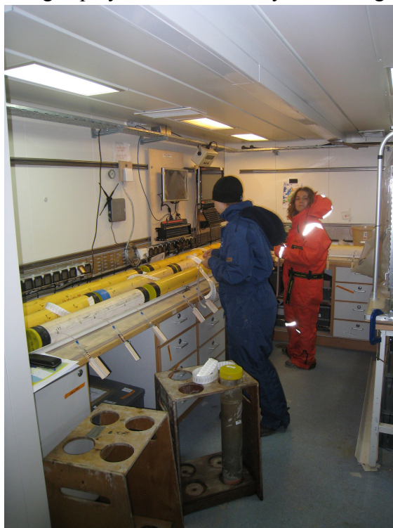
Fig. 18. Anna-Lena Grauel and Maria de la Fuente fitting Rhizon samplers to sections from a Piston Core
