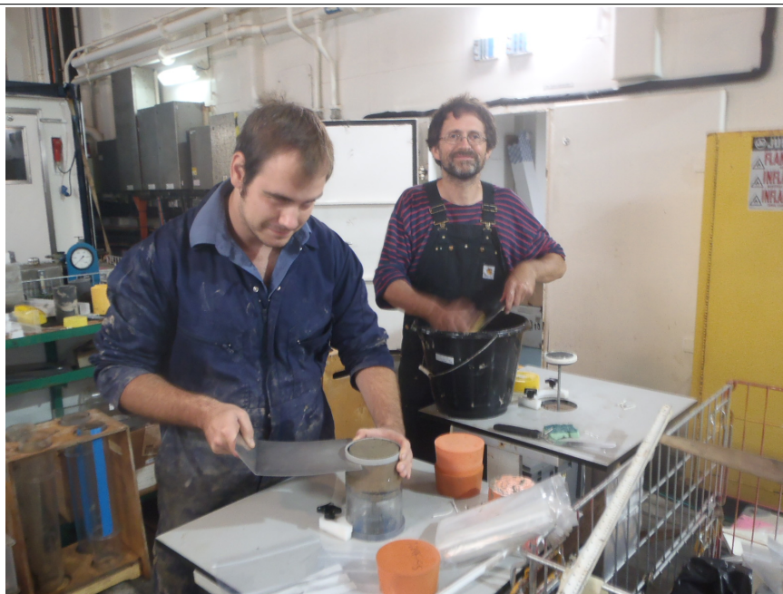
Fig. 16. Sampling of a Megacore tube using the Cambridge extruding and sampling table.
