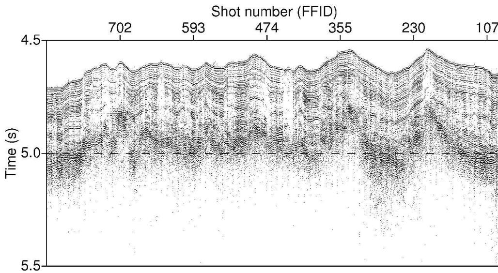
Figure 4.11. QC migration of part of seismic reflection profile RS\_A (GI), over the same range as Fig. 4.10. Note the vertical scale change to highlight the high-frequency content of this profile.
