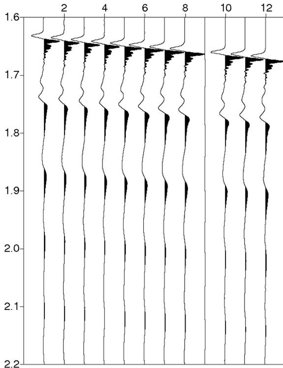
*Figure 2.19. Single shot from the Bolt array recorded on the vertical hydrophone array VA\_01. Channel 1 is the shallowest and channel 12 is the deepest. Channel 9 suffered a broken wire in its connection cable during deployment.*
