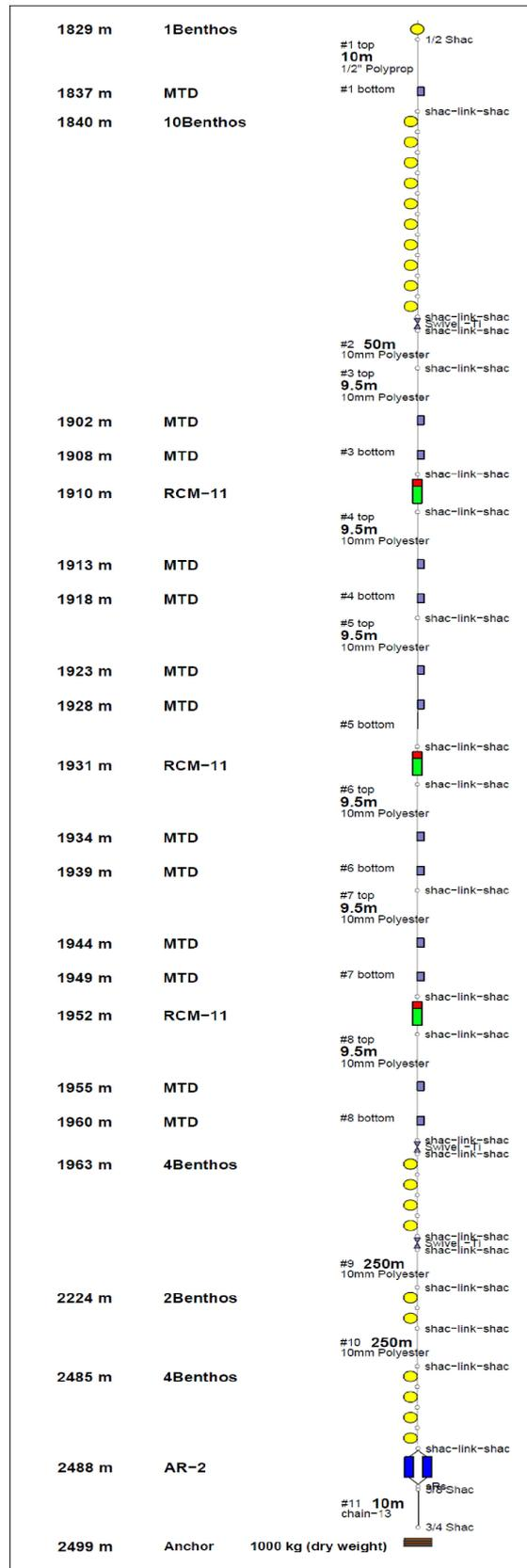
Figure 2.18. Mooring design for vertical hydrophone arrays (VA\_01 & VA\_02). RCM-11 units are data loggers provided by OBIF; MTD are mounting points for individual hydrophones; AR-2 are acoustic releases
