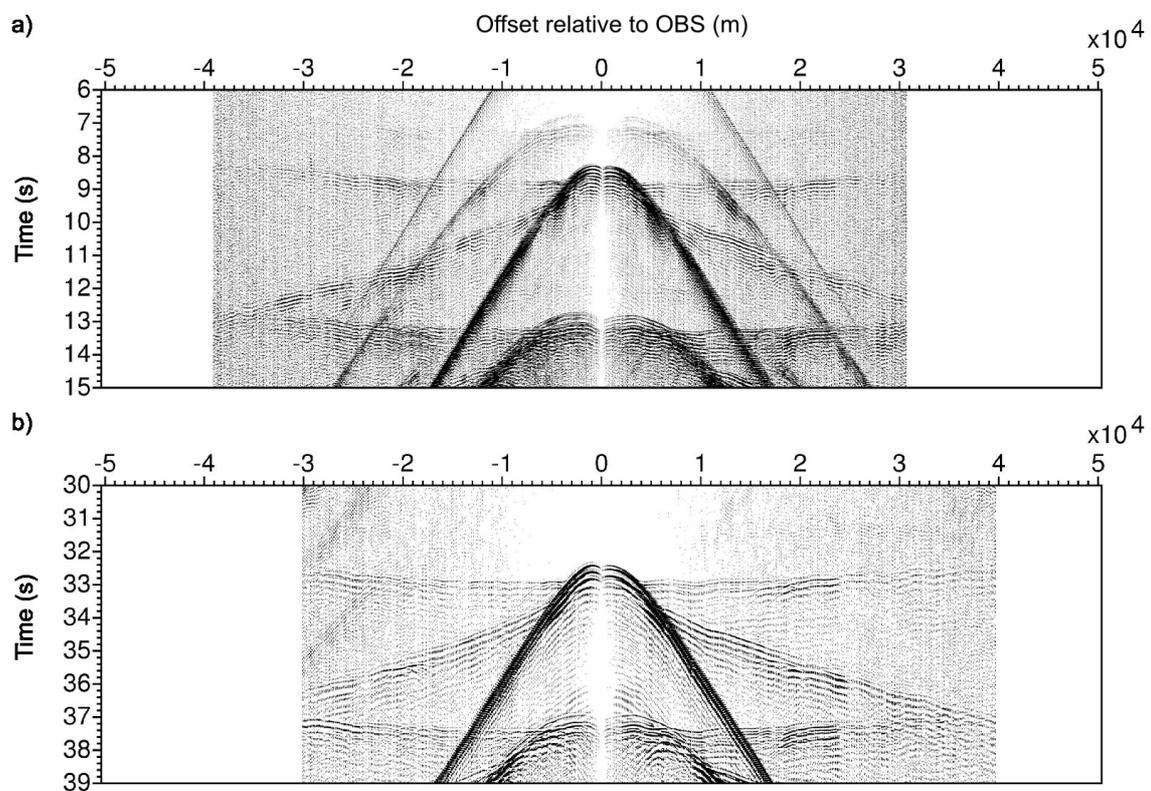
Figure 2.15. Example data from the hydrophone channel for an OBS recording the two-ship SAP\_B profile from the South Grid, plotted reduced at  $8 \text{ km s}^{-1}$ . (a) Record section from the COOK Bolt source. (b) Record from the SONNE G source.
