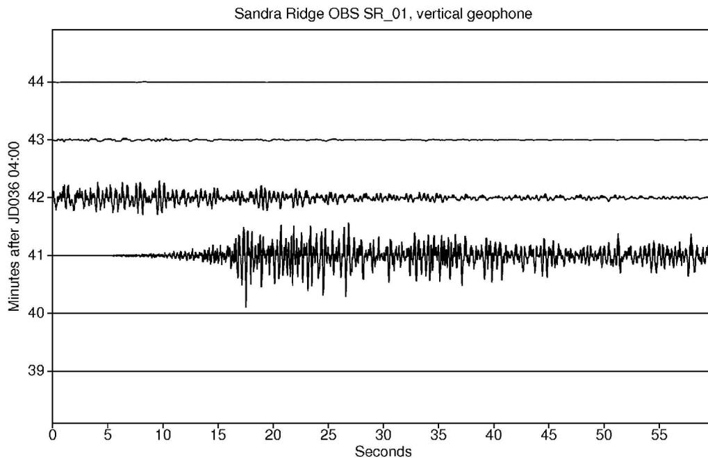
Figure 2.17. Vertical geophone record from the OBS passive monitoring array at the Sandra Ridge (SR\_01) of magnitude 5.7 earthquake in the adjacent Panama Fracture Zone
