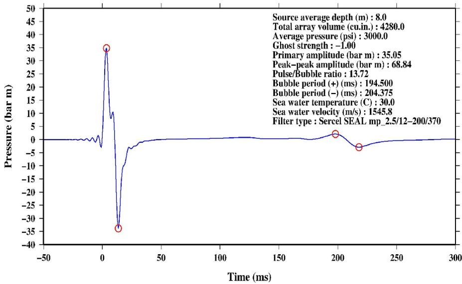
Figure 2.6. Layout and predicted source signature from the SONNE G airgun array, modelled using the PGS Nucleus+ software.
