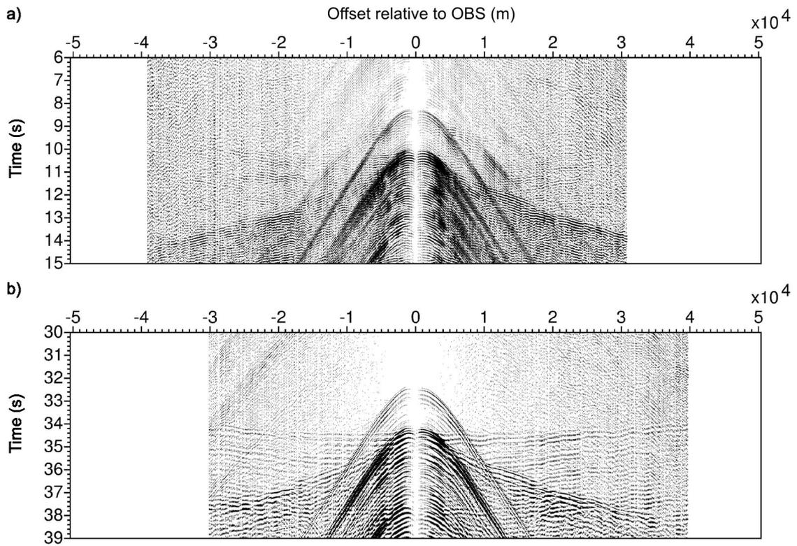
Figure 2.16. Example data from a horizontal geophone channel for an OBS recording the two-ship SAP\_B profile from the South Grid, plotted reduced at  $8 \text{ km s}^{-1}$ . (a) Record section from the COOK Bolt source. (b) Record from the SONNE G source.
