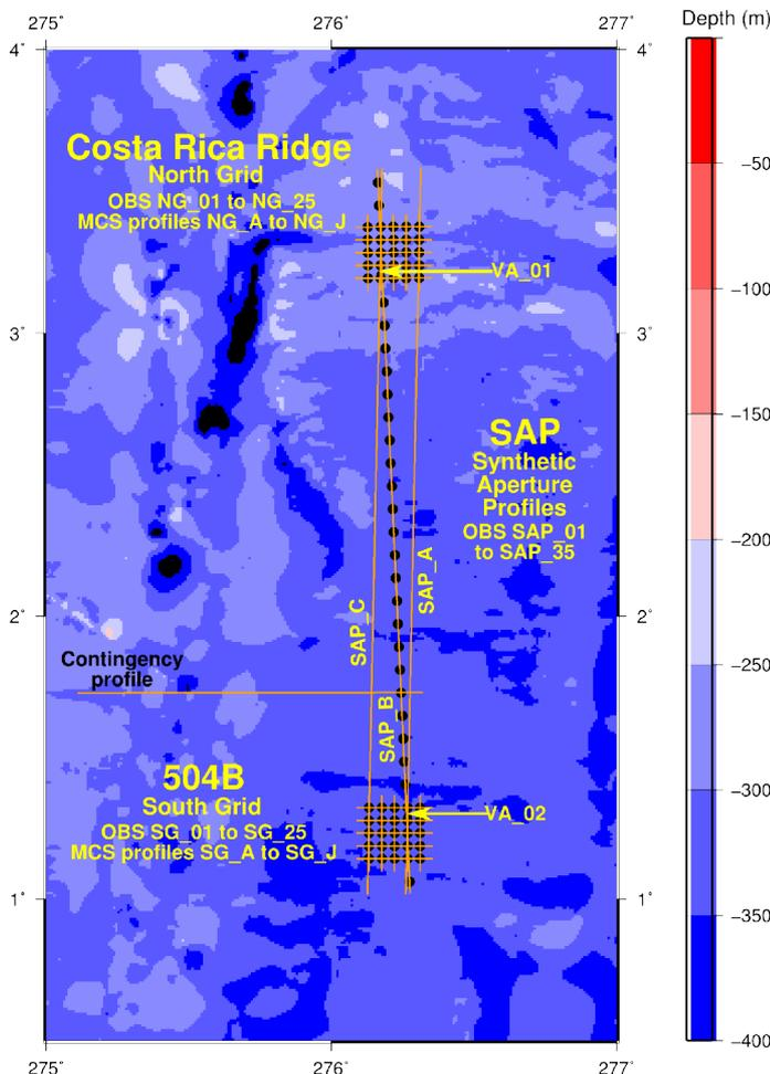
Figure 1.4. JC114 cruise plan with two grids, one centred on the Costa Rica Ridge (North Grid, NG) and one on ODP 504B (South Grid, SG), with three synthetic aperture profiles (SAP) linking the grids together. OBS and vertical array (VA) locations marked by black dots.
