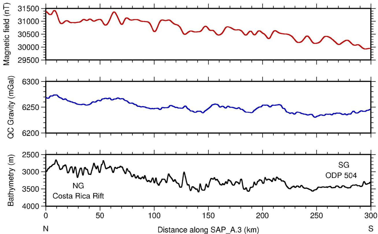
Figure 5.4. Example of potential field data (free-air gravity and magnetic field) plotted for the north-south profile SAP\_A with bathymetry extracted from the EM120 multi-beam echo sounder. Both the gravity and magnetic data have had a 5 km moving average filter applied for QC display purposes.
