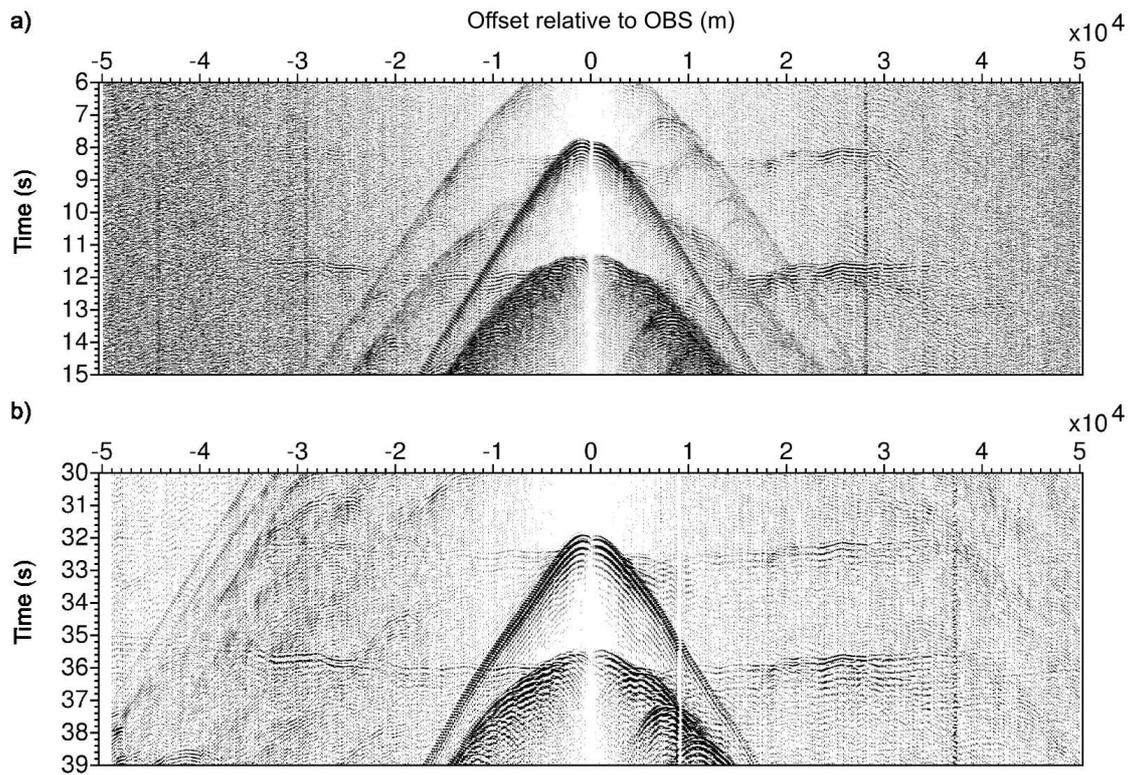
Figure 2.14. Example data from the hydrophone channel for an OBS recording the two-ship SAP\_B profile from the North Grid, plotted reduced at  $8 \text{ km s}^{-1}$ . (a) Record section from the COOK Bolt source. (b) Record from the SONNE G source.
