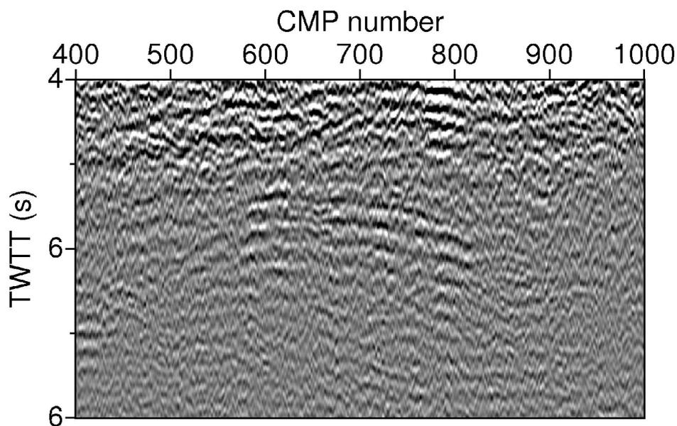
Figure 4.4. Section of brute stack MCS data from NG\_BB (CMP equivalent of shot points 250 to 650) showing the reflection from the axial magma chamber between CMP 600 to 800.
