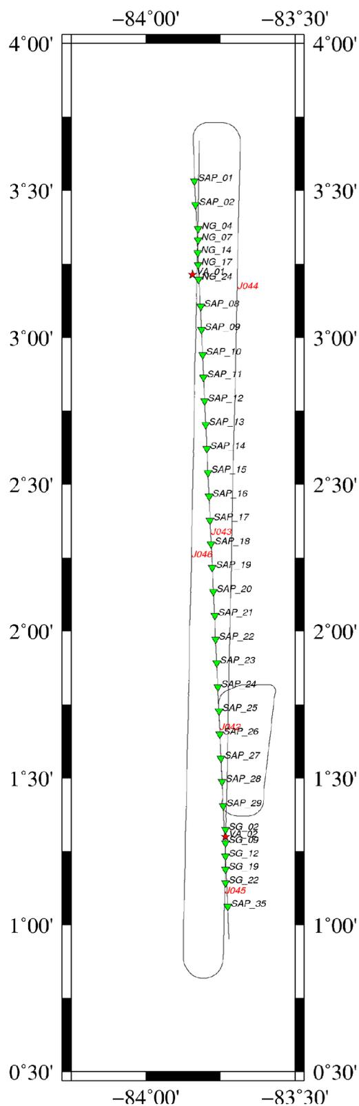
Figure 2.13. OBS (green triangles) and vertical arrays (red stars) locations for the Synthetic Aperture Profiles (SAP) area with ship-track of the recorded airgun sources.
