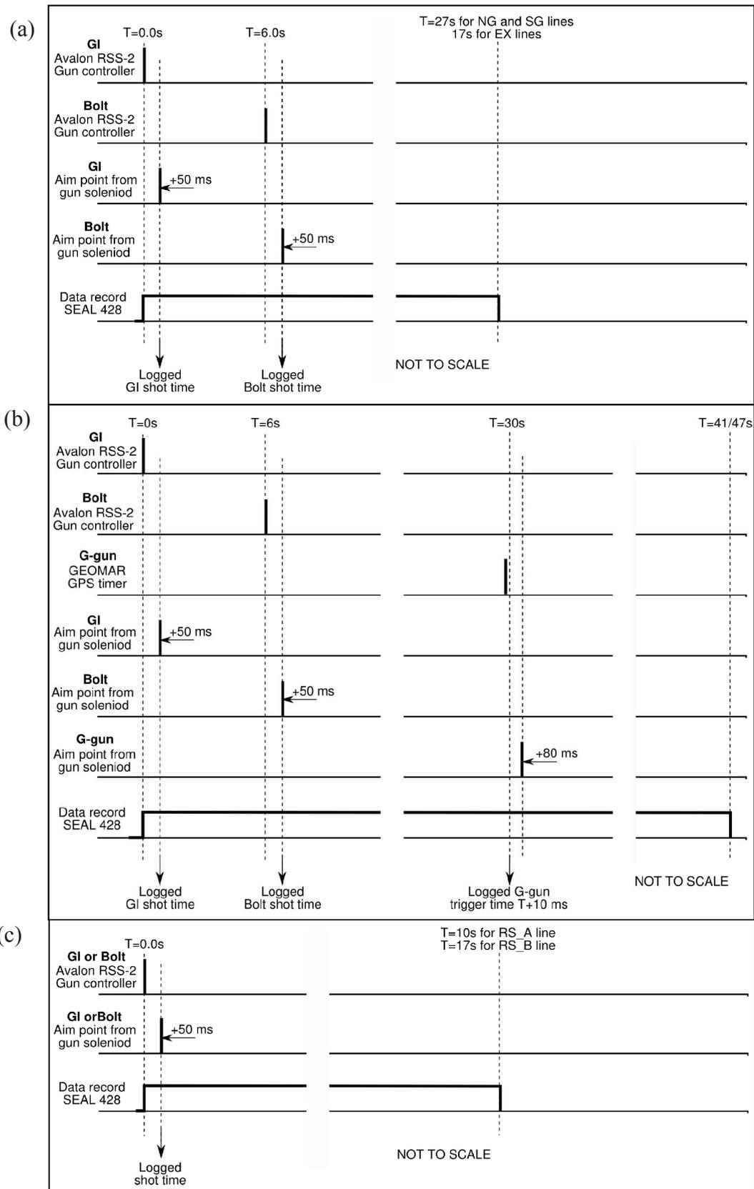
Figure 2.1. Timing diagrams showing trigger, shot fire time “aim point”, logged shot time and record length for the multichannel seismic reflection data: (a) timing for the NG and SG profiles; (b) timing for the SAP profiles; (c) timing for the RS profiles.
