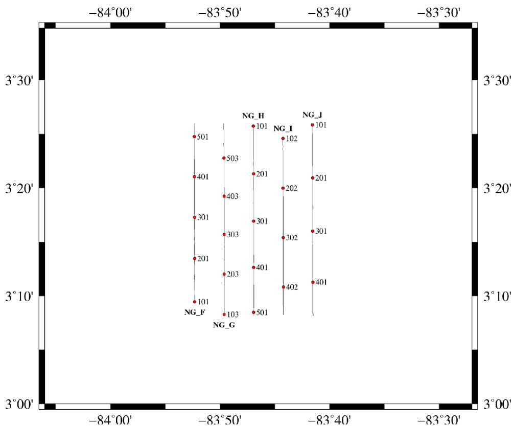
Figure 4.1. Multichannel seismic profiles shot within the North Grid. These profiles were shot with a 1500 m streamer. Shot point numbers (FFIDs) are annotated. The active Cost Rica Rift ridge segment lies along NG\_B.
