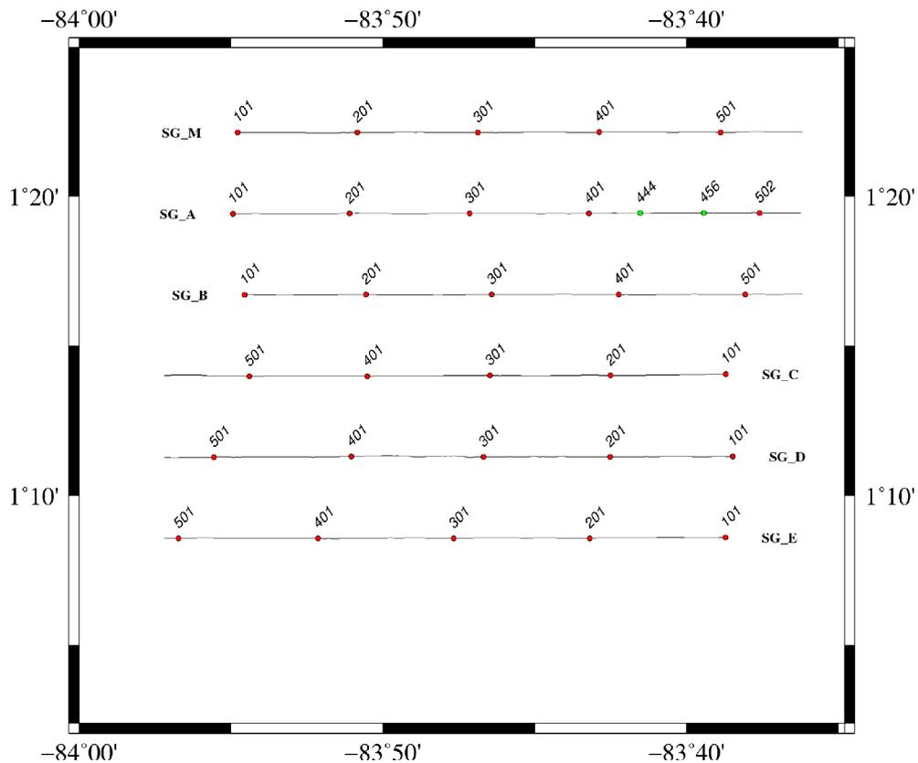
Figure 4.9. Multichannel seismic profiles shot within the South Grid. These profiles were shot with a 4500 m streamer. Shot point numbers (FFIDs) are annotated. The ODP 504B borehole lies at the intersection of lines SG\_C and SG\_I.
