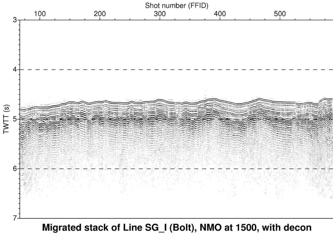
Figure 4.10. QC migration of seismic reflection profile SG\_C (Bolt) processed at  $1500 \text{ ms}^{-1}$
