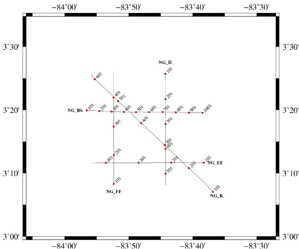
Figure 4.2. (a) Track chart for the reshoot of the NG grid with the 4500 m streamer configuration. Shot point numbers (FFIDs) are annotated.
