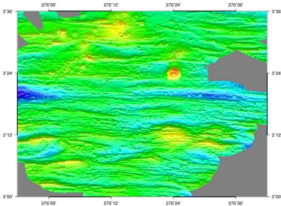
Figure 5.2. Multibeam swath bathymetry map for the North Grid area that spans the Costa Rica Ridge illuminated from the south.
