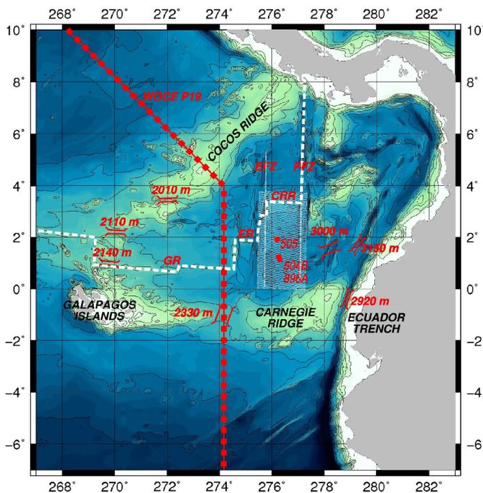
Figure 1.2. Map of the Panama Basin bounded by the Cocos and Carnegie Ridges. The spreading centre (white dashed line) and the EFZ (Ecuador Fracture Zone) and the PFZ (Panama Fracture Zone) which bound the CRR (Costa Rica Ridge) are marked. WOCE P19 is the track of the World Ocean Circulation Experiment PO profile; ODP drill sites are marked as dots, as are the location of sills and their respective depths (parallel lines). The white shaded box shows the principal research area for JC114.
