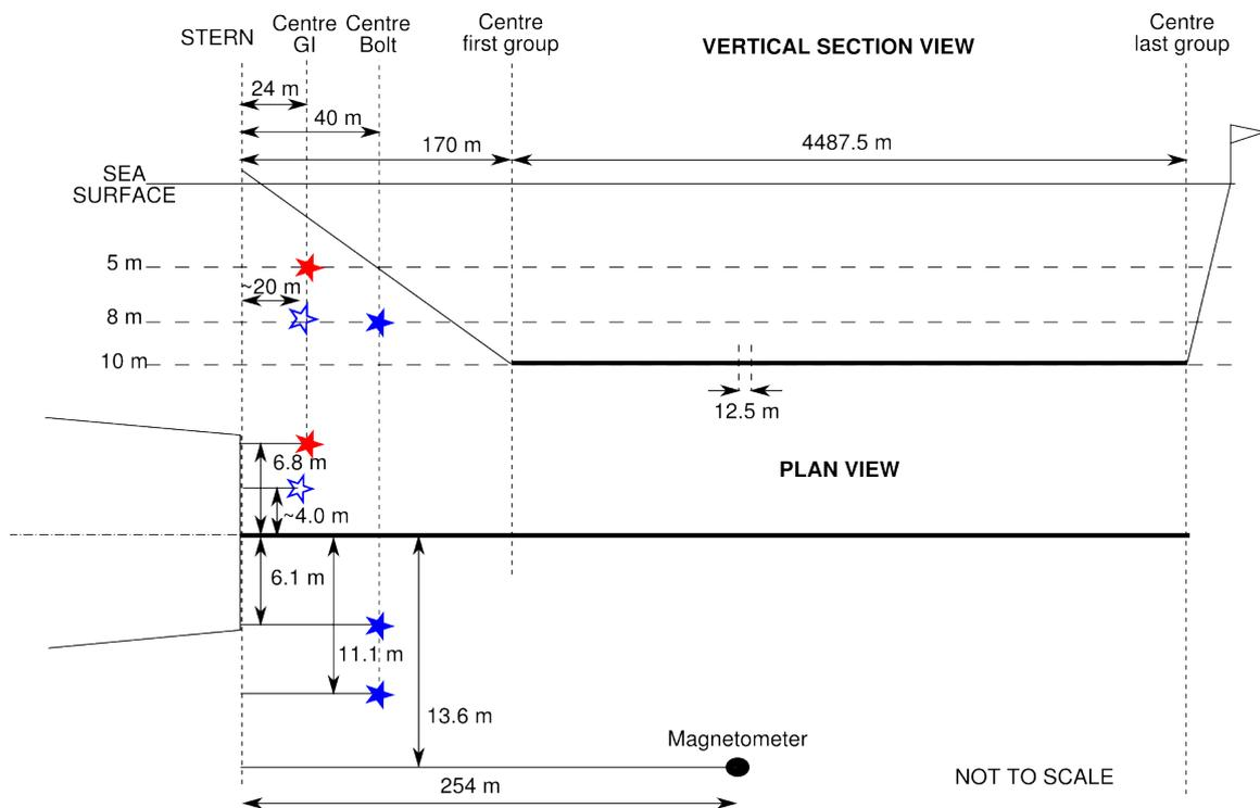
Figure 2.4. Layout of airgun sources and streamer used for the NG, SG, EX and SAP profiles; red – GI sub-array; blue – Bolt sub-array; filled stars represent centre-sub-array locations; the open star represents the additional single Bolt 500 in<sup>3</sup> gun towed for the EX, SG and RS\_B profiles.
