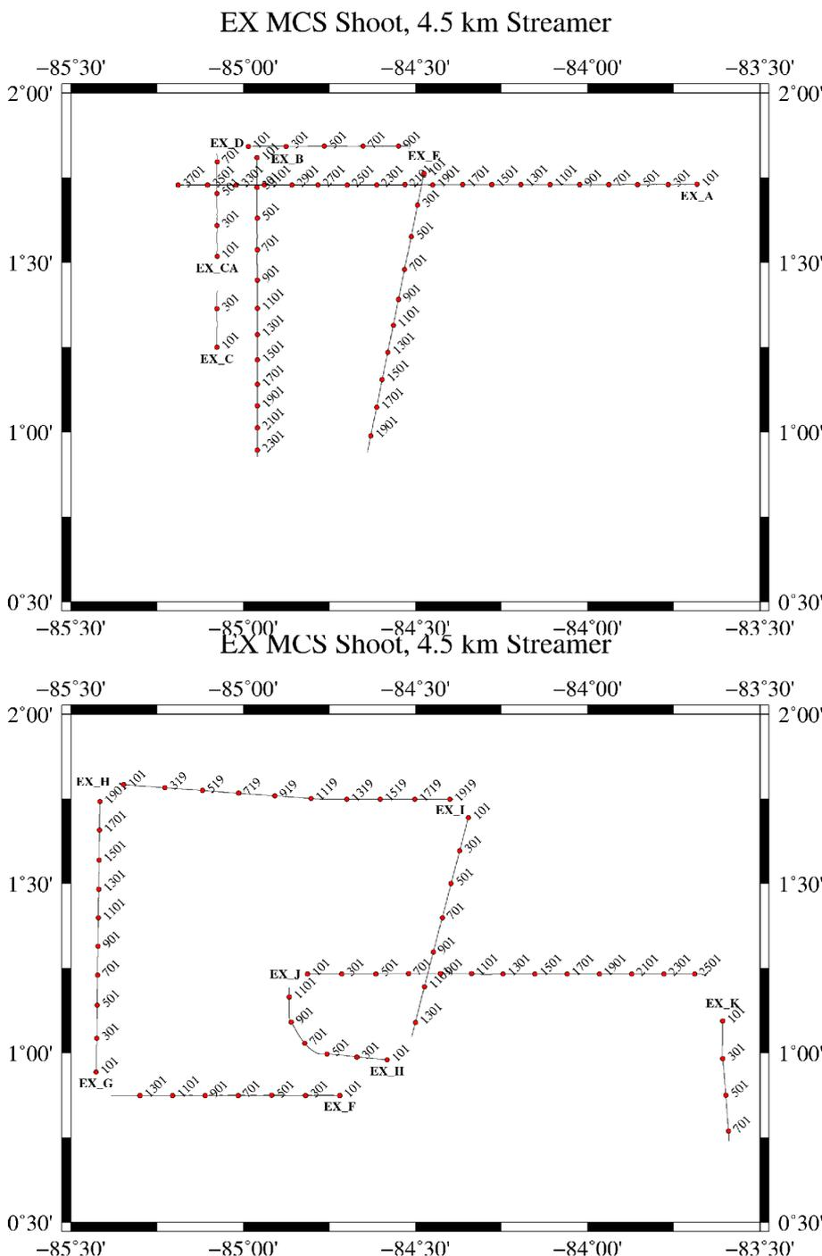
Figure 4.5. Multichannel seismic profiles shot within the Extended survey over the Ecuador ridge and Ecuador and Panama Fracture Zones. These profiles were shot with a 4500 m streamer. Shot point numbers (FFIDs) are annotated. The active ridge segment lies along EX\_A.
