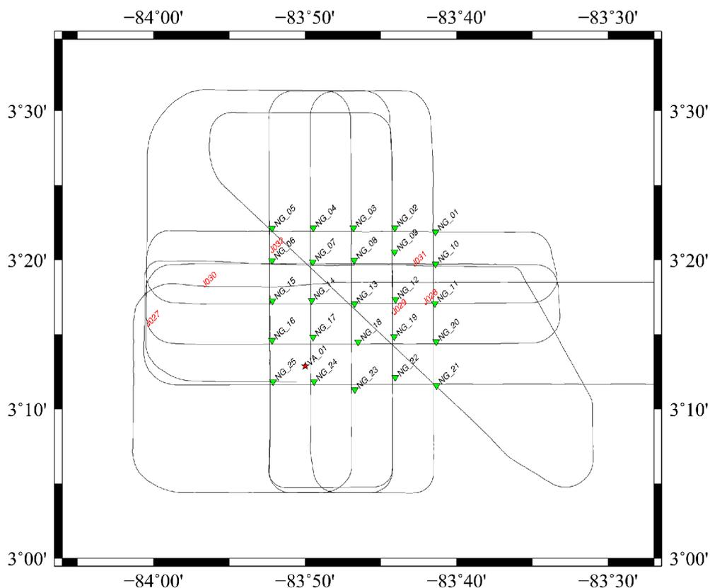
Figure 2.11. OBS (green triangles) and vertical array (VA\_01) (red star) locations in the North Grid area with ship-track of the the recorded airgun sources.
