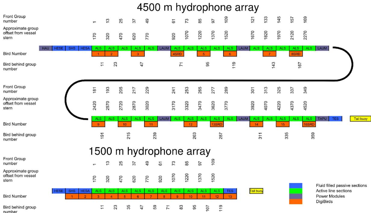
Figure 2.8. Layout of hydrophone array in both the 4500 m and 1500 m configurations. Birds with SRD have emergency buoyancy pods to prevent the streamer going to depths of more than 30 m.
