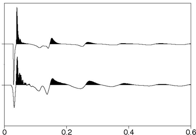
*Figure 2.20. Comparison of predicted (upper) and measured (lower) wave-field for the Bolt seismic source. The shape difference is because the prediction does not include the instrument filter from the OBS logger, otherwise the shape and period of oscillation are well-matched. The predicted signature was calculated using the Nucleus+ software from PGS.*
