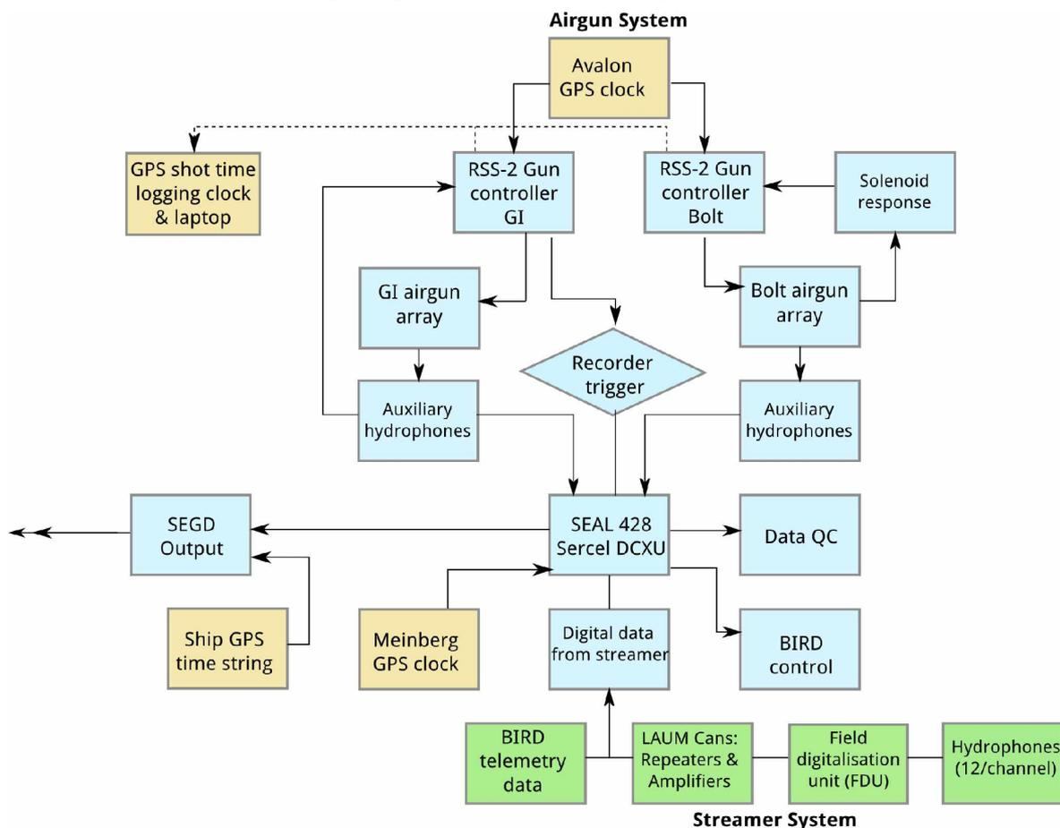
Figure 2.9. Schematic diagram of seismic acquisition system. Although there were two array seismic sources (three when working with the SONNE on the SAP survey) they were all recorded in a single SEG-D file which was then split into the separate records based on the logged shot times, see Figs. 2.2 & 2.3.
