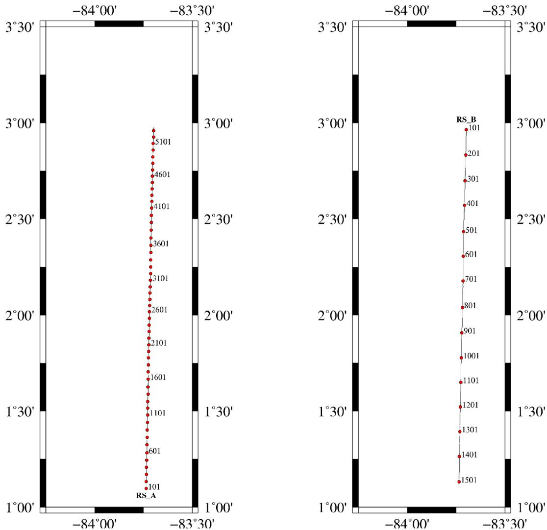
Figure 4.12. Track charts for the multichannel streamer RS profiles. These profiles were shot with a 4500 m streamer. Shot point numbers (FFIDs) are annotated. (a) RS\_A was shot with only the GI source to image the sediment structure over the heatflow measurements from cruise JC113; (b) RS\_B was shot with only the Bolt array as a noise test and for seismic oceanography mapping of the thermohaline structure.
