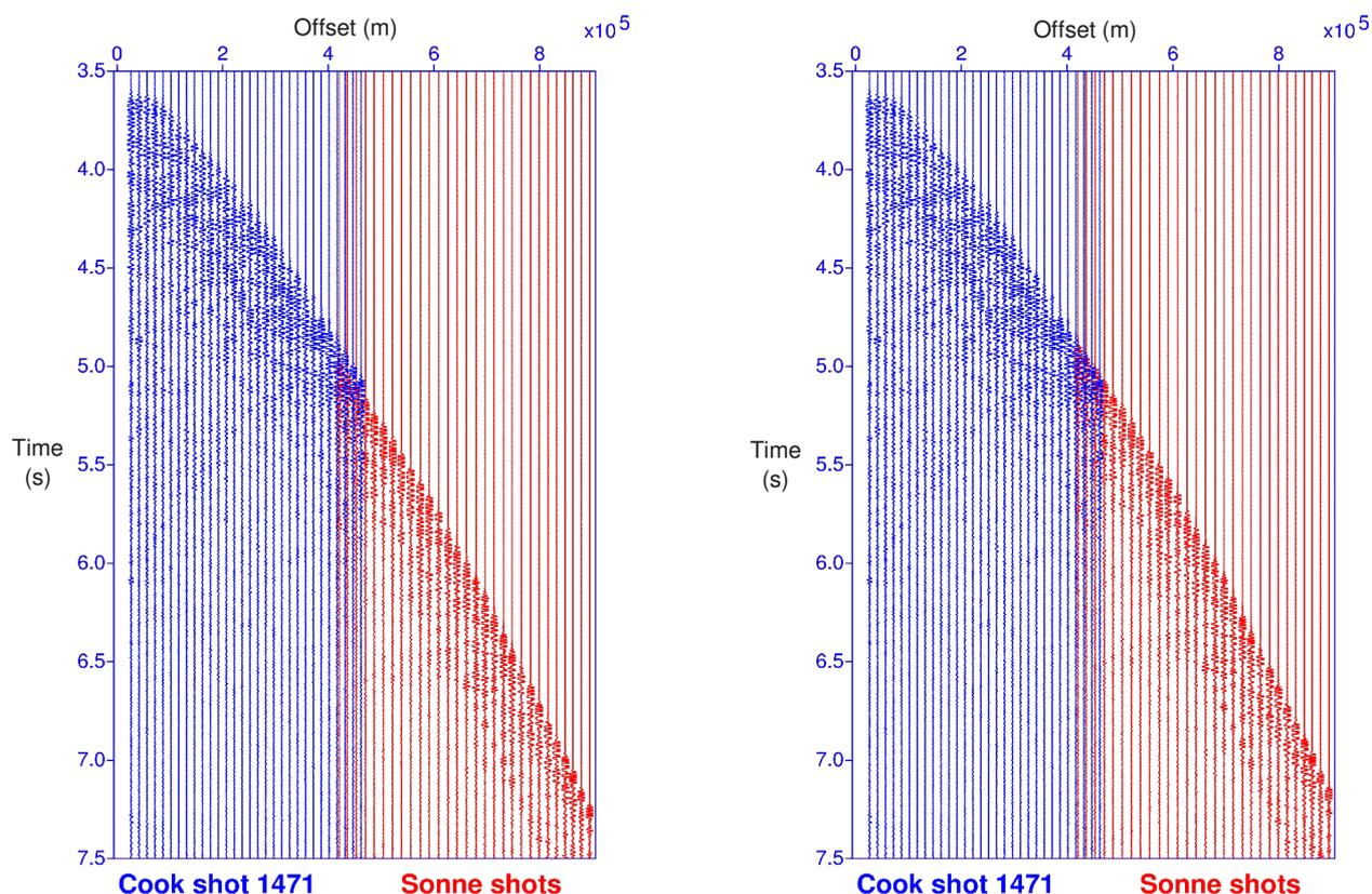
Figure 2.7. Left: merged shots from the COOK (blue) and SONNE (red) before correction. Right: merged shots after correction, note the improved match in the overlap zone between 4.2 and 4.5 km offset. A 300 m overlap between shot recordings from each vessel was purposely designed to verify geometry.
