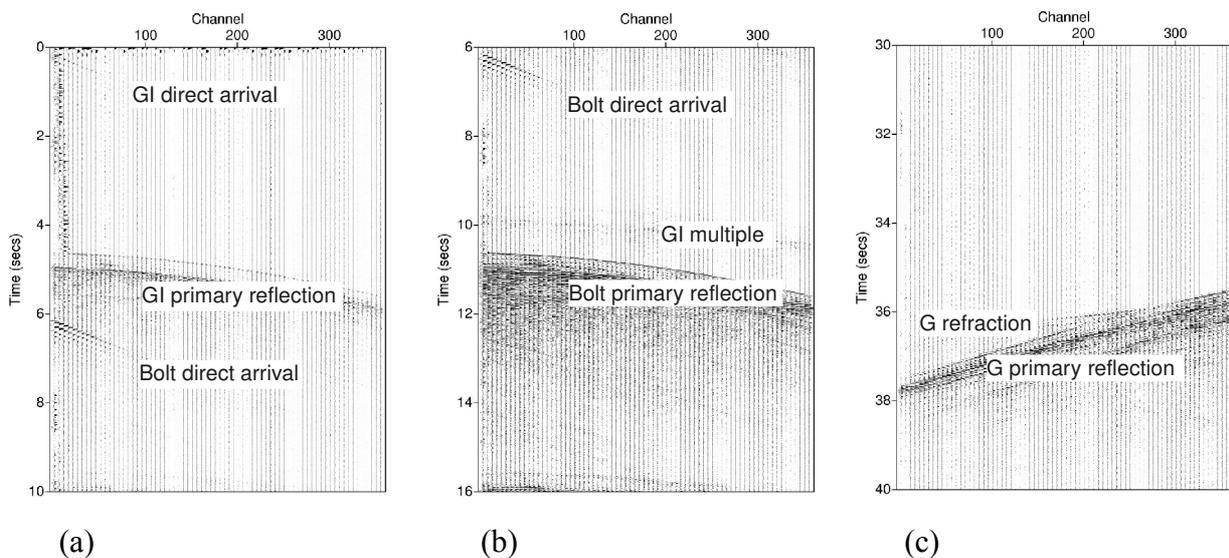
Figure 2.3. Extracted 10 s records for each of shot type: (a) GI shot; (b) Bolt shot; (c) G-gun shot.
