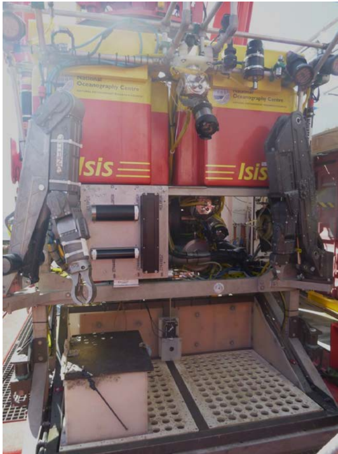
Fig. 3.7. ISIS set-up for forward-looking swath surveys.
