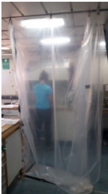
Figure 18.1: Microplastic work carried out by Nina Faure Beaulieu at the laminar flow within the clean tent. The clothing worn is 100% cotton.
