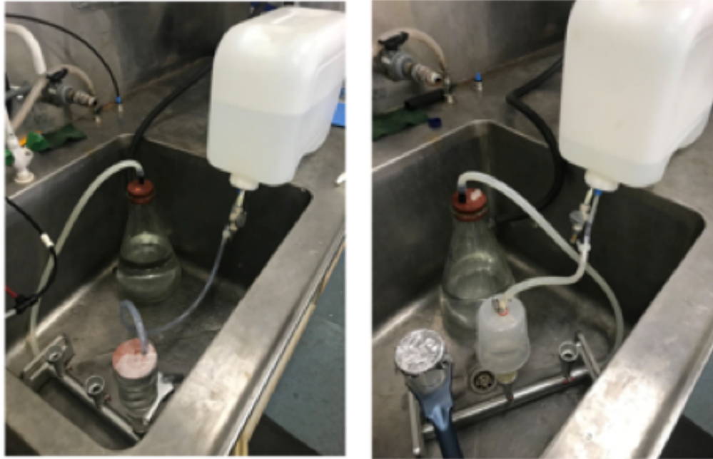
Figure 18.9: 1µm filtration unit with stopper design #1 (left) and #2 (right). A 1µm control is being carried out alongside an actual filtration (right).
