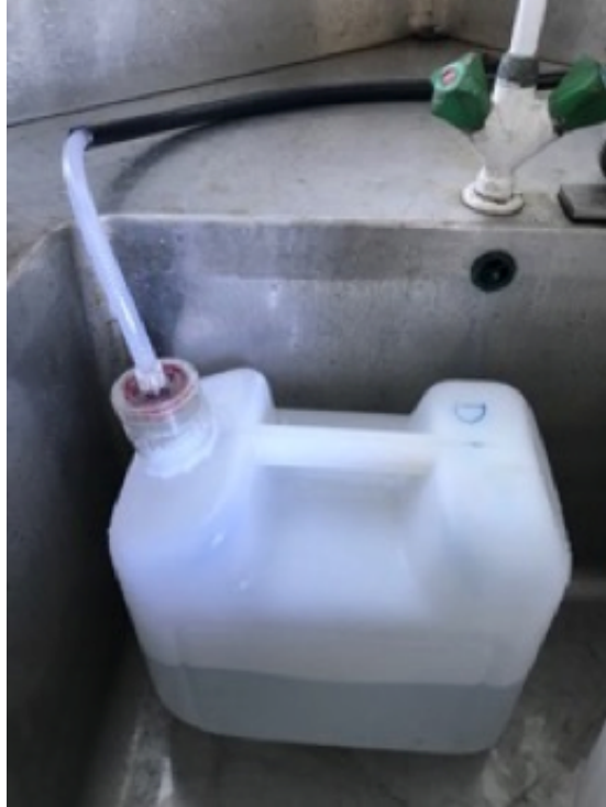
Figure 18.4: Underway sampling using the outflow pipe. The PVC tube slots into the underway pipe
