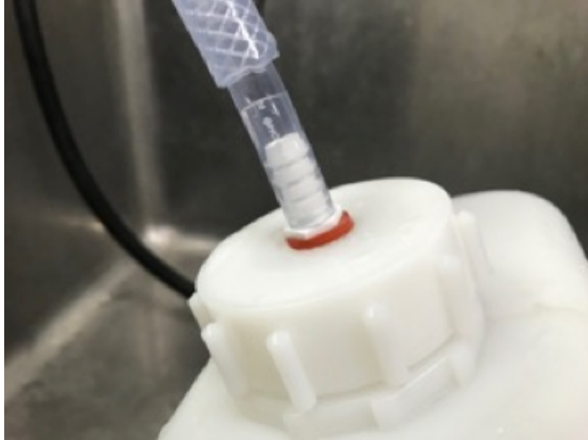
Figure 18.5: Carboy lid modified with a barbed fitting. The PVC tube connects to the barbed fitting and transfers the water without having to open the carboy
