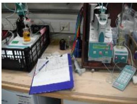
Photo shows the two oxygen analysis systems setup on JC165 (left: Ti-touch, right: Titrino). New Ti-touch dissolved O 2 amperometric end point equipment set up for O 2 analysis on JC165
