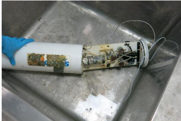
Photo showing the extent of flood damage on the inside of the pH Sensorlab
