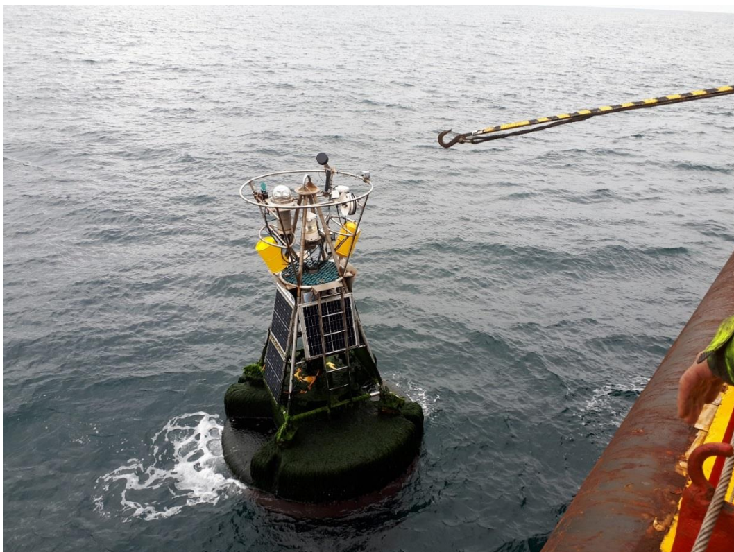
2017 PAP 1 mooring buoy recovery
