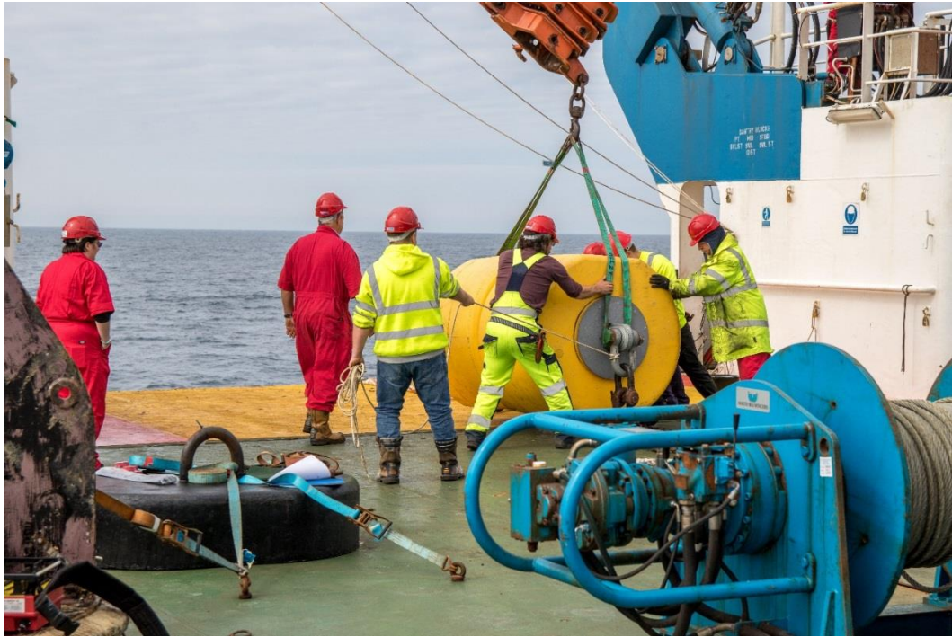
PAP 1 subsurface float (anchor weight in foreground)
