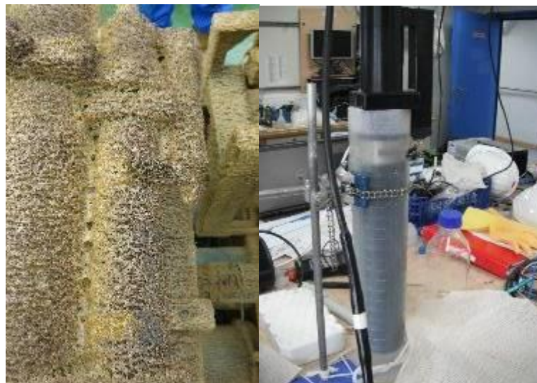
SUNA post deployment under heavy fouling, and the unit cleaned and set up for calibration
