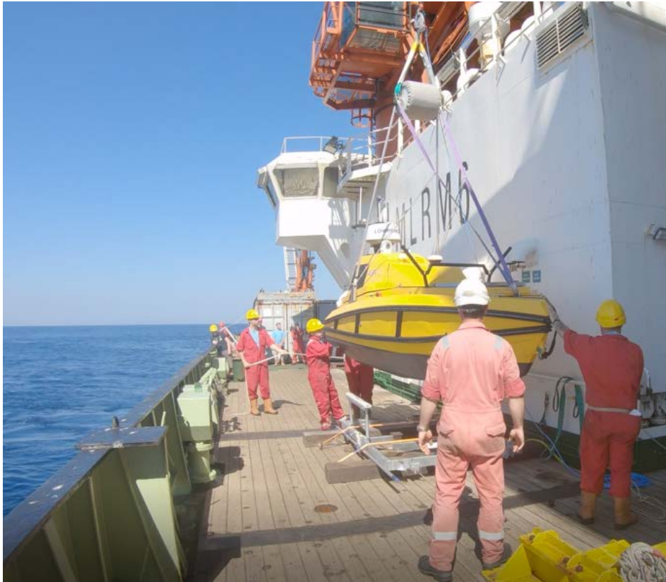
Fig. 6.1 C-Worker 4 with its custom lifting bridle, and the CAMEL transport trolley strapped to the deck
