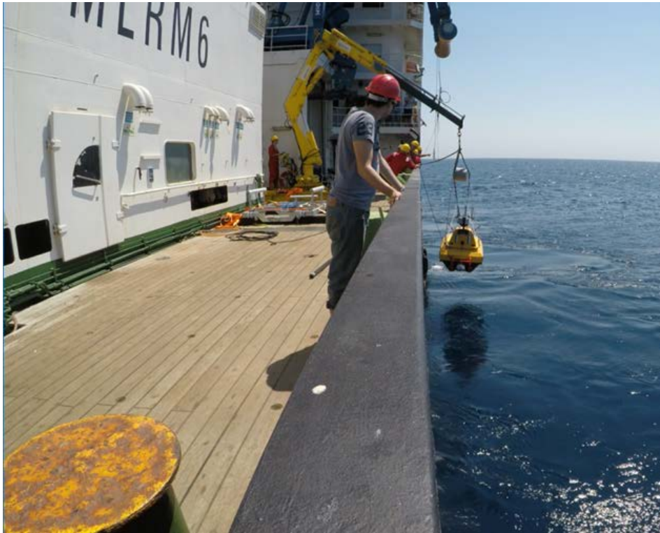
Fig. 6.5 C-Worker 4 recovery. Just after the transfer from the P-Frame to the Yellow HIAB
