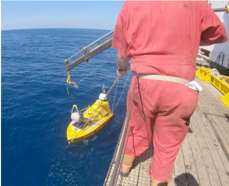
Fig. 6.4 C-Worker 4 Launch. Tag lines still attached.
