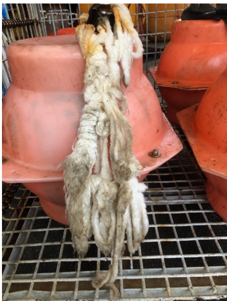
Figure 16.2 The recovered end of the 16mm diameter 3-strand nylon twist rope that parted above the acoustic releases.
