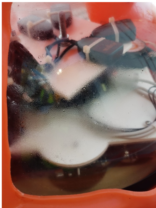
Figure 17.2 Photo of condensation inside the PIES buoy controller.
