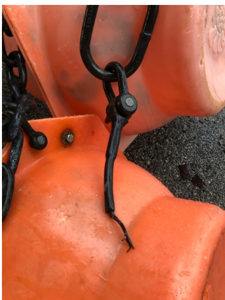
Figure 16.3 The parted 3/16" outer diameter jacketed wire rope (3x19 construction). The wire parted near the termination attached to the glass buoyancy.
