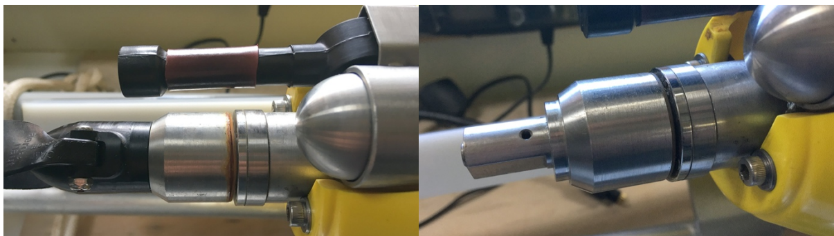
Figure 32. Thruster assembly on glider 405 before (left) and after (right) cleaning and lubrication.
