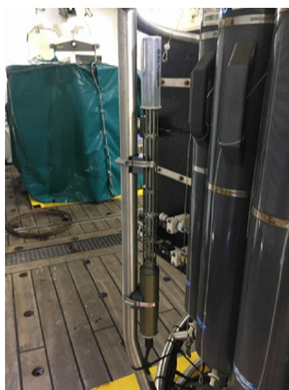
Figure 42. Seabird SBE 35 DOST mounting location overview – same as DY113.
