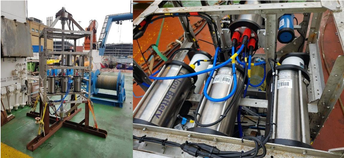
Three SubCTech batteries mounted in a row on the sensor frame
