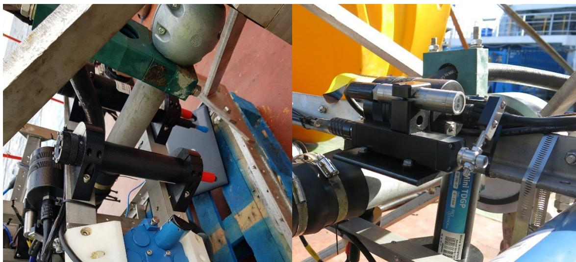
Photo showing the mini TDGP on the frame, right photo shows the Seaguards fluorometer (and Zebratech wiper)
