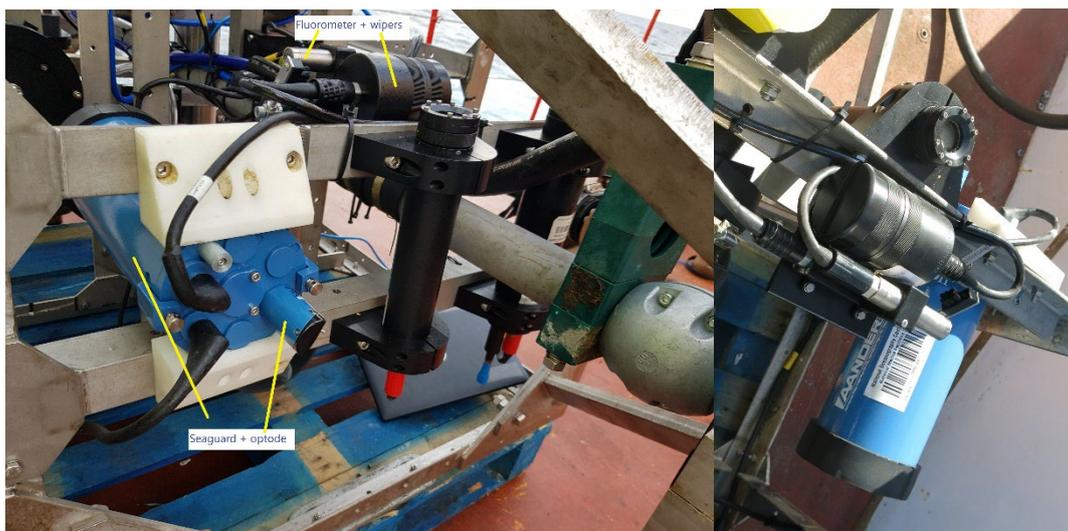
Seaguard is mounted on the top level of frame, with the fluorometer (and the Zebratech wiper) next to it
