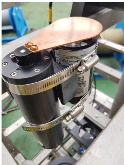
The bio-shutter on the frame stopped working on the day before deployment, despite working non-stop throughout the extensive bench test. As a result, the copper shield was removed prior to the buoy being deployed which will affect the length or quality of the data receive in the long term.
