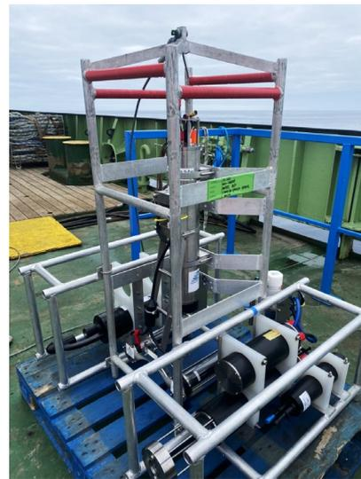
Left: Red Camera Frame set up. UVP5 and RBR Concerto in the middle, LISST HOLO2 on the left hand side, ECOTRIplet and CPICS are on the right hand side. Right: Deck unit setup in deck lab.
