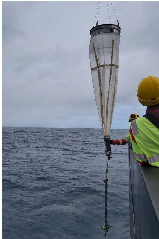
*200 µm mesh WP2 midday net being deployed from the rear starboard side of the ship (07/05/2022).*
