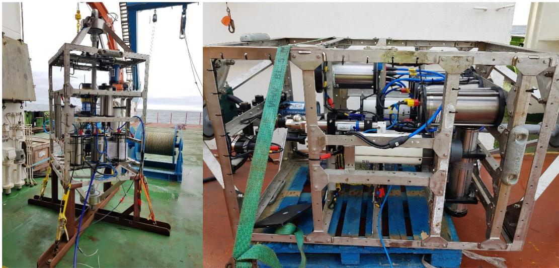
PAP1 deployed sensor frame
