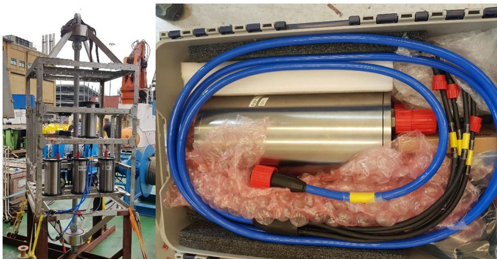
Frame controller mounted on the frame and inside the transportation box with cables
