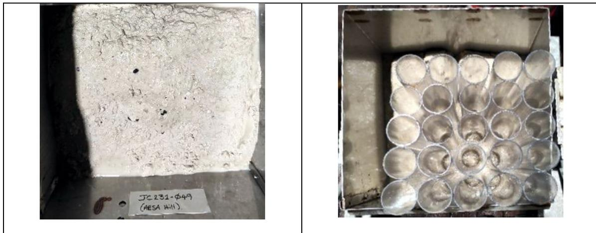
*Example box core surface (left) and 5 × 5 subsampling grid of core liners (right).*
