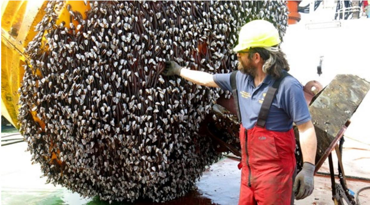
As usual the sensor frame exhibited far less fouling than the buoy and less than has been seen on some of the previous deployments:
