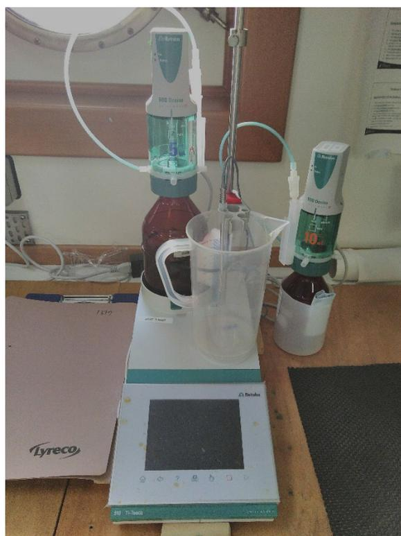
The Metrohm Ti-touch 916 setup used for dissolved oxygen analysis.
