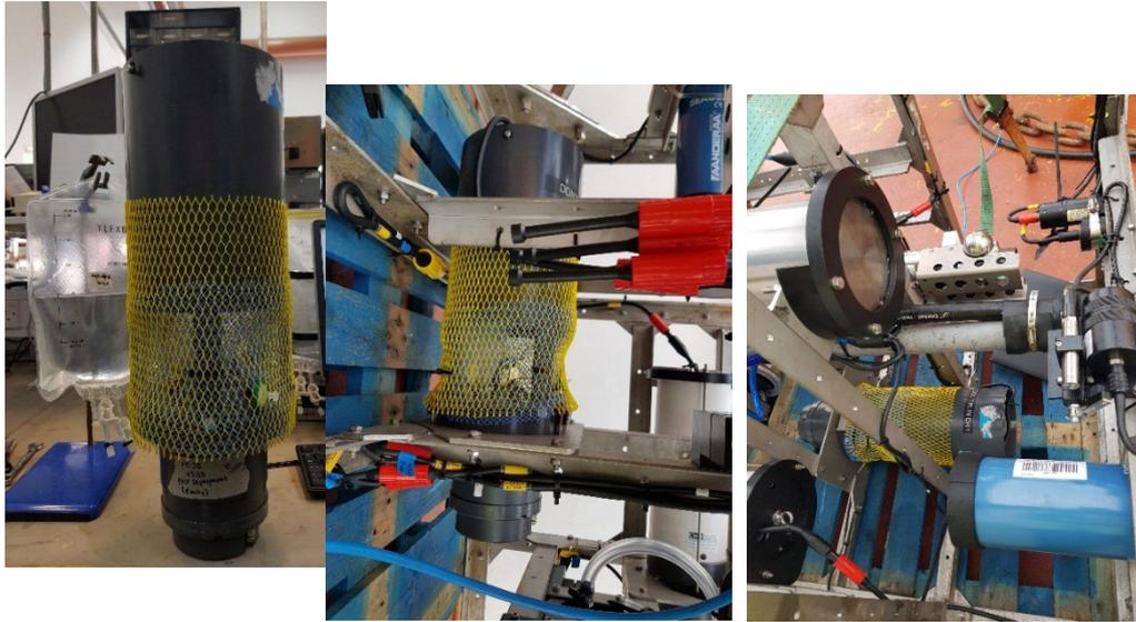
OTE pH sensor - on the bench and fitted on the sensor frame
