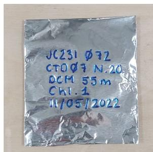
*Aluminium foil pouch example for HPLC and DCM chlorophyll samples.*
