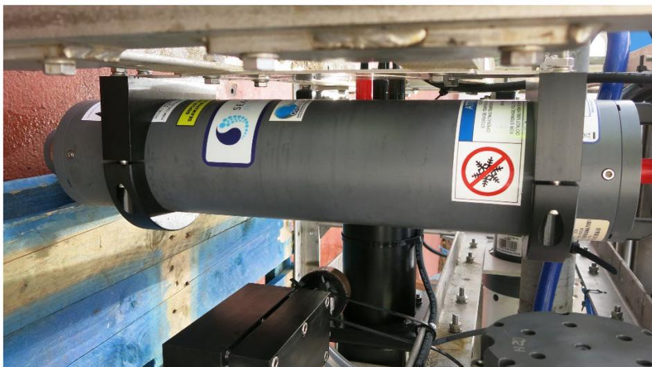
The SeaFET v2 pH sensor has internal batteries for backup and powered through the frame hub. It was configured at NOC to run every 30min.
