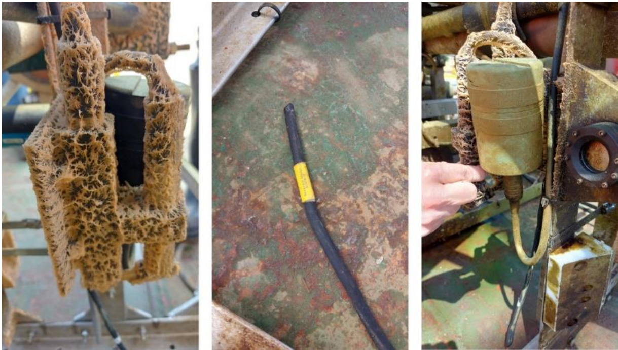
Turner fluorometer + optode – SN: 2410
