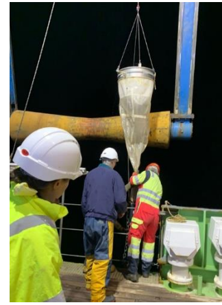
Deployment of the 200 \mu\text{m} mesh WP2 night net from the P frame on the rear starboard side of the ship (Station: 025 - 11/05/23).
