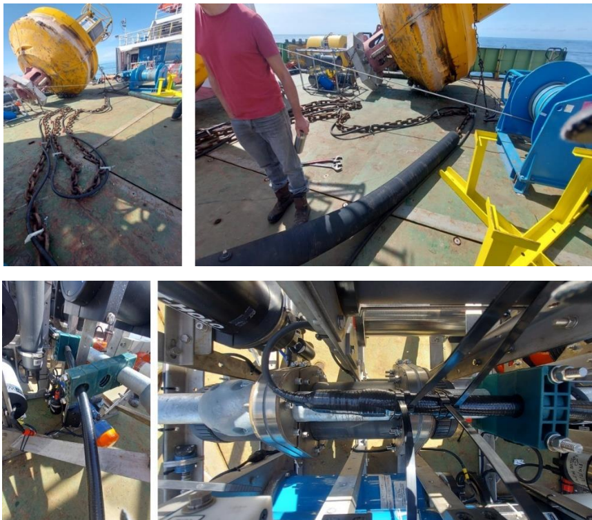
Photos show the umbilical and chain laid out on deck the morning of the deployment, with the green bracket, tubing (with black tape covering) inside the frame
