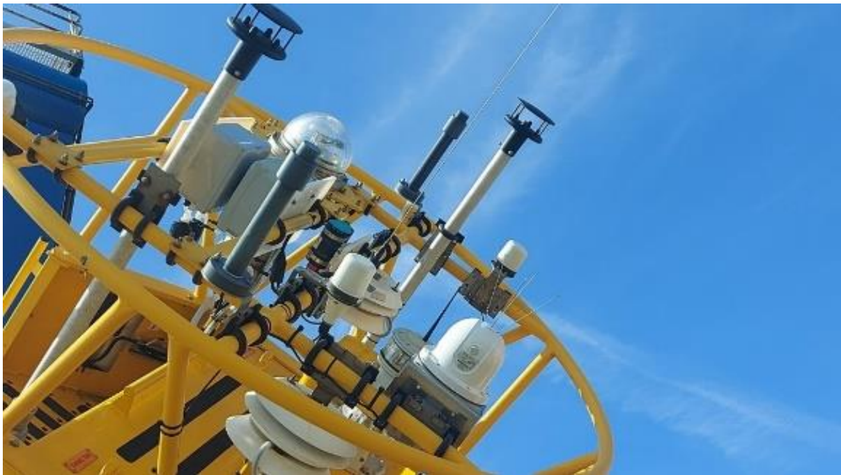
Photo of Met Office sensors, tracker, OCR and 2 Pro-CO2 atmospheric gas inlet boxes.
