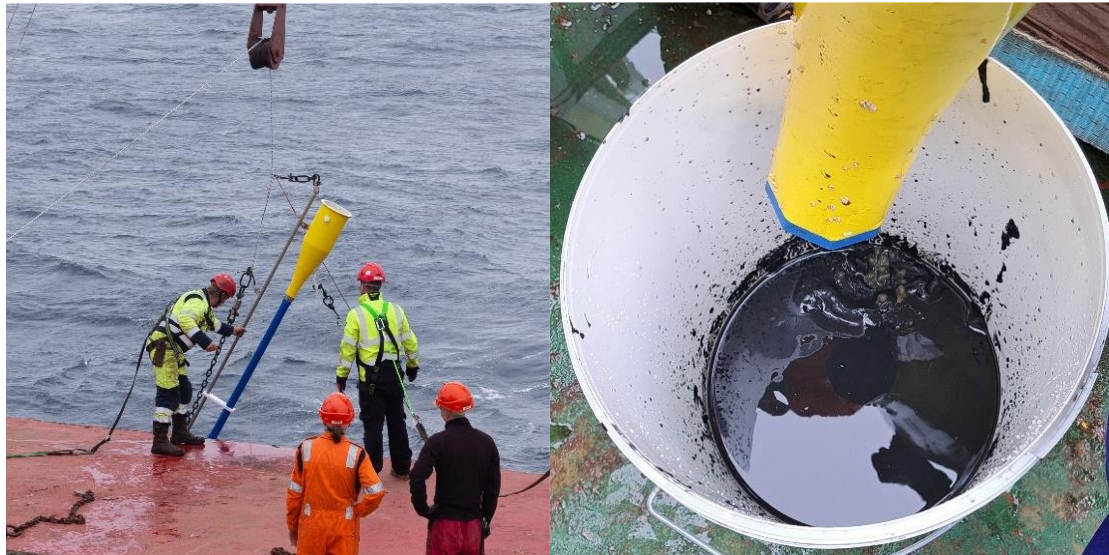
Recovery of the Anderson trap to deck and appearance of sediment that spilled from the trap during processing.
