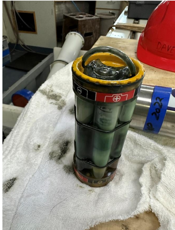
Flooded SBE 37 ODO SN: 23950 Battery Pack.
