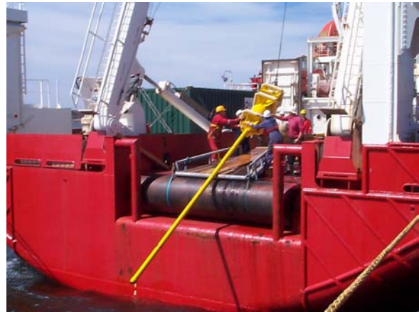
Fig. 15. View from FIPASS of the 6 m corer being recovered.
