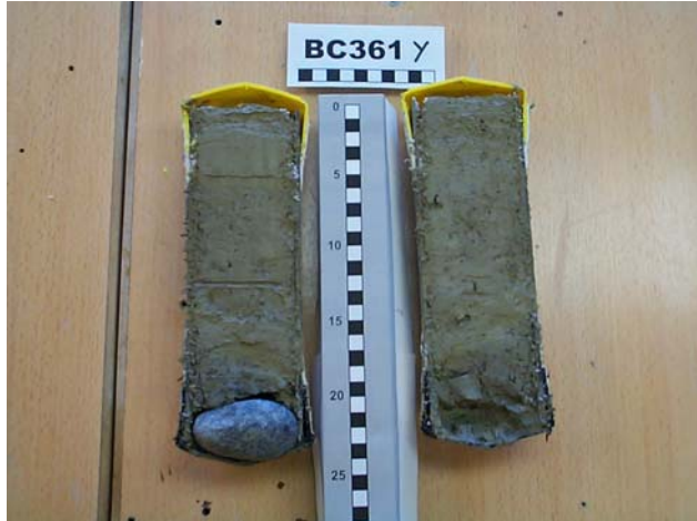
Fig. 8: Photo of split subcore Y of box corer BC361. Sediments: 0-17 cm: brown olive, bioturbated diatomaceous mud; 17-23 cm: grey, massive diamict. Note the rounded cobble (gabbro) at the base of the subcore.
