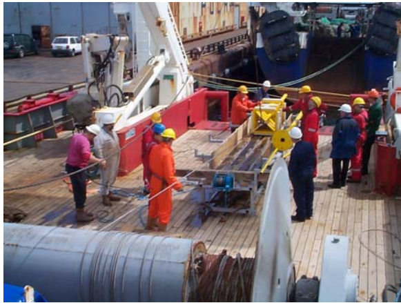
Fig. 14. Pennant on the trawl winch used to haul in the corer.
