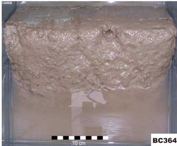
Fig. 17: Photo of box core BC364. Surface sediment: muddy diatomaceous ooze. Note the tilting of the recovered sediment package
