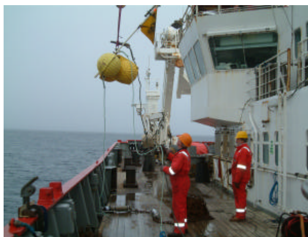
“Acoustic modem trial” mooring being deployed.
