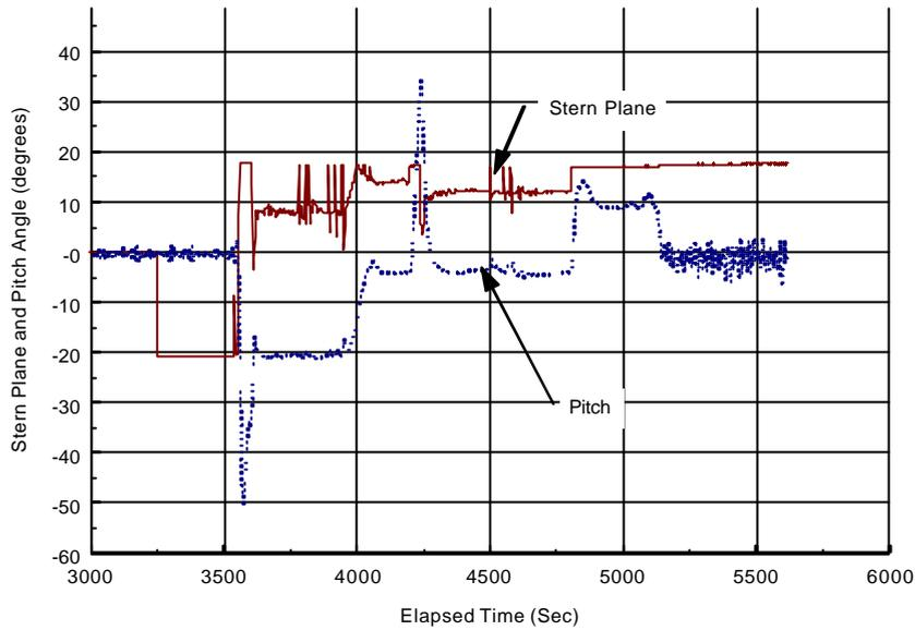
Figure 2.6. The time period from 4300 to 4700 seconds show the time of level, steady flight, the stern plane angle of 12 degrees is close to its full travel (17 degrees).
