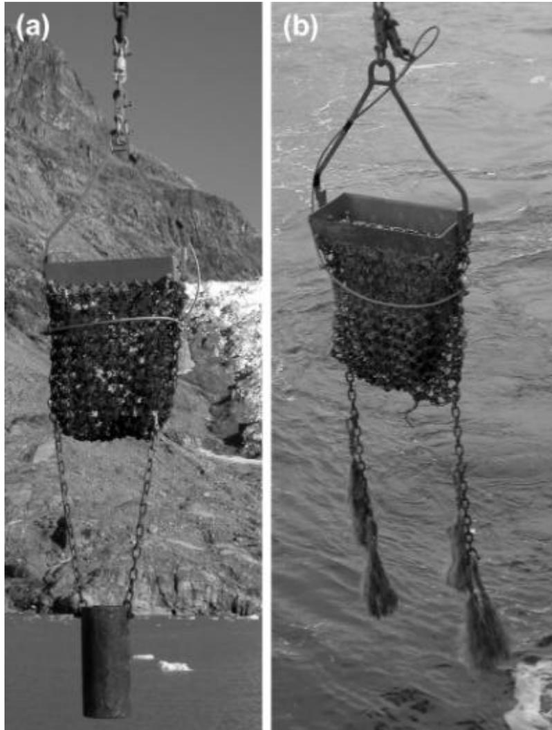
*The UK National Marine Equipment Pool (SOC) rock dredge as used during RRS James Clark Ross cruise 106-south: (a) conventionally rigged with dredge bucket, (b) dredge bucket replaced with hemp tangles.*
