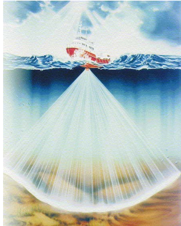
Figure 6.1: Schematic of the multi-beam echosounder system (Modified from the Simrad operator manual).
