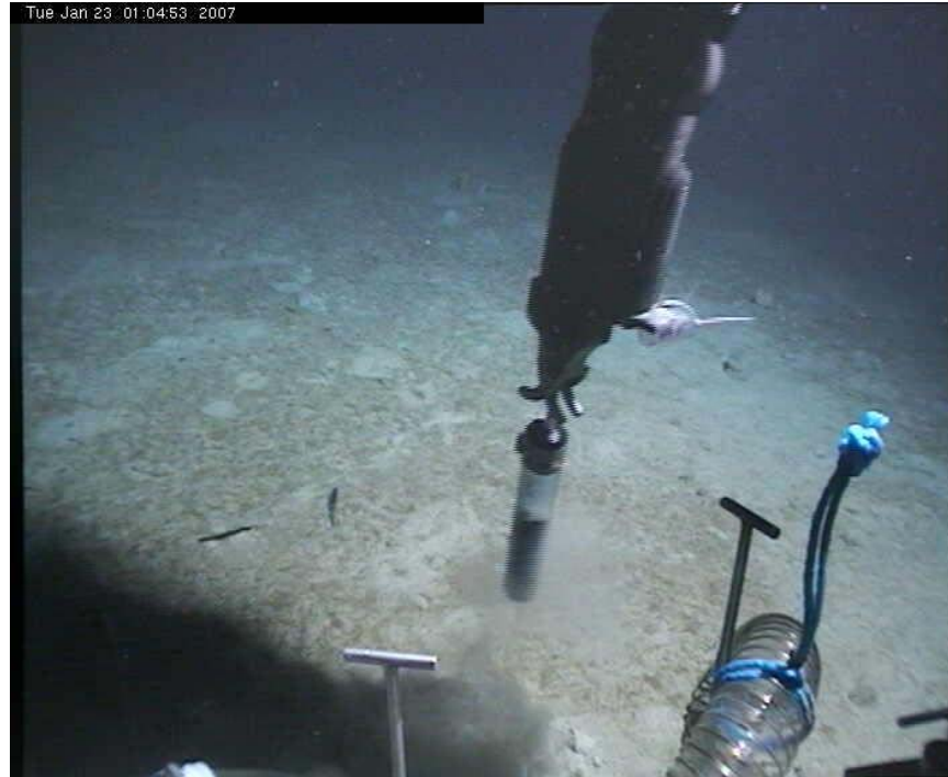
Figure 4.3. Push core being taken of the sea floor using the manipulator arm of Isis
