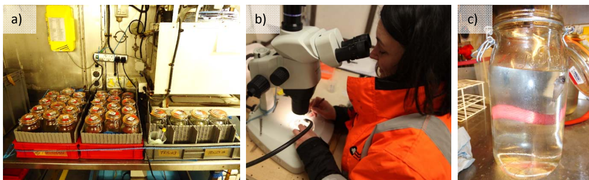
Figure 46 a) Density bottle method set up in JCR cold room (temperature set to 4°C). Each jar contains a sea water glycerol mix, 27 solutions cover S.G. range of 1.0250 to 1.0900 in 0.0025 increments, plus one jar of original filtered sea water. b) Fish were dissected to remove gas from swim bladder. c) Fish were suspended in solutions until they either demonstrated neutral buoyancy or the mean was taken of the last solution the fish sank and the first it floated in.
