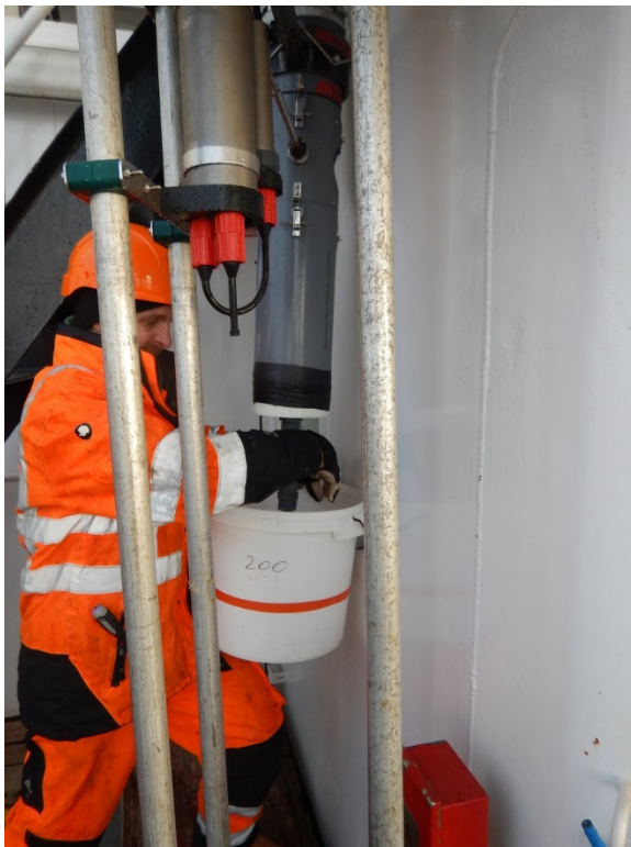
Figure 38 Collecting water from upward looking cod end through tap
