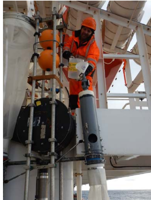
Figure 33 Filling of the downward looking cod end prior to deployment
