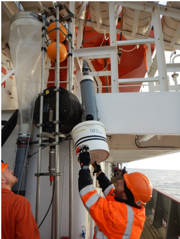
Figure 36 Collecting water from the downward looking cod end on the manual triggering of the motor
