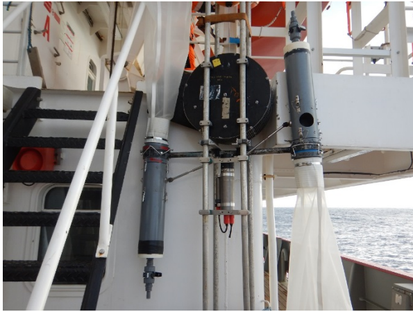
Figure 32 MUDL net showing the cod ends, motor device and arms and motion compensation mechanism
