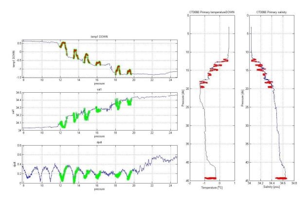
**Figure 7:** Multiple warm anomalies on CTD cast 66 associated with a decrease in the decent rate of the CTD package and old water being flushed past the sensors. Anomalies manually identified (in red/green) were removed.
