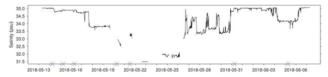
Fig. 9. Salinity data with underway cleaning times indicated by crosses.
