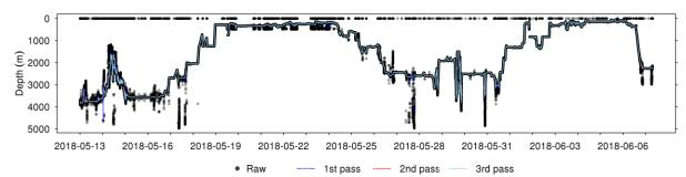
Fig. 1. Raw and filtered EA600 echo-sounder data.
