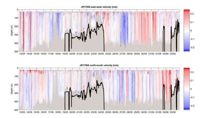
**Figure 2.** East-West and North-South velocities between 13<sup>th</sup> May 2018 and 3<sup>rd</sup> June 2018 (water tracking, 16 m bins). Black line is bathymetry extracted from the EA600.
