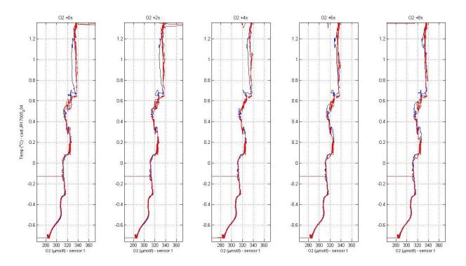
**Figure 4.** Temperature vs. oxygen concentration for a 0, 2, 4, 6 and 8 second alignment (left to right) of cast 004 (full profile shown). Water temperature ranges between -0.7 and 1.4°C and the alignment is improved with a greater advance (8 seconds producing the best agreement between up and down casts).
