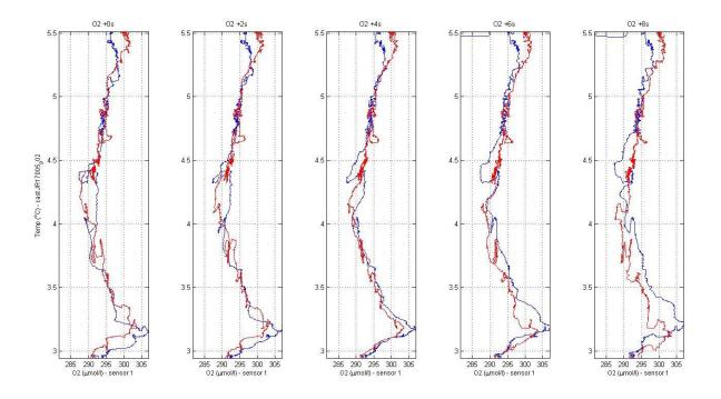
**Figure 3.** Temperature vs. oxygen concentration for a 0, 2, 4, 6 and 8 second alignment (left to right) of cast 002 in  $3-5.5^{\circ}$ C temperature water. Blue = downcast. Red = upcast. A 4 second alignment looks optimal here.
