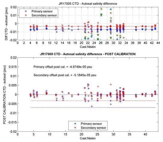
**Figure 9. Top.** CTD minus Autosal differences for the primary and secondary sensors. Points in green are > 0.2 standard deviations from the median and were discarded. Red and blue lines are the median offsets once outliers in green were removed. **Bottom.** CTD minus Autosal salinity differences once the offsets (dashed red and blue horizontal lines) had been applied.
