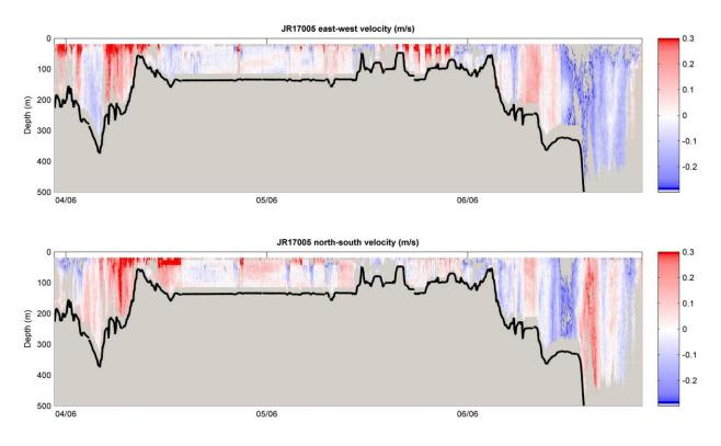
**Figure 3.** East-West and North-South velocities between 4<sup>th</sup> and 7<sup>th</sup> June (bottom tracking, 8 m bins). South of Svalbard and in Storfjorden.
