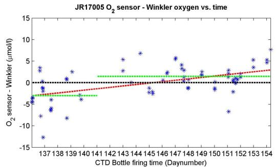
**Figure 11.** CTD sensor – winkler sample offset vs. time AFTER correction for the depth dependent offset. Red line = linear trend. Green lines = pre- and post May  $21^{st}$  average offsets. Black line = mean (zero) offset.
