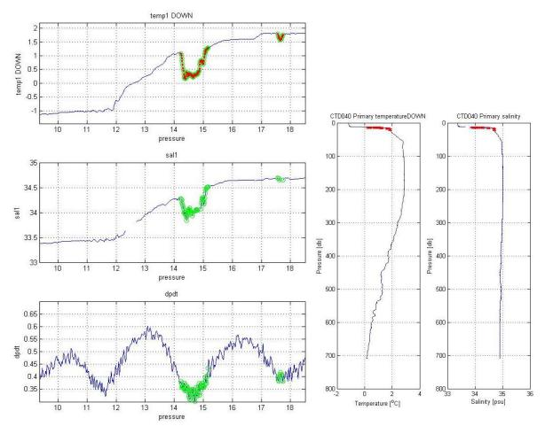
**Figure 6:** Example of a broad (1 m) spike in the temperature and salinity associated with a decrease in the decent rate of the CTD package as it passes through a sharp gradient in temperature (3°C increase over 6 metres) and salinity. As the CTD package slows colder (and fresher) water from above is pushed back past the sensors again. The section between 14 and 15 db was identified manually and removed from the profile.
