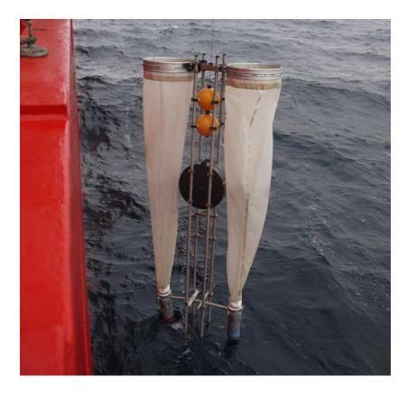
Fig 2: Deployment of Bongo net
