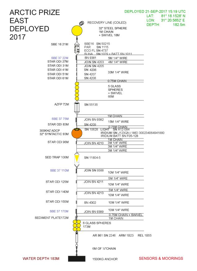
Figure 2.23: EAST mooring diagram deployed in 2017 and recovered during this cruise. Note: instrument depths on diagram are approximate.
