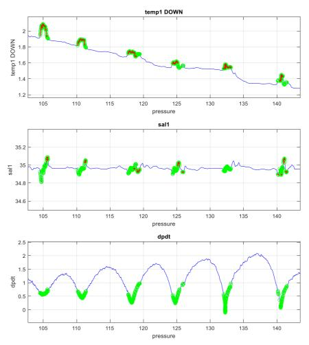
Figure 2.3: Example of flagged temperature anomalies from water recirculating within CTD package as veer rate changes.
