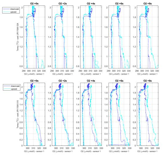
Figure 2.1: Oxygen measurements plotted against temperature to track water mass space rather than depth. Upcast and downcast data with advances from 0 to 8 seconds.
