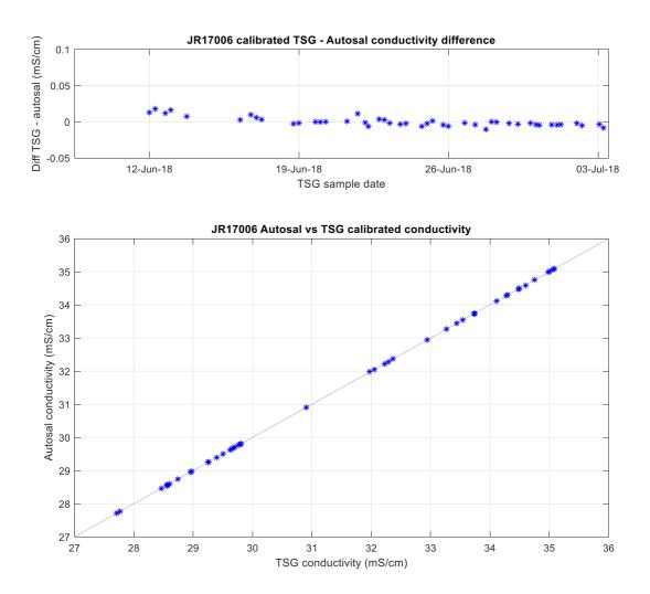
Figure 2.14: (Top) difference between the corrected TSG and Autosal conductivity readings in time. (Bottom) corrected TSG vs Autosal conductivity readings.
