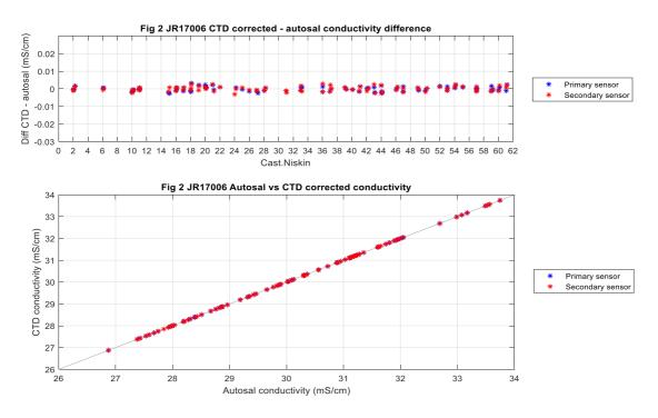
Figure 2.6: Top: difference between the corrected CTD and Autosal conductivity readings in time. Bottom: corrected CTD vs Autosal conductivity readings.
