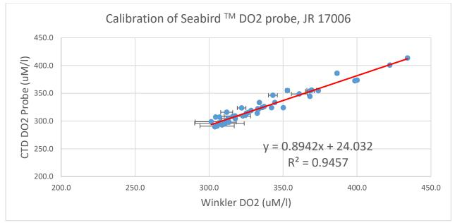
Figure 4.1: Calibration of Seabird oxygen probe
