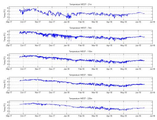
Figure 2.29: WEST mooring temperature timeseries, Sep-17 to Jun-18 at 21m, 74m, 110m, 160m and 220m.
