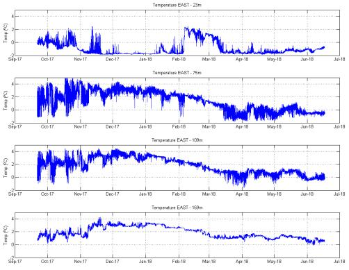
Figure 2.27: EAST mooring temperature time series, Sep-17 to Jun-18 at 23m, 75m, 109m and 169m.
