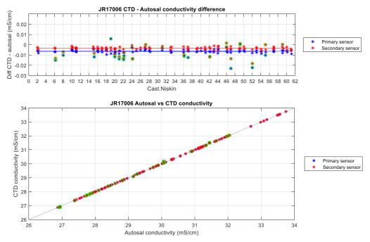
Figure 2.5: Top: difference between the raw CTD and Autosal conductivity readings in time, close-up. Bottom: raw CTD vs Autosal conductivity readings. Green circles indicate outliers, removed from dataset before calculating the final sensor offsets. The offsets are the lines shown on the top plot.
