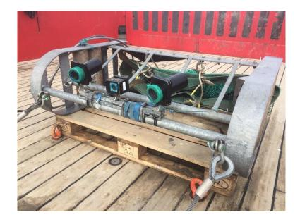
Figure 9.1: Agassiz trawl and camera system rigged prior to deployment from JCR.
