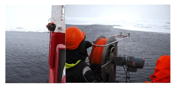
Figure 2.18 - the line being payed out over the stern of the ship (left) and reeled in using the boom on the winch to guide the line onto the drum equally
