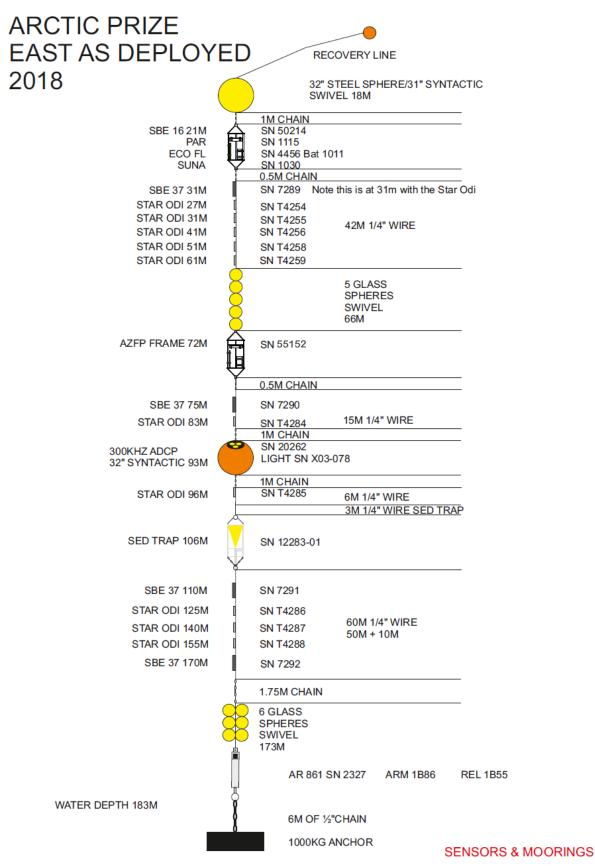
Figure 2.34: EAST mooring diagram, deployed on 20-Jun-18.
