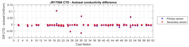
Figure 2.4: Difference between the raw CTD and Autosal conductivity readings in time, all values.
