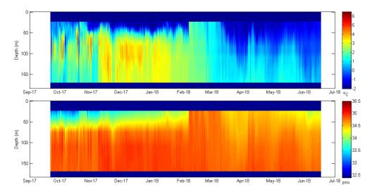
Figure 2.24: EAST mooring CTD contour time series, Sep-17 to Jun-18. Temperature data is from the SBE37s and Star-Odis, salinity from the SBE37s.
