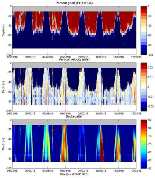
Figure 2.33: example of ADCP backscatter (middle) and vertical velocity (bottom) data over one week on the West mooring. The top plot shows the data quality percentage (sum of PG1 = 3-beams solution and PG4=4-beams solution). Data where the PG sum is less than 50% have been masked in the bottom plots (dark blue).
