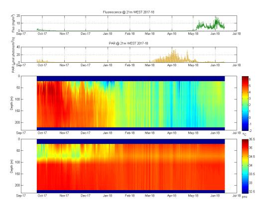
Figure 2.25: WEST mooring CTD contour time series with Chl-a fluorescence and PAR, Sep-17 to Jun-18. Temperature data are from the SBE16, SBE37s and Star-Odis, salinity from the SBE16 and SBE37s. An offset in conductivity is suspected on the ~75m SBE37.
