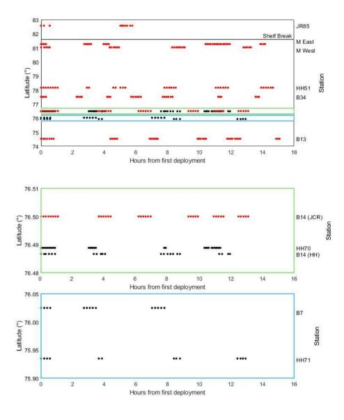
Figure 2.16 - Stations where MSS profiling was completed during JR17006 in red. Stations visited on the previous Arctic PRIZE cruise (HH23042018) are shown in black, Station B14 was visited during both cruises. Note extra contour at 250m.
