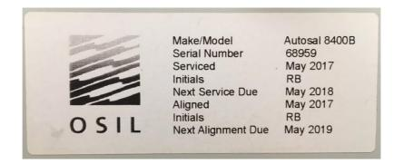
Salinity samples were collected by the science team and stored in the corridor lab with the BAS Guildline Autosal Sn 68959. The room temperature was controlled to approximately 23 degrees C and the bath temperature was set to 24 degrees C. The temperature of the lab was observed to fluctuate between approximately 22.8 – 23.9 degrees C.
