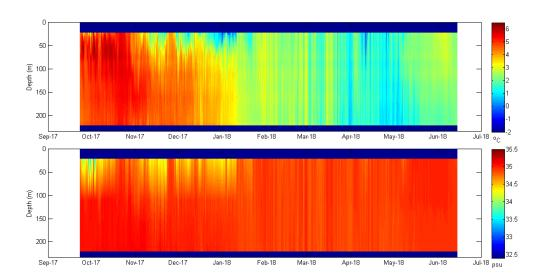
Figure 2.26: WEST mooring CTD contour timeseries, Sep-17 to Jun-18. Temperature data are from the SBE16, SBE37s and Star-Odis, salinity from the SBE16 and SBE37s. Salinity data from 75m SBE37 excluded.
