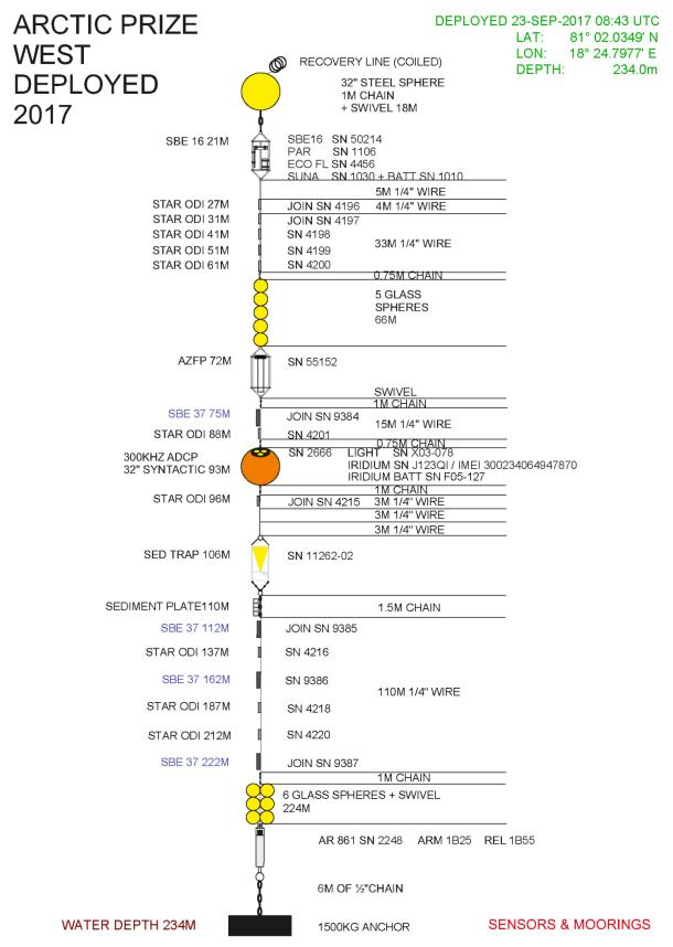
Figure 2.22: WEST mooring diagram deployed in 2017 and recovered during this cruise. Note: instrument depths on diagram are approximate.
