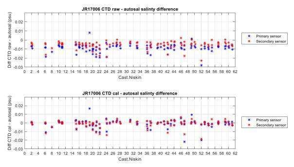
Figure 2.7: Top: difference between the raw CTD and Autosal salinity sample readings. Bottom: re-calculated CTD vs Autosal salinity sample readings using the corrected conductivities.
