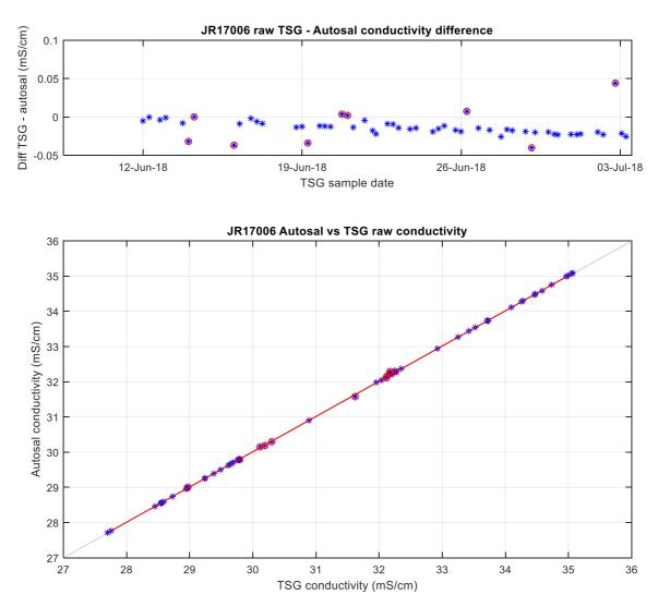
Figure 2.13: (Top) difference between the raw TSG and Autosal conductivity readings in time. (Bottom) raw TSG vs Autosal conductivity readings. Outliers indicated by red circles.
