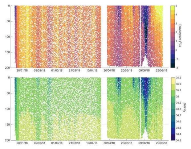
Figure 2.20: Raw temperature and salinity time series from January to July 2018, from the surface down to 200m.
