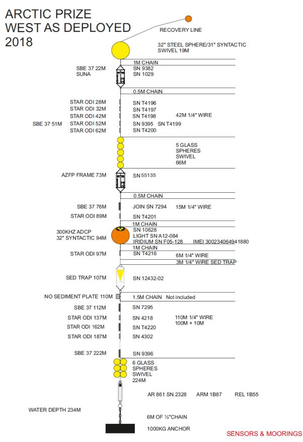
Figure 2.35: WEST mooring diagram, deployed on 22-Jun-18.
