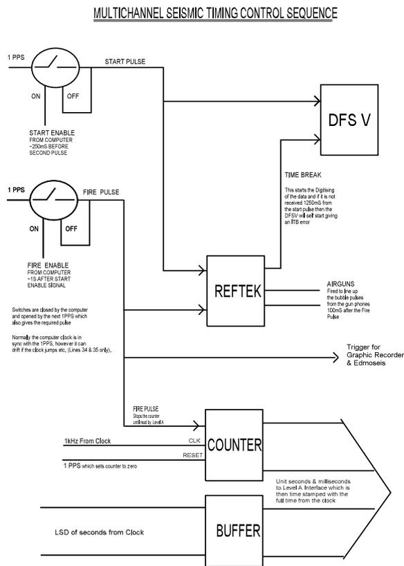
Fig. ZZ. Multichannel seismic system timing control sequence.
