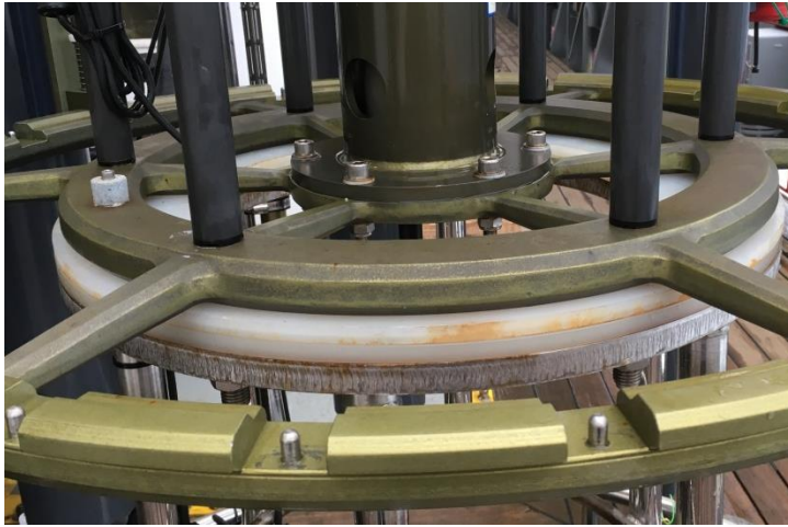
Figure 16:- Installation of additional CTD isolation washer
