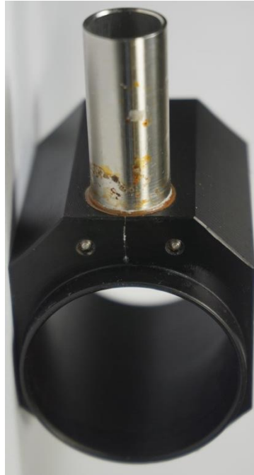
Figure 13:- Transmissometer end bracket hairline crack
