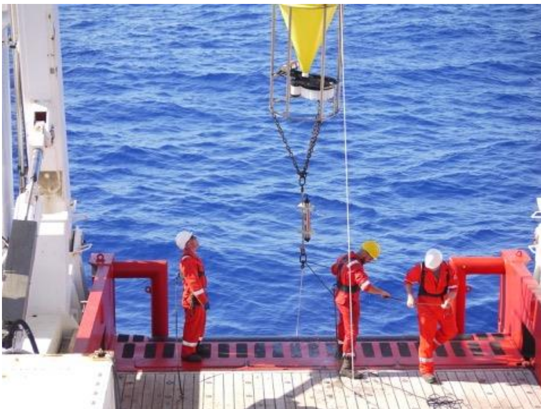
Figure 3: Sediment Trap Recovery.
