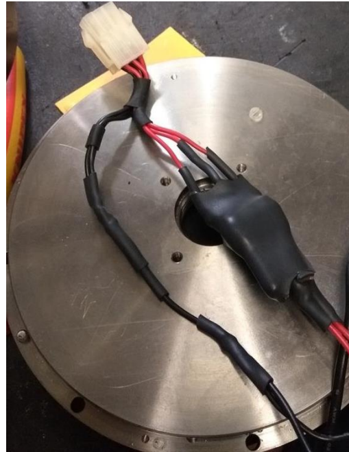
Figure 21:- Chelsea Battery Pack S/N 182042 Replacement charging components
