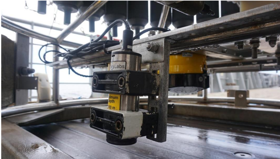
Figure 18:- Seabird Eco-FLBB installation
