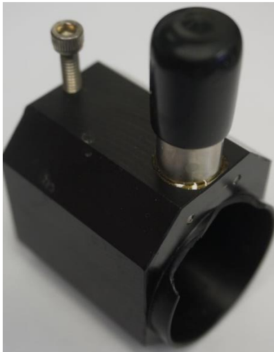
Figure 14:- Transmissometer bracket damaged end
