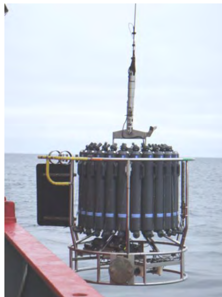
Figure 1.1-1: CTD being deployed from the mid-ship gantry.
