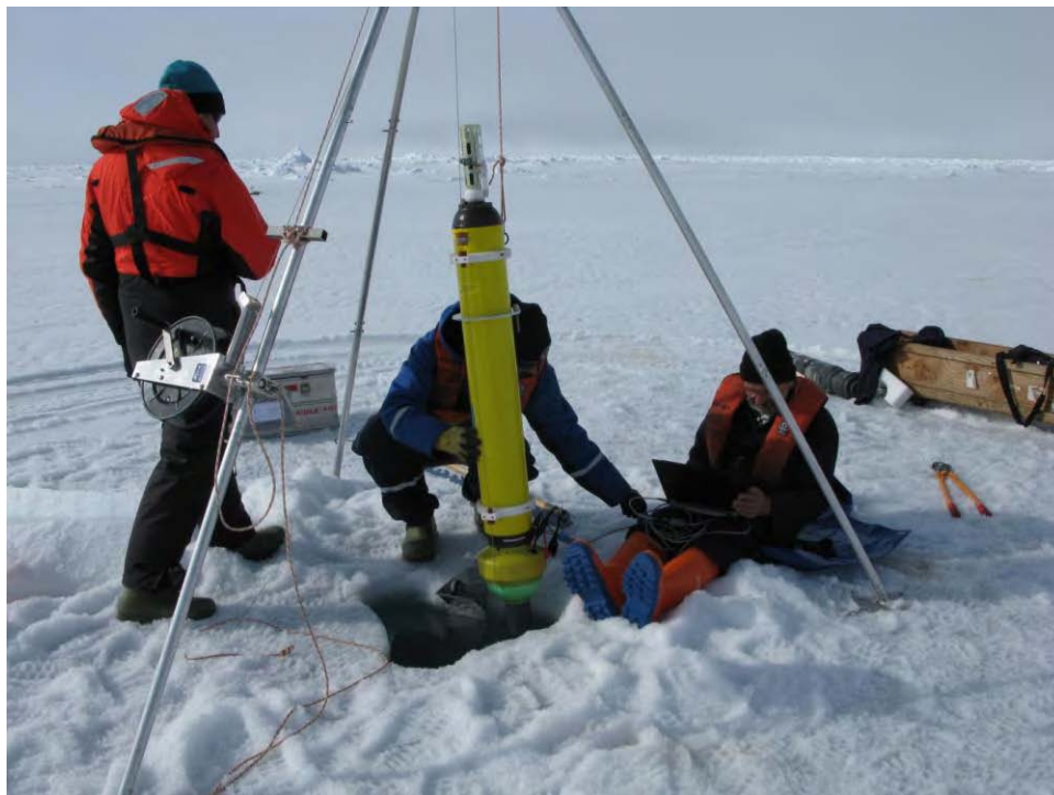
Figure 2.14. APEX buoy in preparation for deployment through the ice. The float is constrained to profile along the weighted line suspended from the tripod and passing through the line guides mounted to the outside of the hull.
