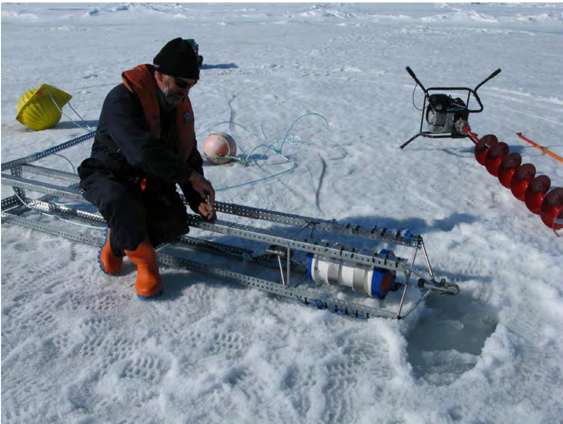
Figure 2.6. ADCP & frame following recovery
