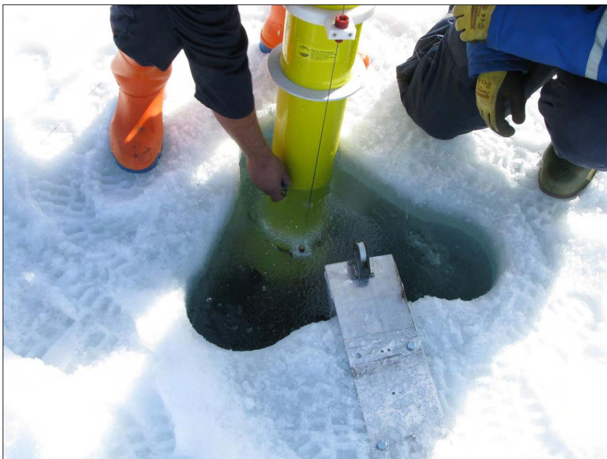
Figure 2.15. Deployment of the APEX float through the sea ice
