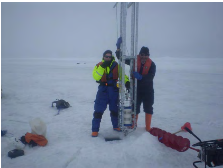
Figure 2.4. ADCP prior to deployment
