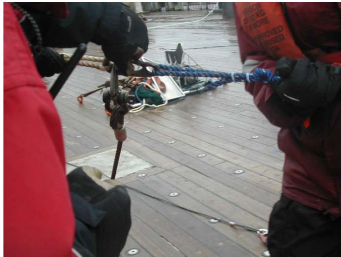
Figure 8 - Attaching the Gilson winch wire to the lazy deck
