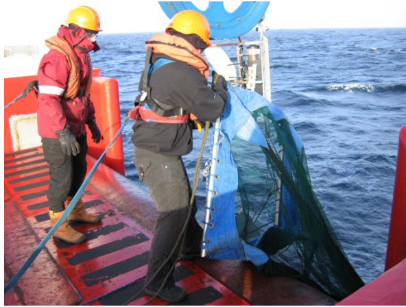
Figure 5 - Deployment of the net, Depressor just deployed
