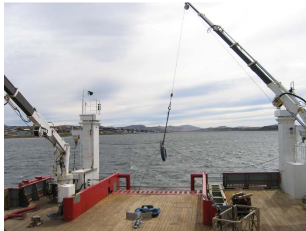
Figure 1 - Putting the block into place using the Effer crane
