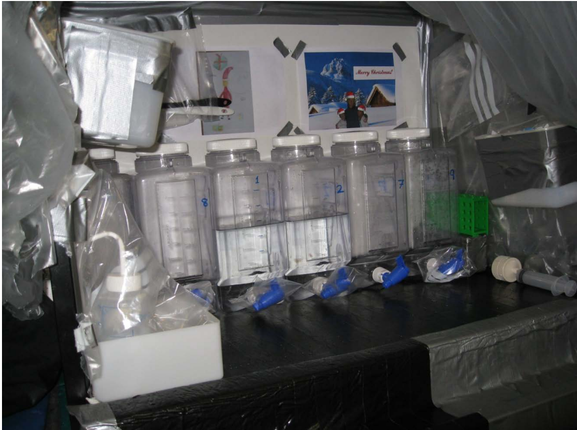
Figure 22 - Interior of laminar flow cabinet showing 9L experimental carboys used for krill iron excretion experiments. Despite being sited in a draughty cold room, the plastic tent covering the working area (removed here) precluded contamination
