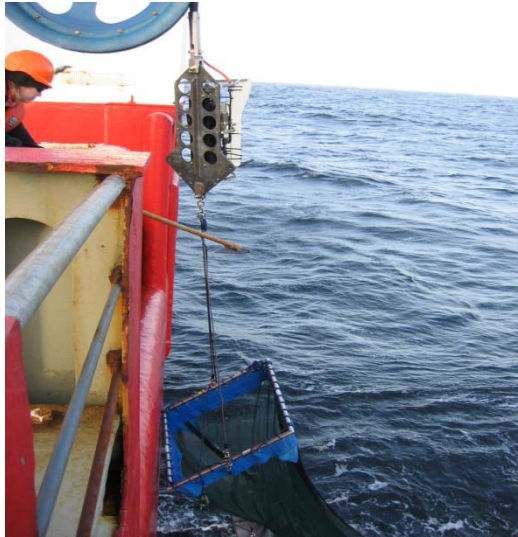
Figure 7 - Using the hook to get hold of the lazy deck
