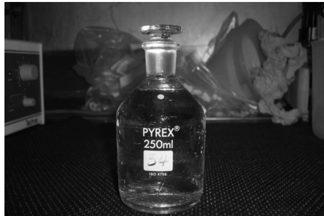
Figure 24 - 250 ml glass stoppered bottle showing the Presens O 2 sensitive spot glued to the bottle-neck
