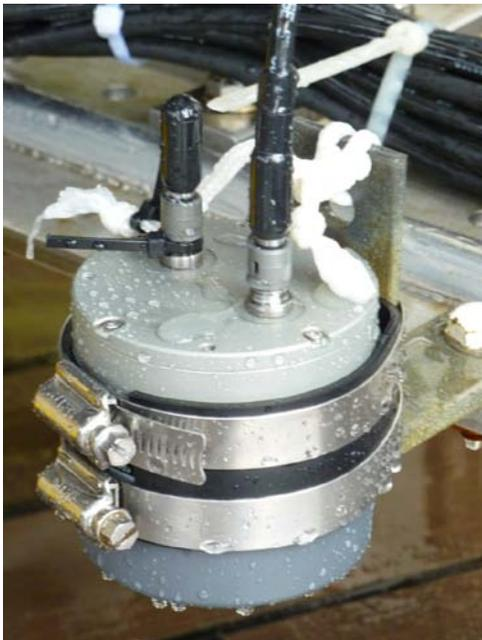
Figure 1 - ES853 echo sounder with serial cable connection.
