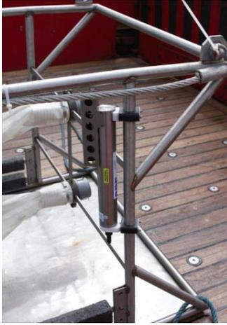
Figure 13 - CTD mounted on EBS frame on the port back
