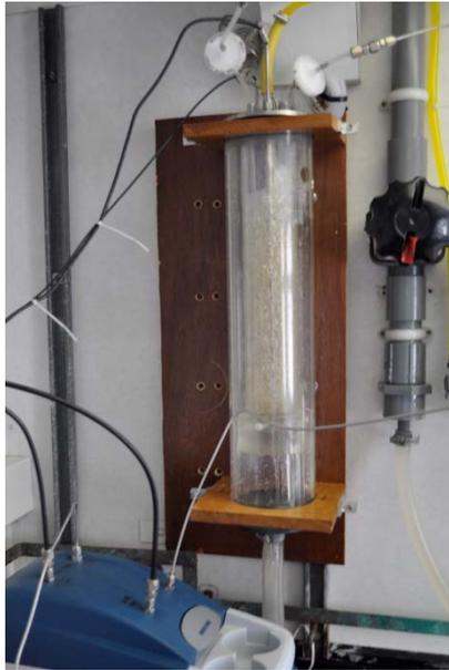
Figure 30 - Percolating packed bed equilibrator, connected to ship's pumped seawater supply in chemistry lab.
