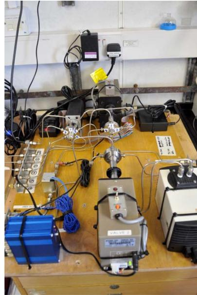
Figure 29 - Valve board, connecting the N<sub>2</sub>O/CO analyser to the equilibrator headspace, marine air line and reference gases.
