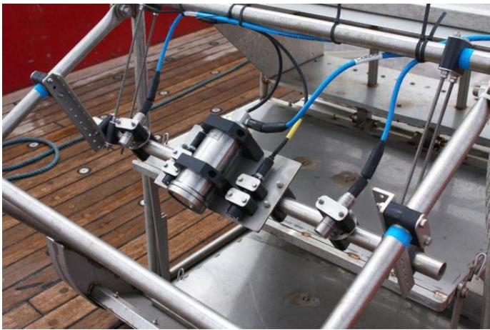
Figure 14 - Front of EBS with Camera (centre) Lasers (each side of camera) and Lights (on the outsides)
