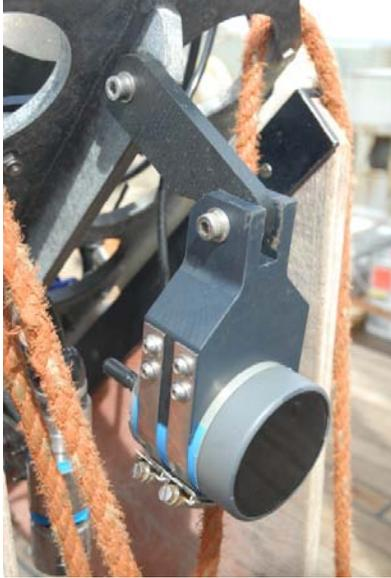
Figure 4 - The echo sounder is shown in a revised position, occupying the space previously held by the flow meter.
