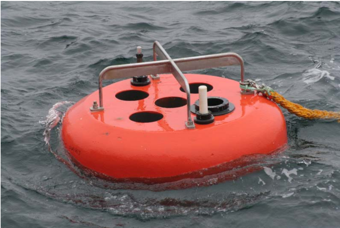
P2 mooring at the surface with no ADCP in bracket
