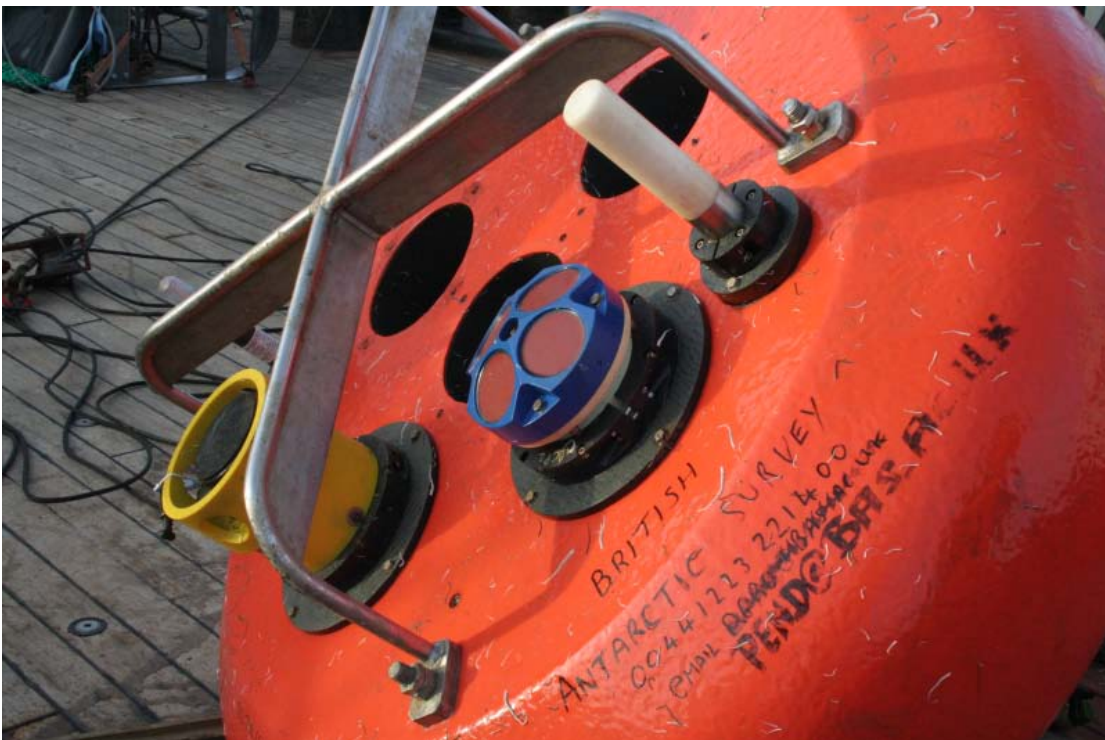
WCB mooring after recovery with ADCP and WCP in their places
