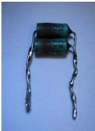
Figure 11. Burnt TIR2 ND6011 shunt resistor(s).
