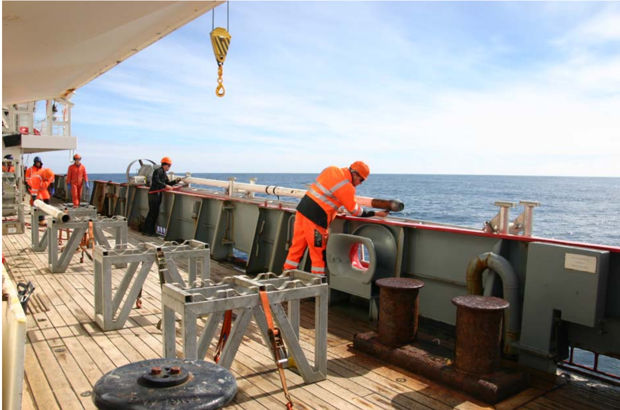
Figure 6. Preparation of the BAS gravity corer for a 9 m-deployment on cruise JR284. (Photo: Christine Batchelor).
