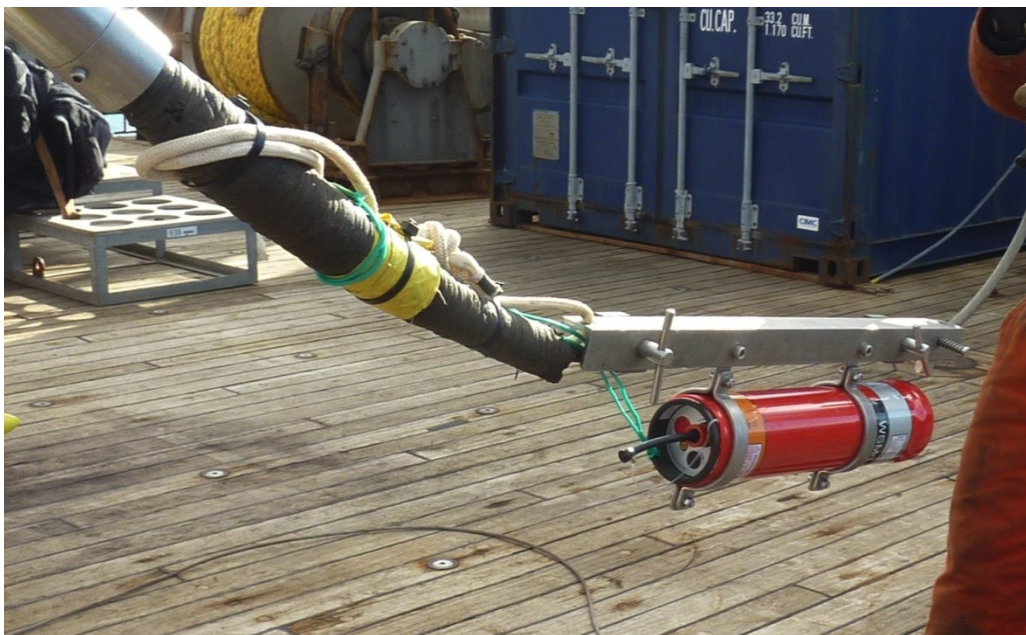
Figure 8: USBL attached to biowire cable, directly above termination
