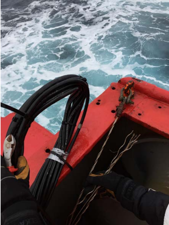
Figure 37. Damaged towing strop.
