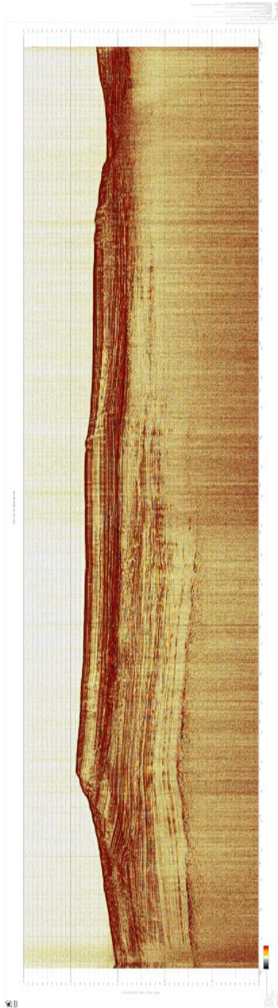
Figure 11. BAS145-57 Brute stack. The left portion of the line is constrained by detailed velocity picks while the right hand half (from approximately centre) is constrained by a basic linear velocity model.
