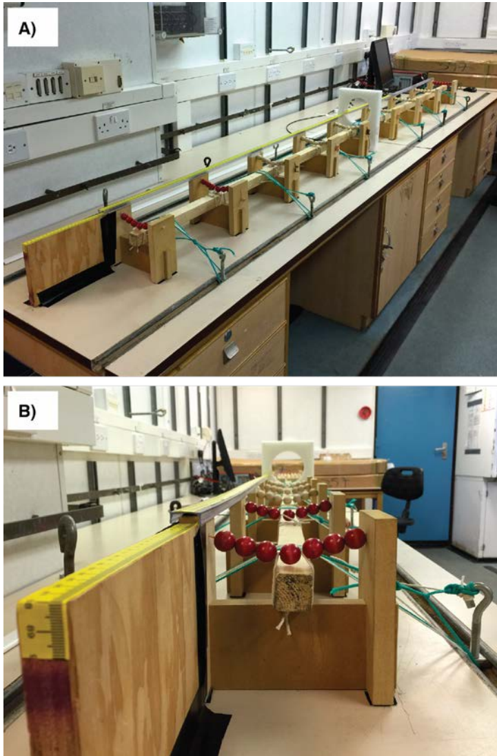
Figure 32. Magnetic susceptibility track built during JR298. A) General view; and B) view along measurement track.
