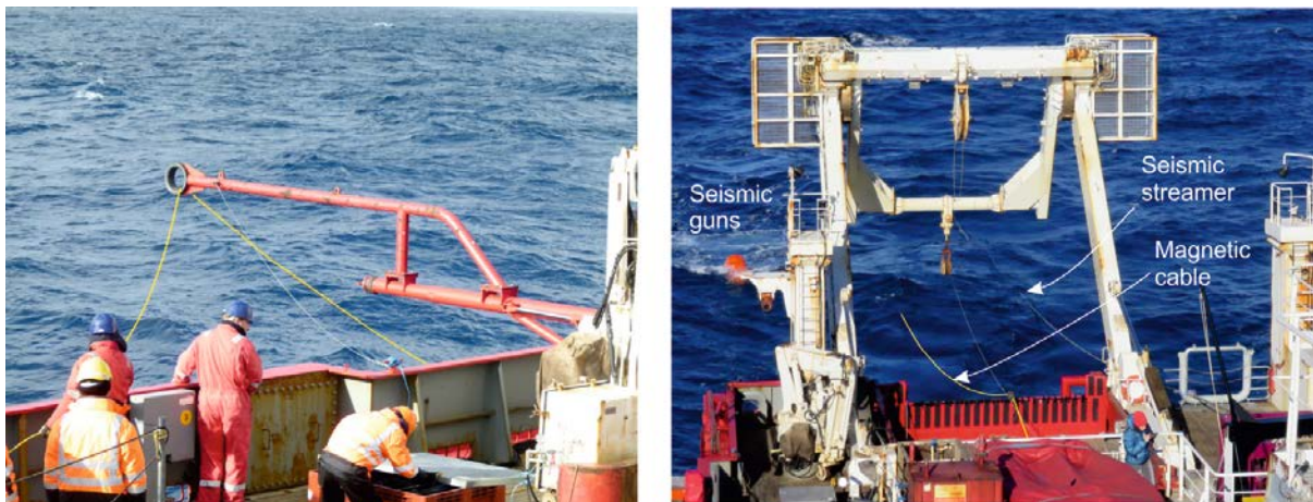
Figure 43. a) Starboard side fairlead magnetometer deployment (yellow cable) when collecting seismic data in ice-free conditions. b) Magnetometer deployment through A-frame when also collecting seismic data in icy conditions.
