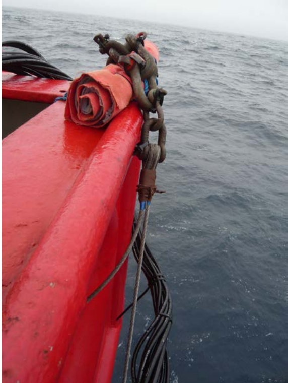
Figure 38. Repaired strop and modified towing arrangement.
