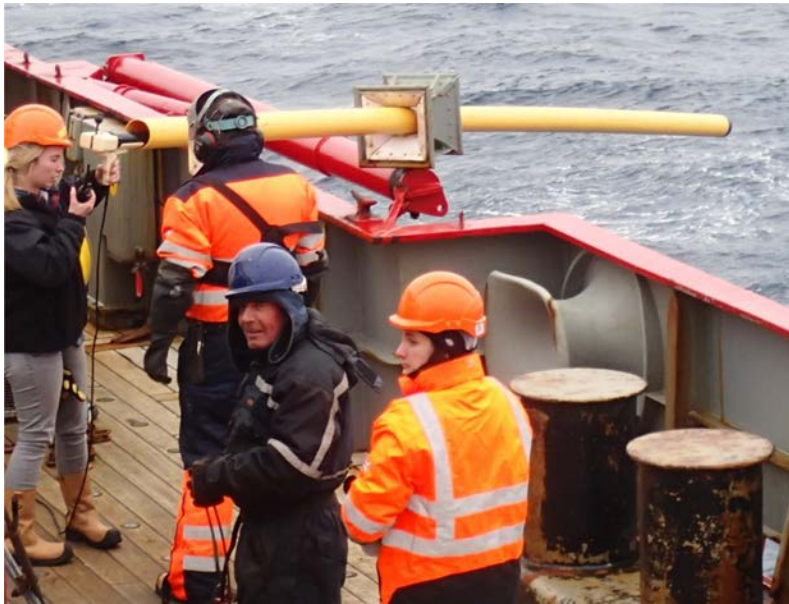
Figure 44. XBT deployment through gravity core liner pushed through port quarter boom fairlead.
